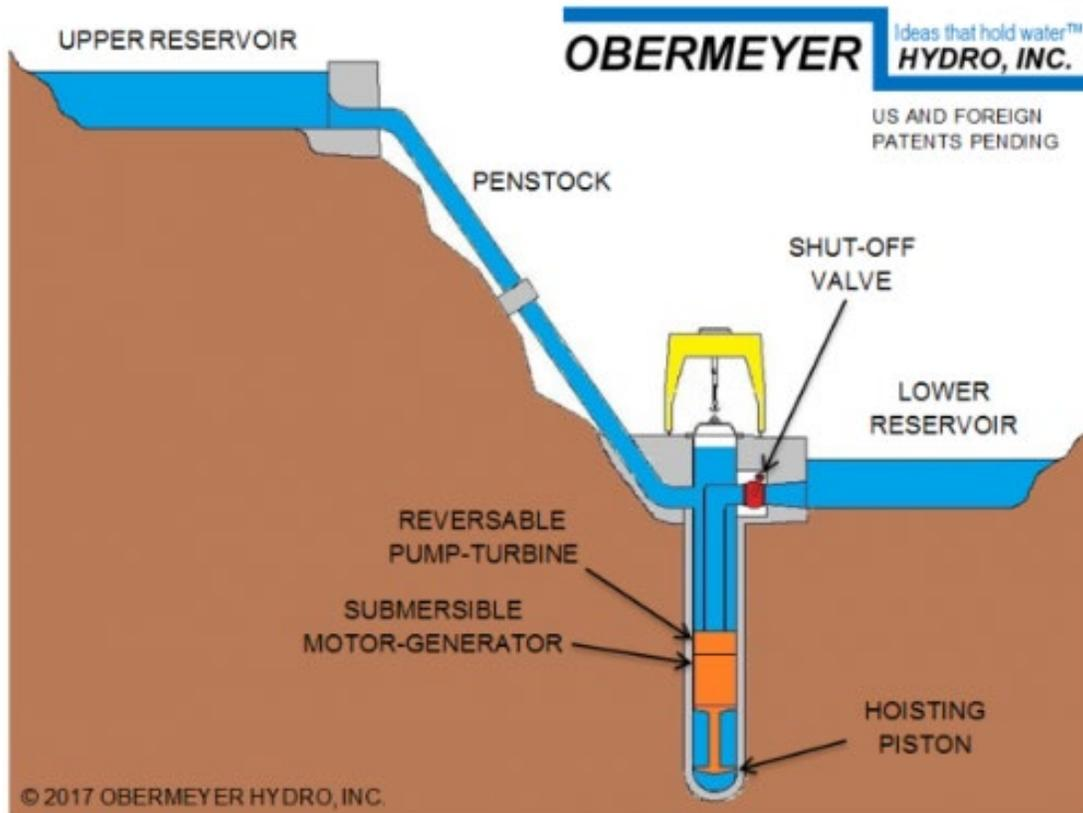
**Figure 3-3 Cross-Section of PSH Plant Using Submerged Pump Turbine and Motor Generator (Source: Obermeyer Hydro)**
