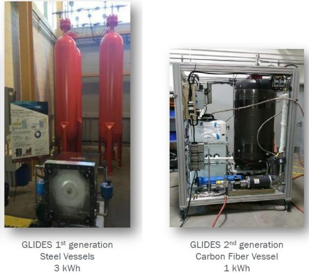
**Figure 3-17 GLIDES Proof-of-Concept Prototypes (Source: Abu-Heiba, 2019)**
