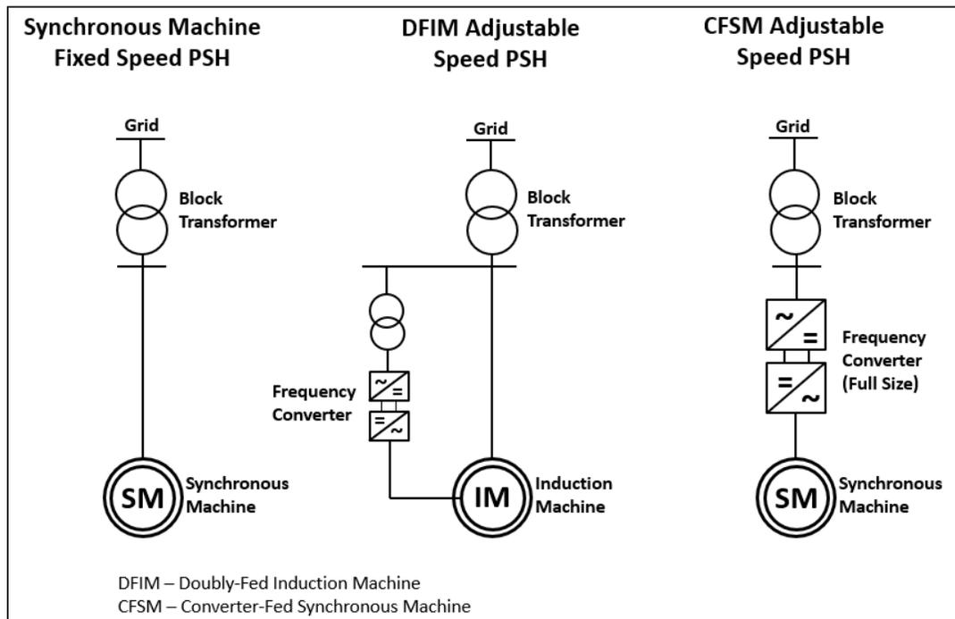
**Figure 2-4 Single-line Diagrams of Fixed- and Adjustable-Speed PSH Technologies (Source: Koritarov et al., 2015)**
