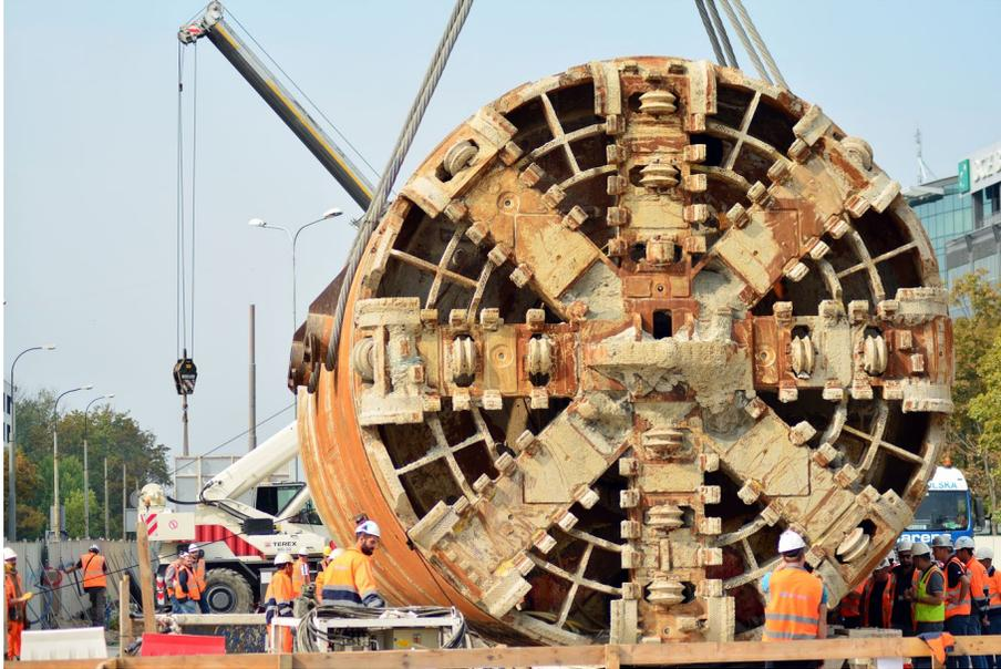
**Figure 5-1 TBM Cutter Head (Photo credit: Shutterstock)**
