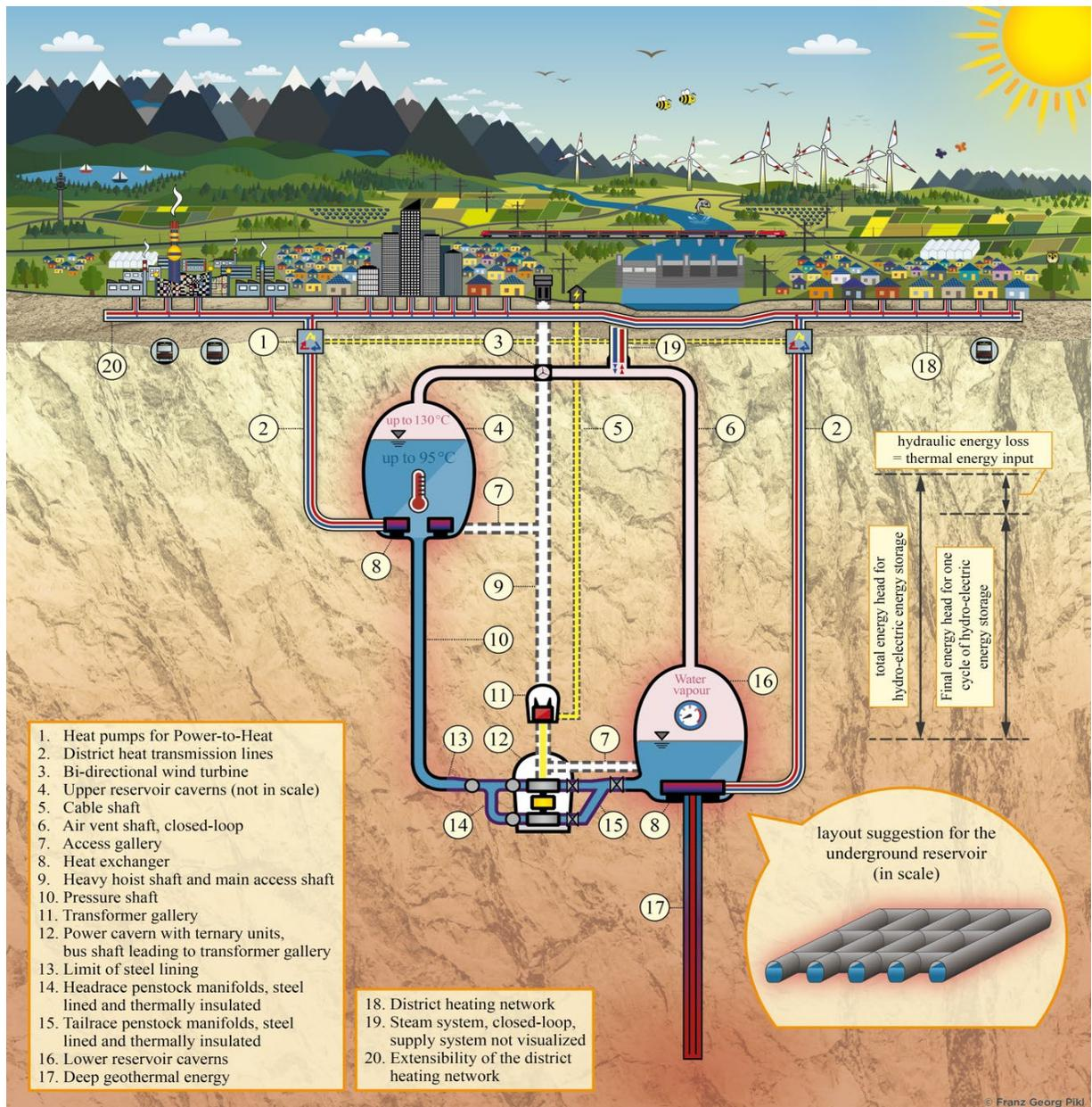
**Figure 3-18 Schematic of Thermal Underground PSH System (Source: Franz Georg Pökl, Graz University of Technology)**
