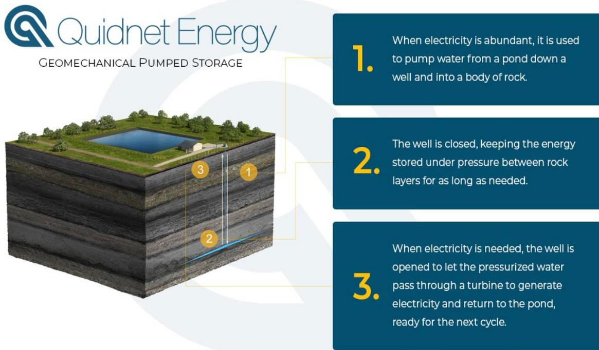
**Figure 3-5 Geomechanical PSH Technology (Source: Quidnet)**
