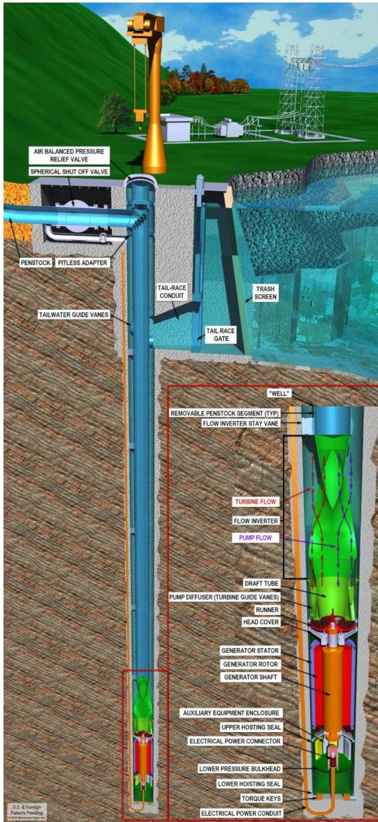
**Figure 3-4 Cross-Section of a Well with Submerged Pump Turbine and Motor Generator (Source: Obermeyer Hydro)**
