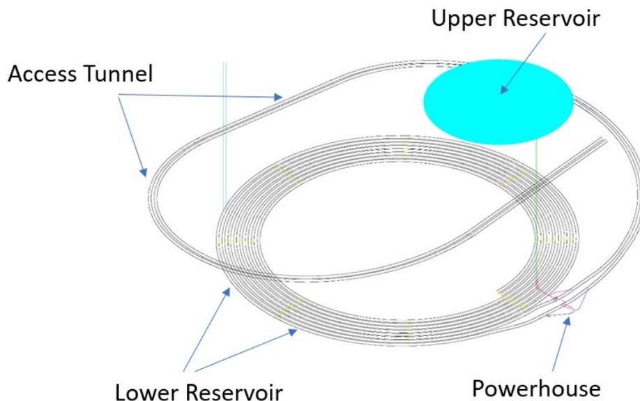
**Figure 3-11 Design Concept of Underground PSH (Source: Nelson Energy)**
