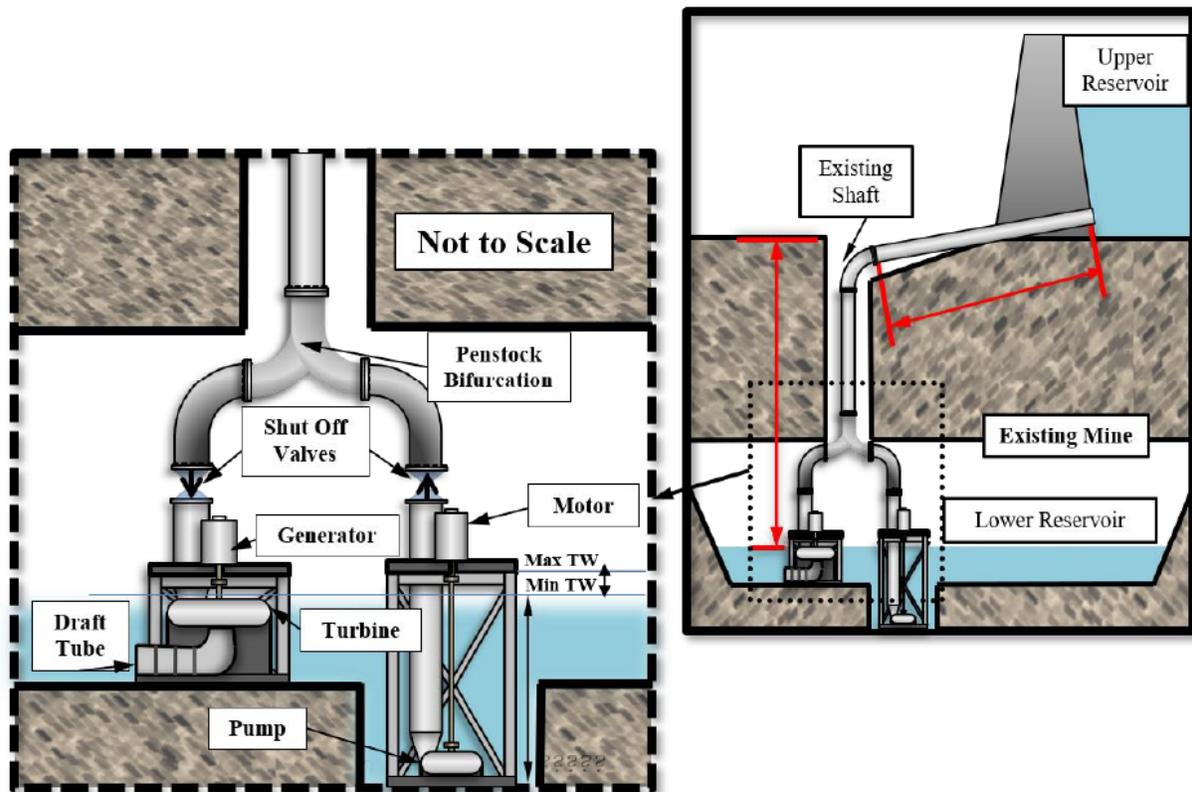
**Figure 3-12 Conceptual Configuration of a Closed-loop PSH Plant in an Underground Coal Mine (Source: Hadjerioua et al., 2020)**
