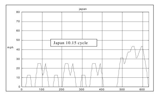
Figure 4-1b Speed Profile of the Japan 10/15 Cycle
