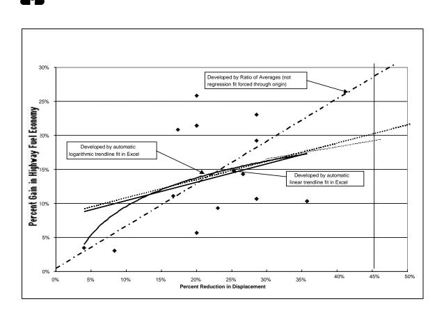
Figure 1 HWY Cycle Percentage Gain in Fuel Economy as Function of Engine Displacement Reduction
