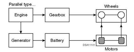
Figure 2-2 One Example of a Parallel Hybrid Drivetrain
