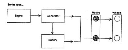
Figure 2-3 One Configuration of a Series Hybrid Drivetrain
