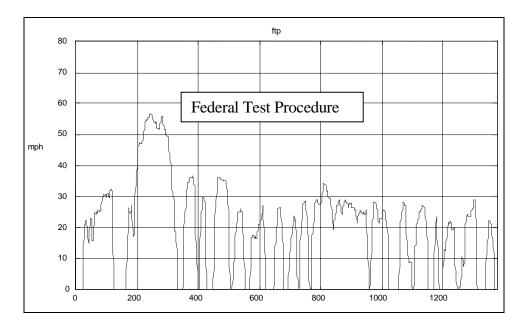
Figure 4-1c Speed Profile of the Federal Test Procedure (FTP)
