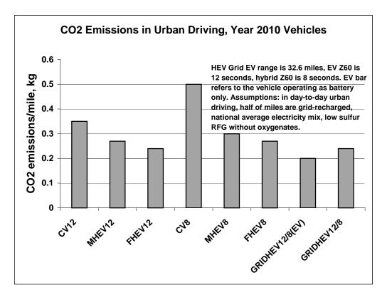
Figure 4-13 CO<sub>2</sub> Emissions from Similar Conventional and Hybrid Vehicles in Urban Driving (FTP driving cycle, kilograms per mile)
