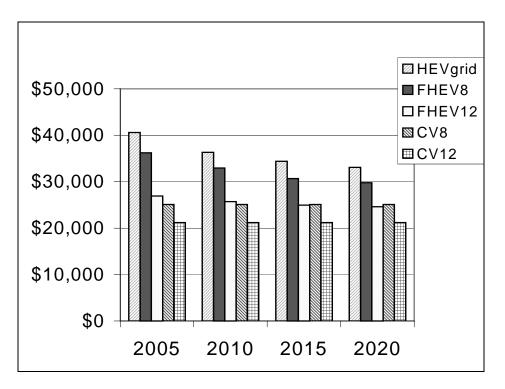
Figure 4-10 Vehicle Cost Comparison: Grid-Connected and Grid-Independent Parallel HEVs vs. CV
