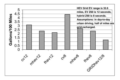
Figure 4-12 Comparison of Gasoline Use: CV vs. Grid-Independent and Grid-Connected (32.6-mile range) HEVs in Urban Driving
