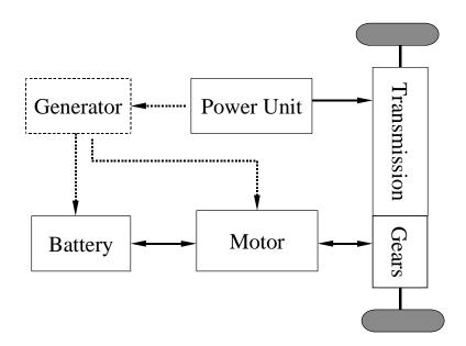
Figure 4 Parallel HEV Drivetrain Components and Their Connections
