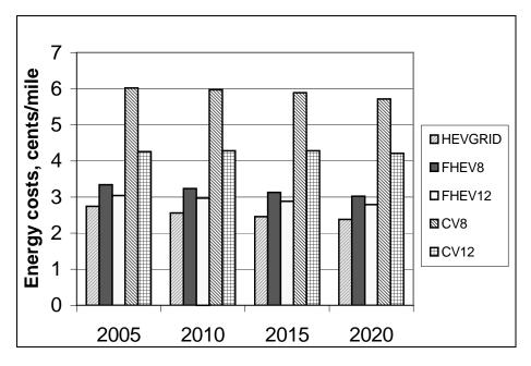
Figure 4-9 Fuel + Electricity Cost: CVs vs. Parallel Grid-Connected (EV Z60 = 12 seconds) and Grid-Independent HEVs
