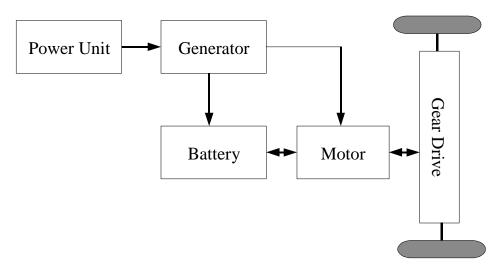
Figure 3 Series HEV Drivetrain Components and Their Connections
