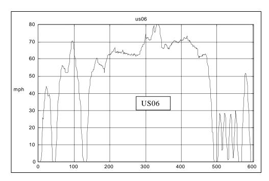
Figure 4-1d Speed Profile of the U.S. No. 6 Cycle
