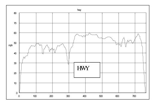
Figure 4-1e Speed Profile of the Highway Cycle
