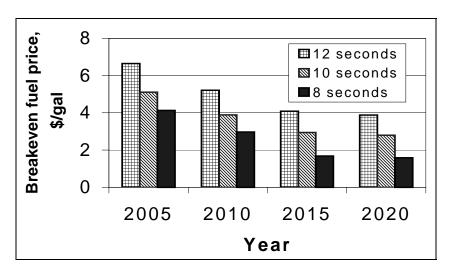
Figure 4-8 Breakeven Fuel Prices for CVs and Parallel Grid-Independent Mild Hybrids, for Three Performance Levels
