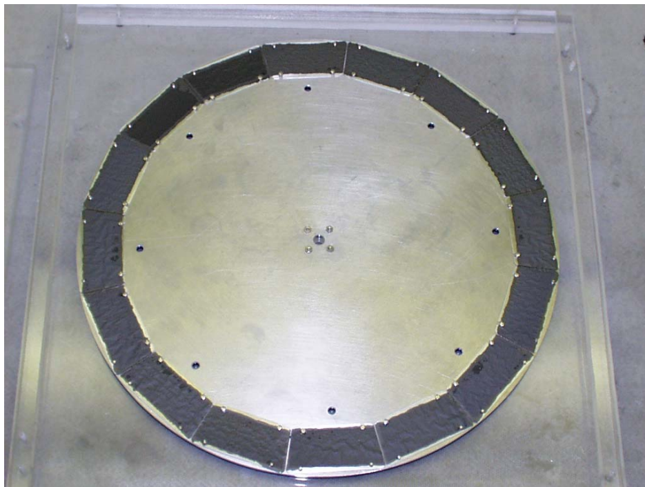
Fig. I-76. Picture of the large rotating target wheel installed at the Enge spectrograph. The beam hits the targets at 6 inch radius with the target rotating at about 1000 rpm.
