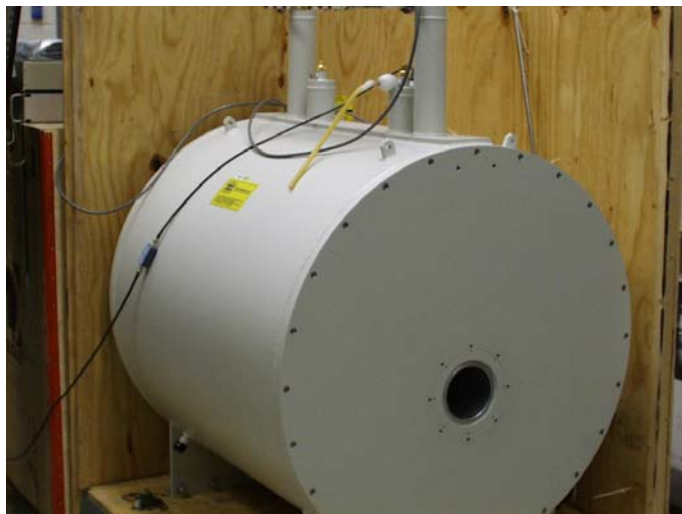
Fig. I-79. Picture of the 5 inch warm bore, 7 Tesla, superconducting solenoid that will be used to host the Penning trap of the APT.
