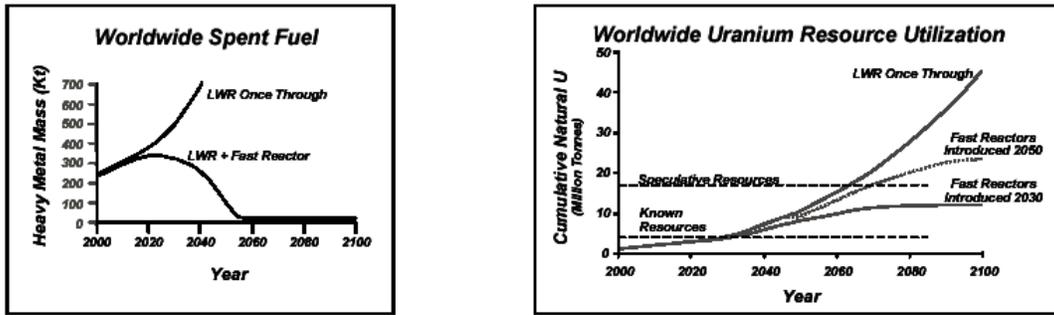
Figure 1. The effect of closed fuel cycles on waste burden and resource utilization
