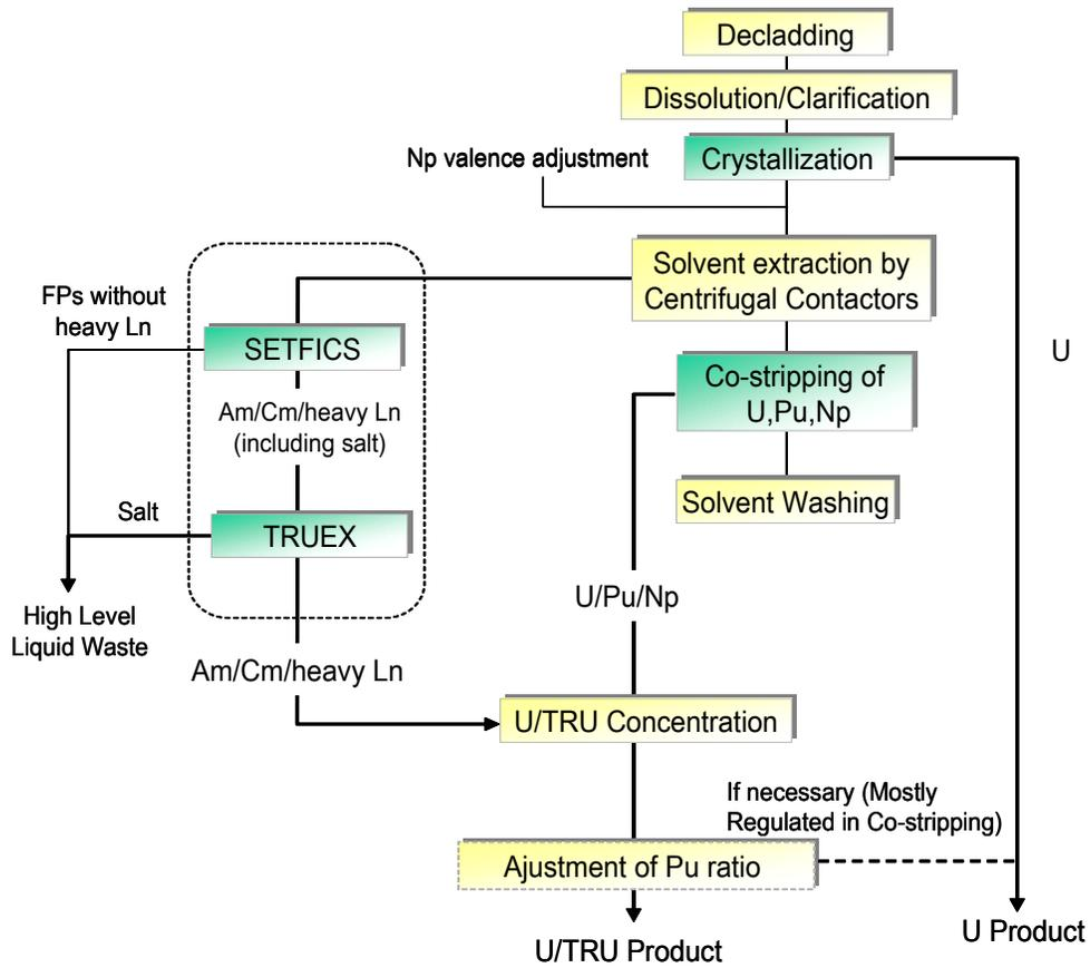
Figure 2. Schematic flow diagram of Advanced Aqueous Reprocessing
