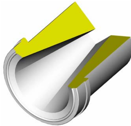
Figure III-18. A section view of the tapered nozzle to be used in the prototype liquid-lithium target. It is rectangular, 10 mm by 5 mm, on the output and circular, 22 mm in diameter, on the input.
