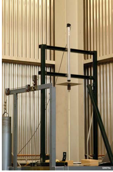
Fig. 4. Experiment Setup of Linear Potentiometer
