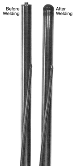
FIGURE 3-40. AN ASSEMBLED FUEL ELEMENT BEFORE AND AFTER WELDING.
