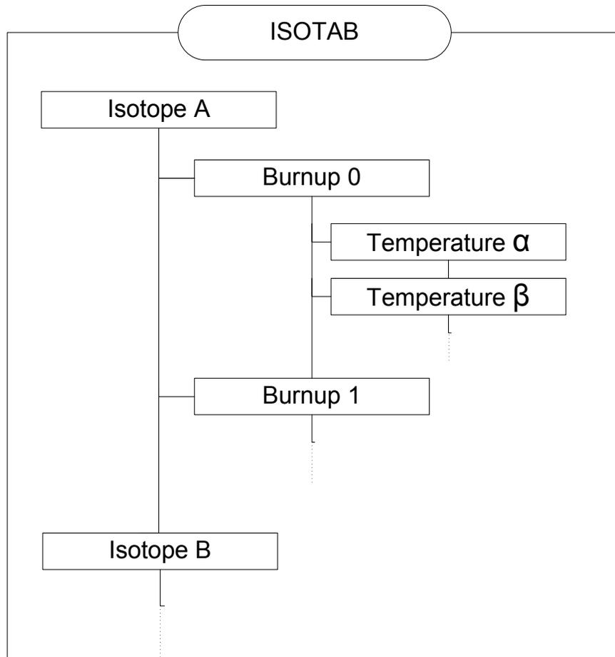
**Figure 5. Structure of ISOTAB File.**
