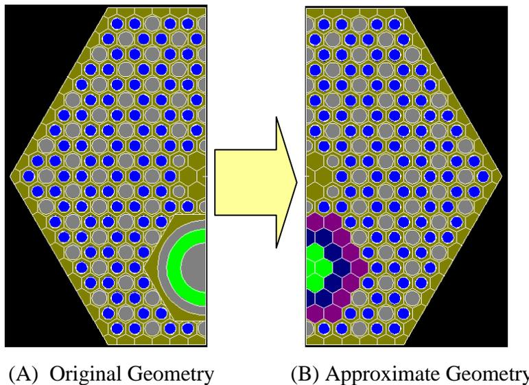
**Figure 23. Geometry Approximation of Rodded Fuel Block Model.**
