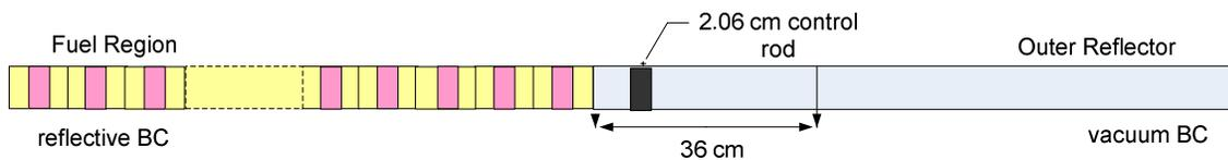
**Figure 16. One-Dimensional Slab Geometry Model for Control Rod.**
