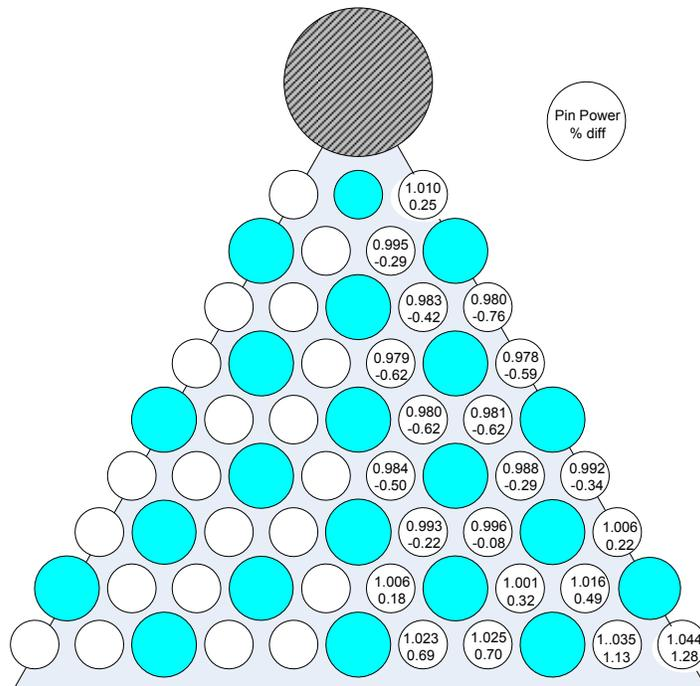
**Figure 26. Pin Power Distribution Determined from DRAGON Calculation.**
