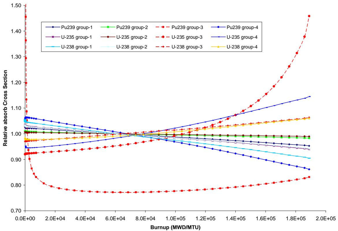
**Figure 7. Burnup Dependence of Absorption Cross Sections.**
