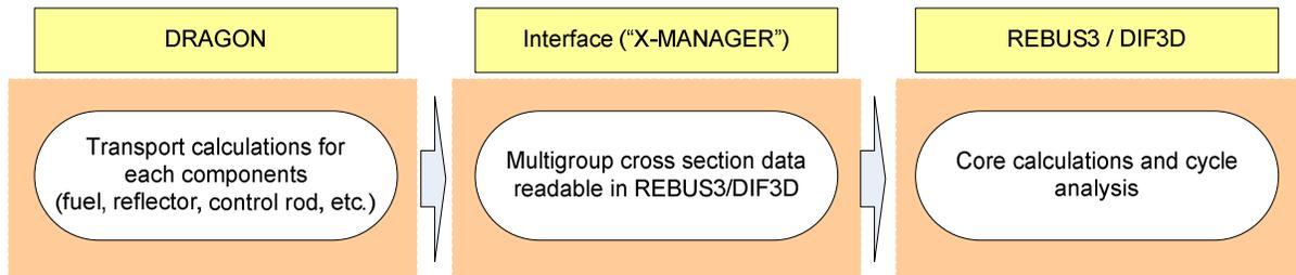
**Figure 1. Link between DRAGON and REBUS-3/DIF3D Codes.**
