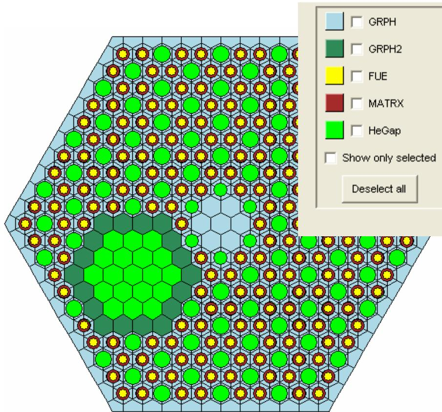
**Figure 30. VHTR Fuel Block with Control Rod Hole.**
