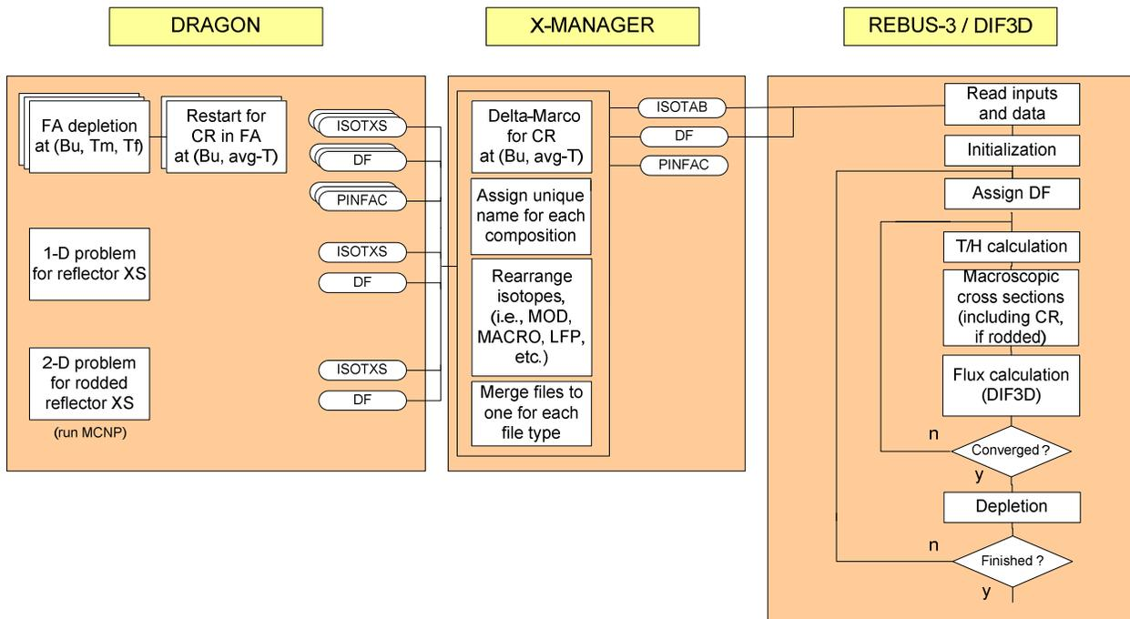
**Figure 27. Data Flow for DRAGON, X-MANAGER, and REBUS-3/DIF3D.**
