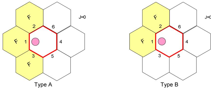
**Figure 18. Two-Dimensional Modeling for the Rodded Reflector Region.**
