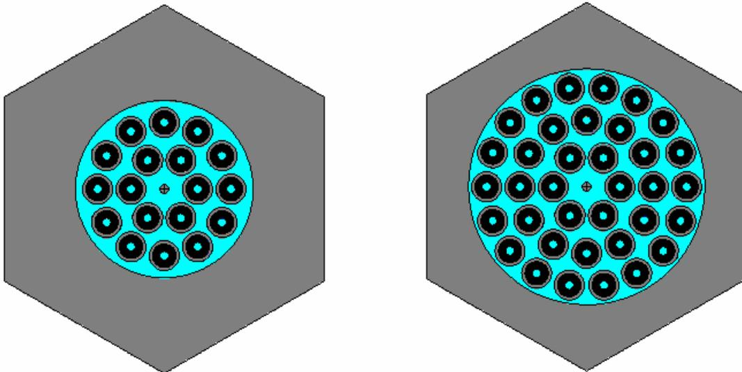
**Figure 2. Radial Layouts of New 18-Pin (Left) and 36-Pin (Right) Stringer Assemblies.**
