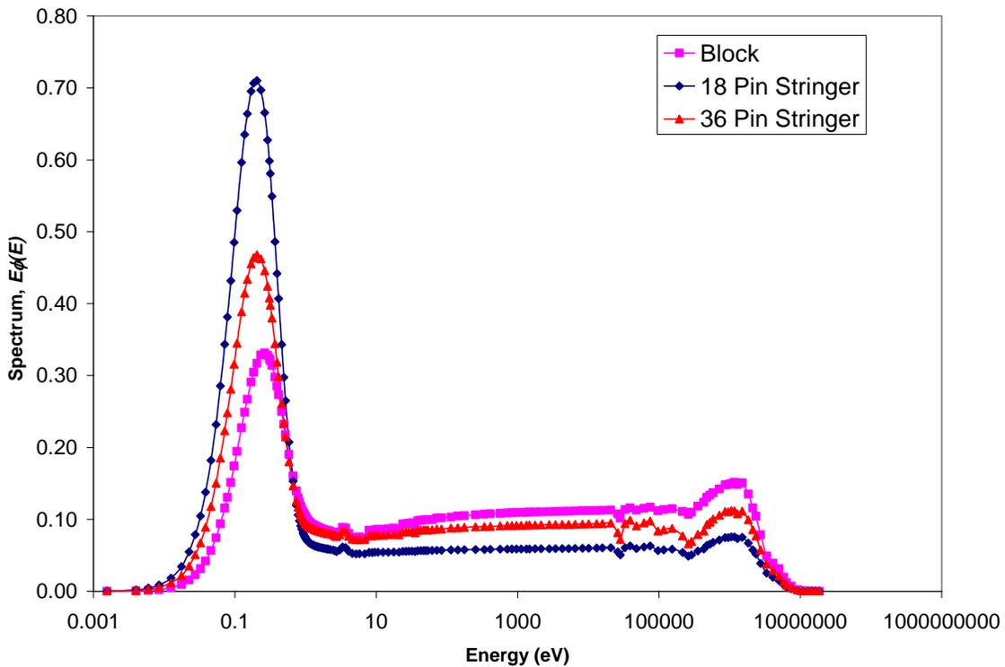
**Figure 10. Variation of Neutron Spectrum with Assembly Design.**
