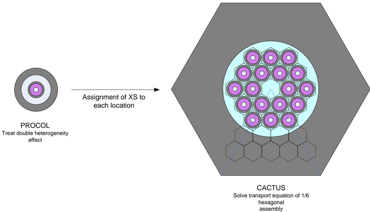
**Figure 3. Schematic of CACTUS Geometry Model.**
