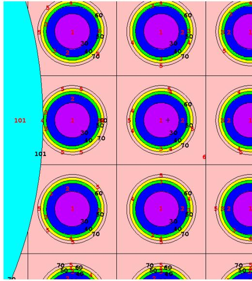
**Figure 5. Representation of TRISO Particles in Fuel.**
