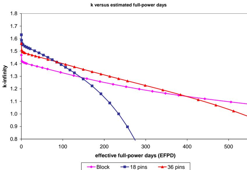
**Figure 7. Comparison of k-infinity Versus Cycle Length for 25% Enrichment.**
