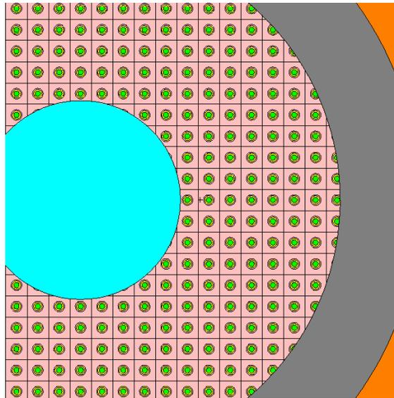
**Figure 4. Enlarged View of Annular Fuel Compact.**
