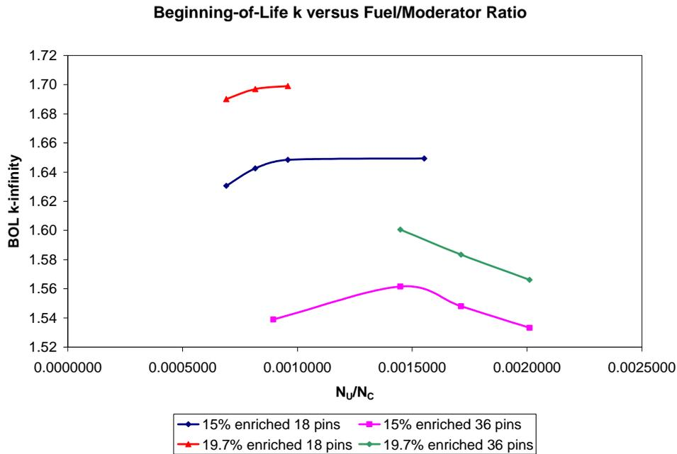
Figure 8. Trend of BOL k-infinity Versus Fuel-to-Moderator Ratio.
