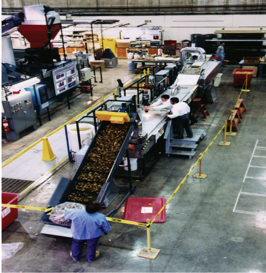
FIGURE 8.2 Wash, Rinse, and Dry Continuous Equipment
