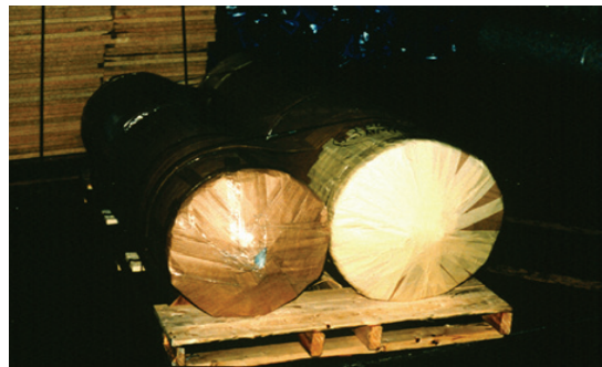
FIGURE 8.5 Recovered Foam from Shredder Residue Made into Carpet Padding
