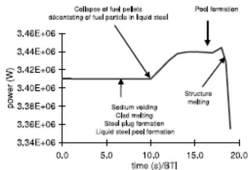
Figure 39 Power Generated in the Blocked Assembly during the Postulated TIB Accident
