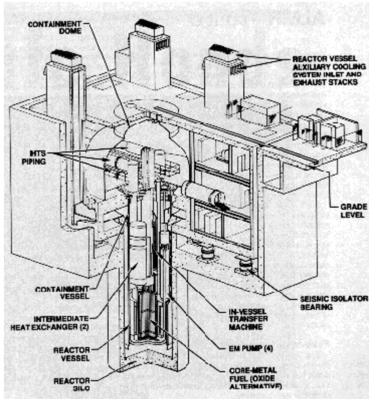
Figure 25 PRISM Reactor Module [4-18]
