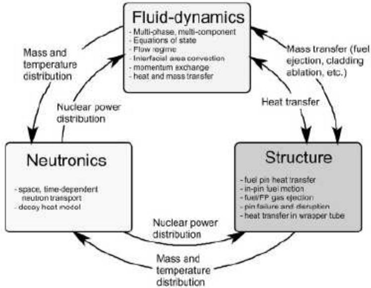
Figure 31 Overall Framework of the SIMMER-III Code
