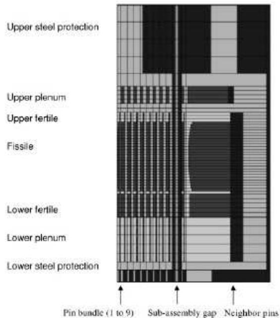
Figure 38 SIMMER-III Geometry of the Assemblies Considered in TIB Analysis
