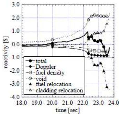
Figure 34 Reactivity Components during the IP Nominal LOF Case
