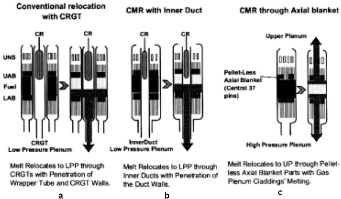
Figure 11 Post-Accident Material Relocation with CMR
