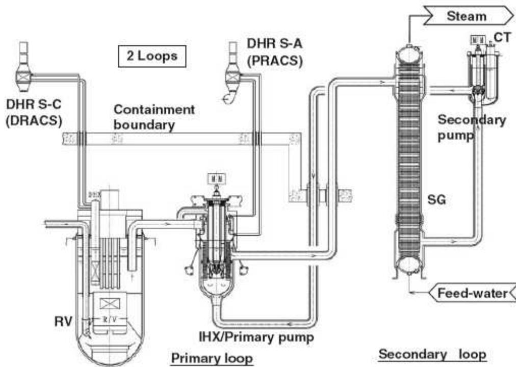
Figure 16 Schematic View of the Modified JSFR Heat Transport System [4-1]
