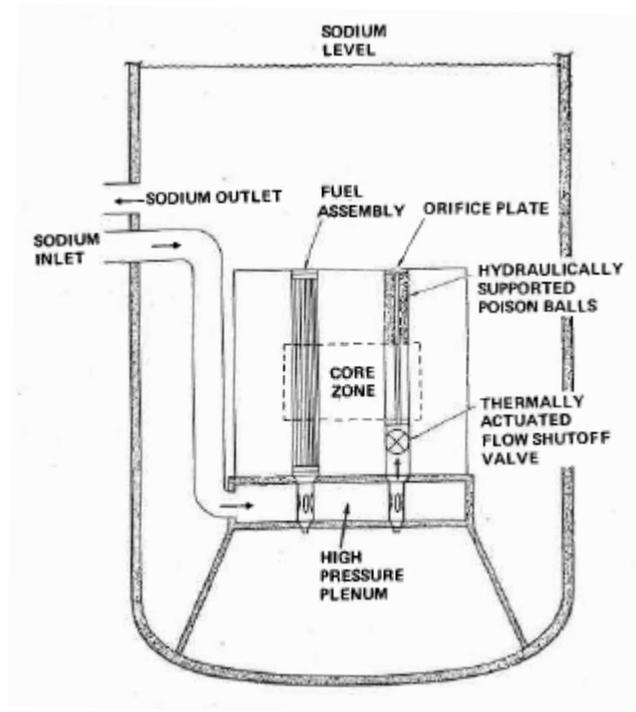
Figure 3 Hydraulically Supported Absorber Ball Assembly in a SFR
