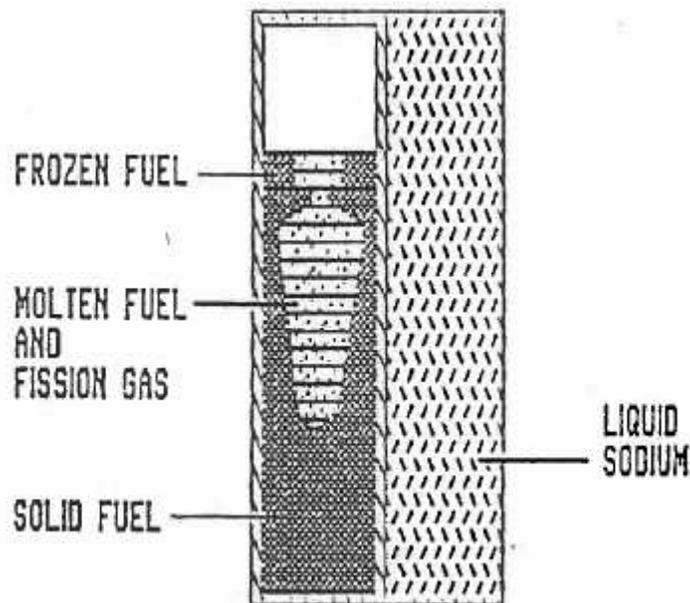
Figure 30 PINACLE Configuration
