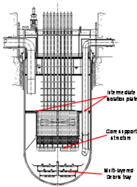
Figure 12 Schematic View of JSFR with Multi-Layered Debris Tray
