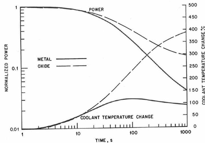
Figure 40 Reactor Power and Peak Coolant Temperature Change Histories for the Unprotected LOF Accident
