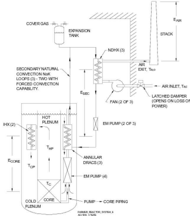
Figure 6 ABTR Pool-Type Heat Transport System Configuration [3-27]
