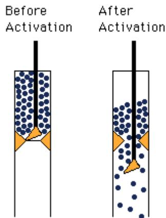
Figure 28 Ultimate Shutdown System Assembly
