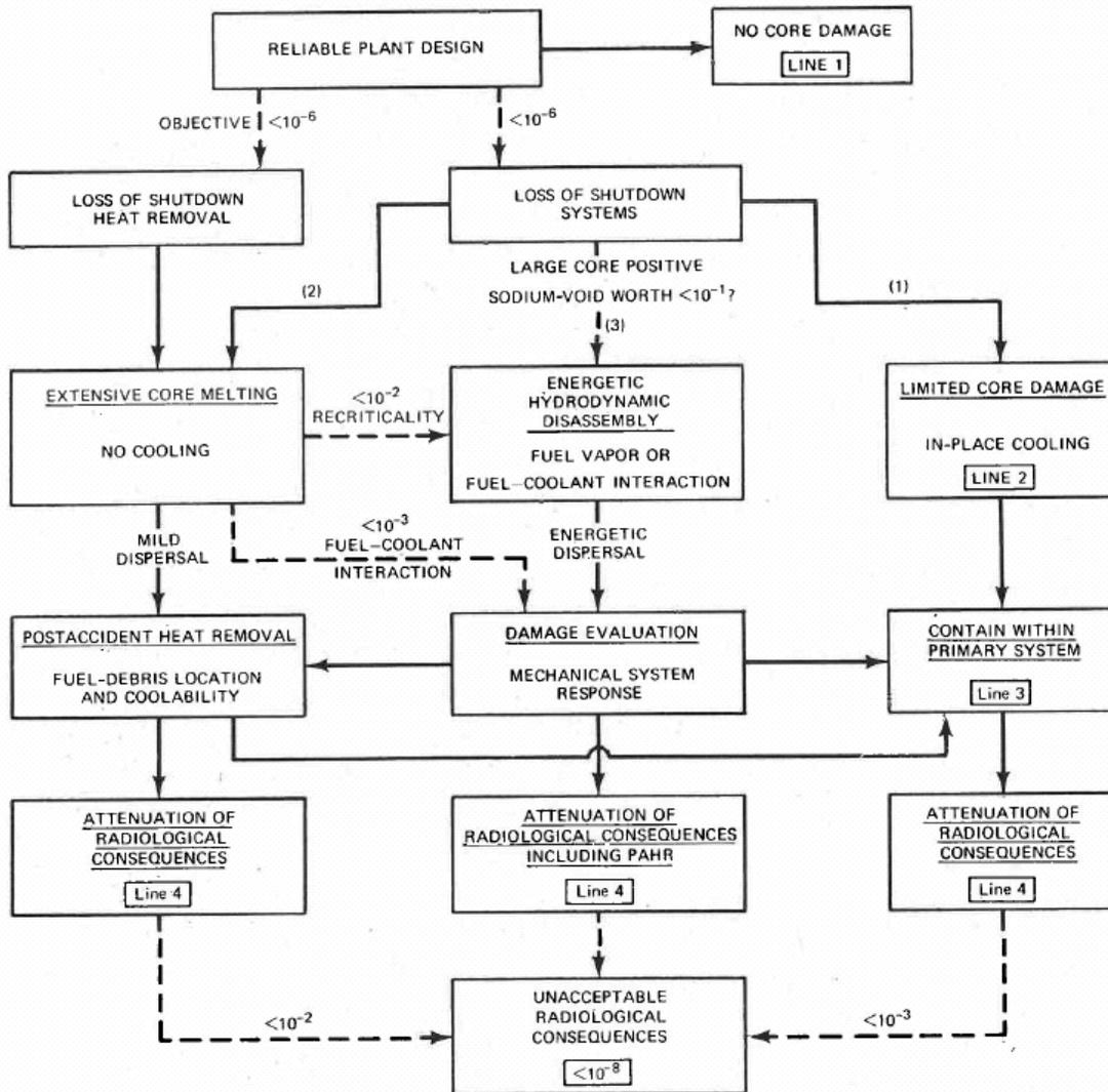
Figure 1 Simplified Path Structure of CDA Initiators and the Lines of Assurance [2-1]
