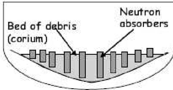
Figure 13 Core Catcher with Neutron Absorbers
