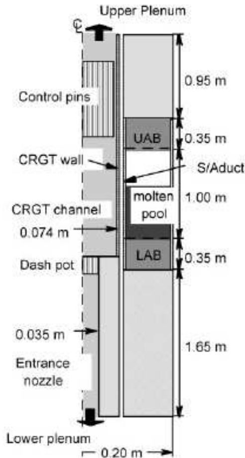
Figure 36 Geometry of Simmer-III Analysis of CRGT Fuel Removal
