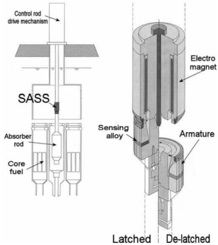
Figure 18 Self-Actuated Shutdown System [4-2]
