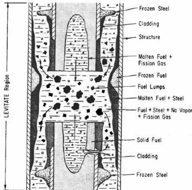
Figure 29 Typical LEVITATE Configuration
