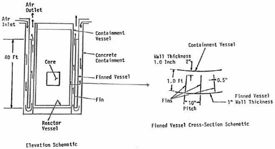
Figure 26 Schematic Representation of the RVACS
