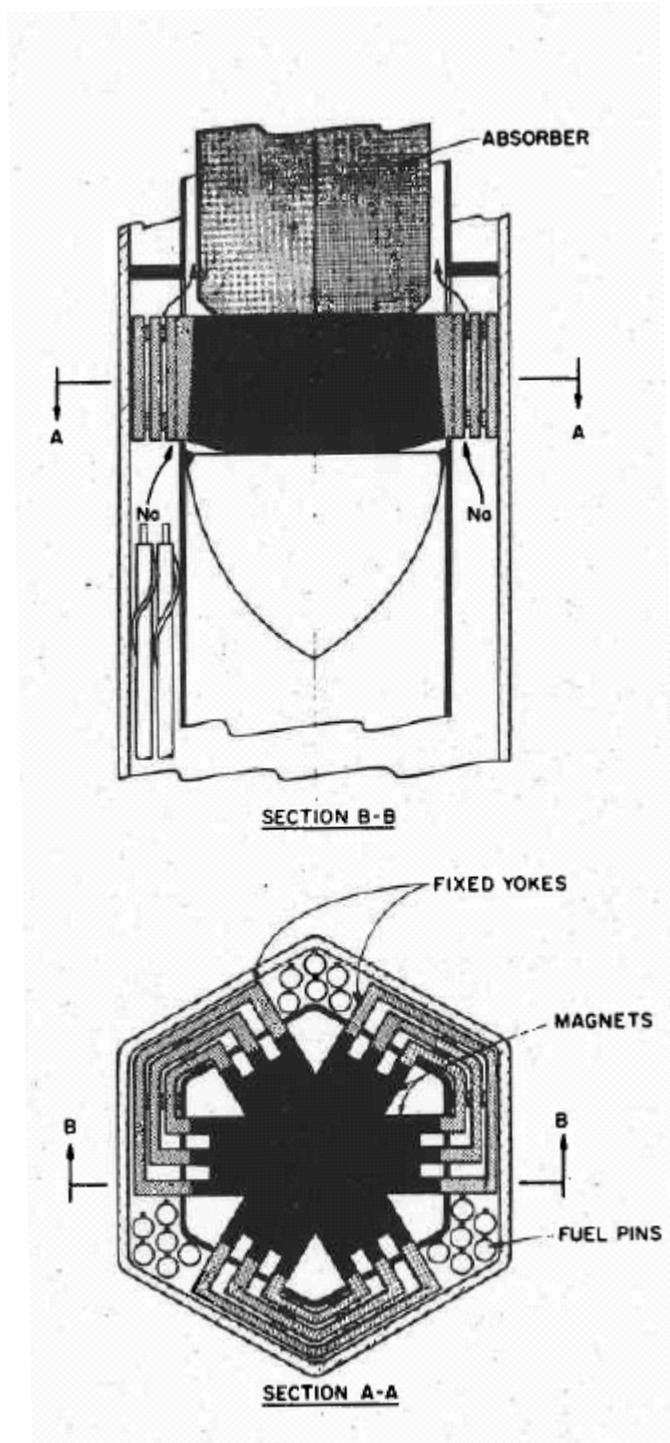
Figure 2 Conceptual Design of a Ferromagnetic Curie-Point-Operated Device
