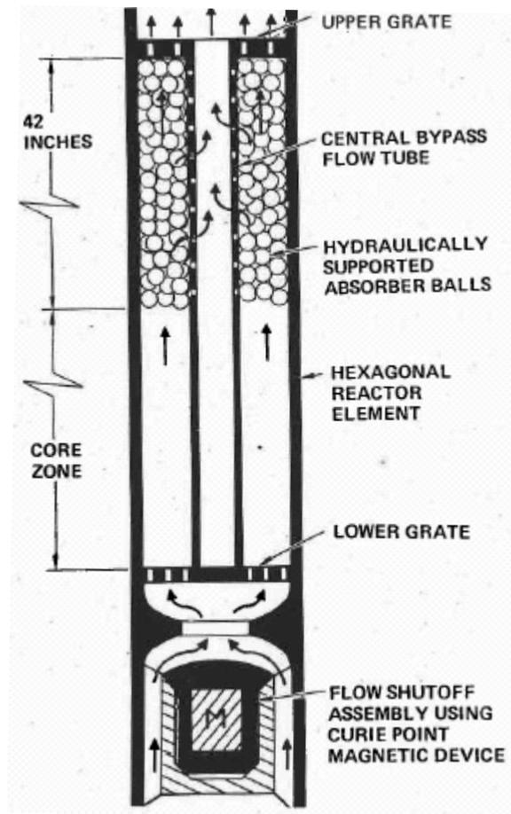
Figure 4 Absorber Ball Assembly Conceptual Design
