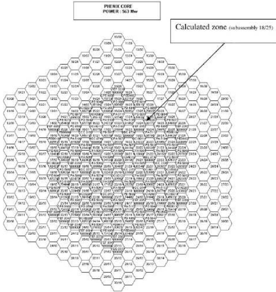
Figure 37 Phoenix Core Configuration and Location of Postulated Blockage
