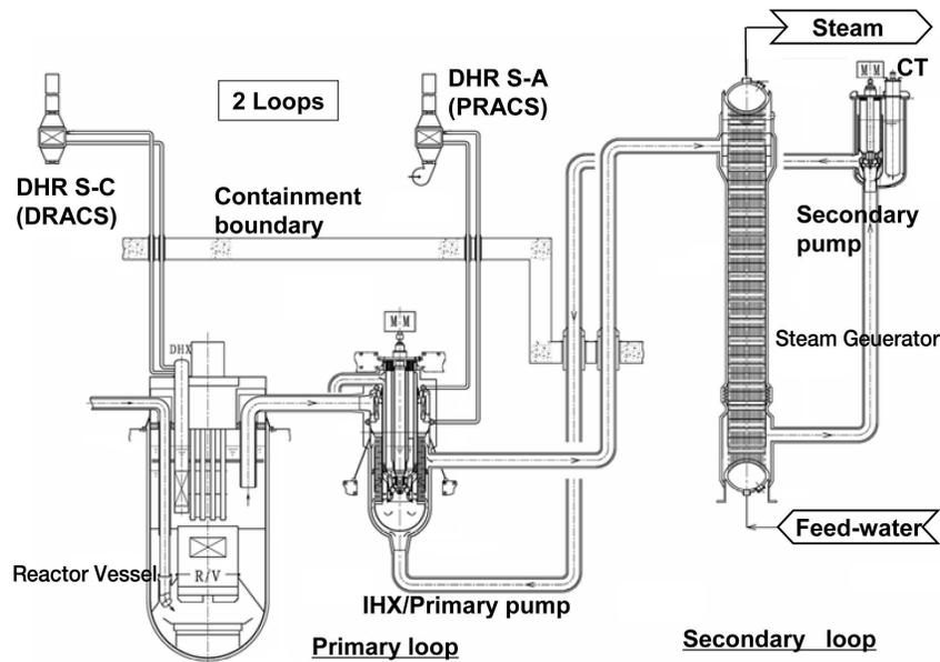
Figure 7 JSFR Loop-Type Heat Transport System Configuration [3-28]
