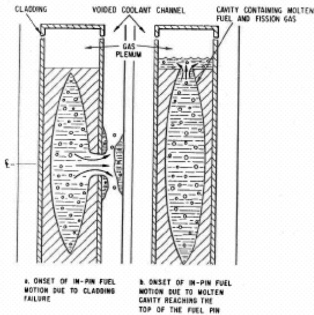
Figure 10 Molten Fuel Relocation Modes
