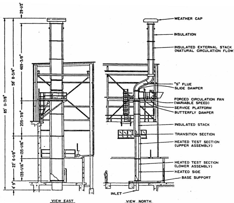
Figure 8 Schematic Overview of the NSTF
