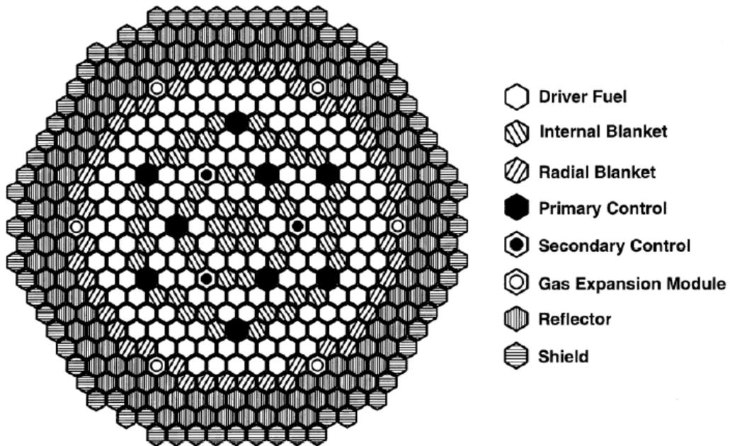
Figure 27 GEM Assembly Locations in the PRISM Core [4-16]
