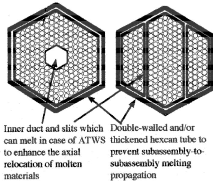
Figure 19 Concept Fuel Assemblies for Enhanced Molten Fuel Escape from the Core [4-4]
