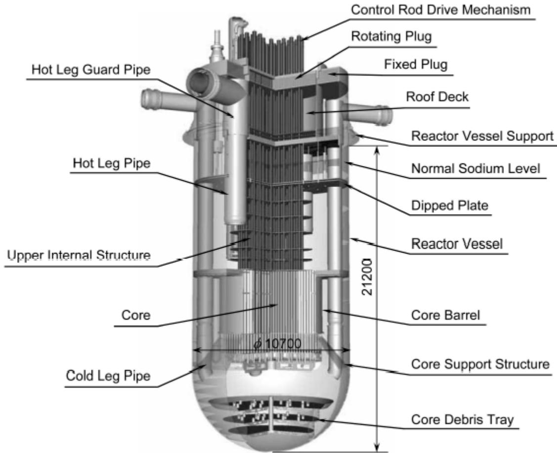
Figure 23 JSFR Reactor Vessel and Internal Structures [4-2]
