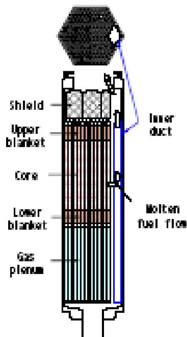
Figure 21 Modified-FAIDUS - Fuel Assembly Design [4-3]
