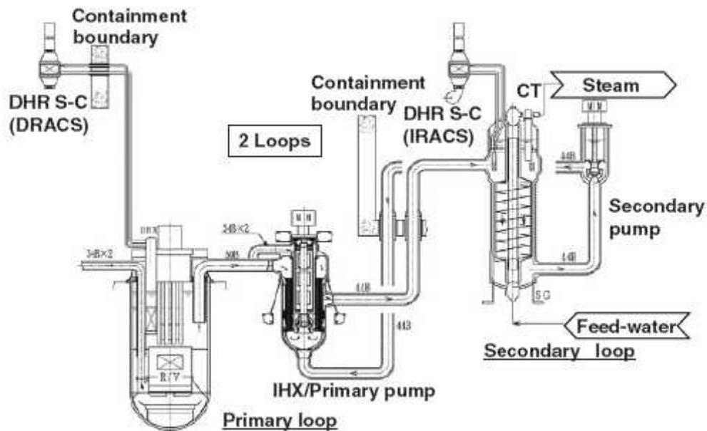
Figure 17 Schematic View of the Original JSFR Heat Transport System [4-1]
