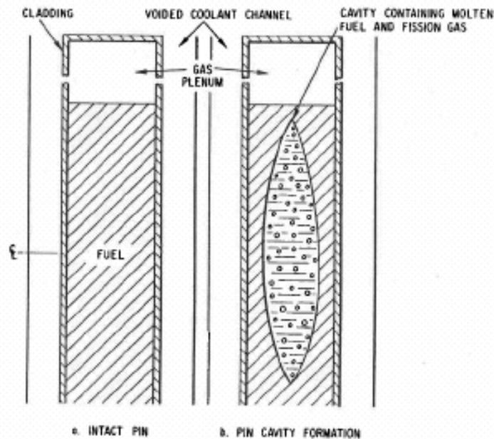
Figure 9 Cavity Formation During the Initial Accident Phase
