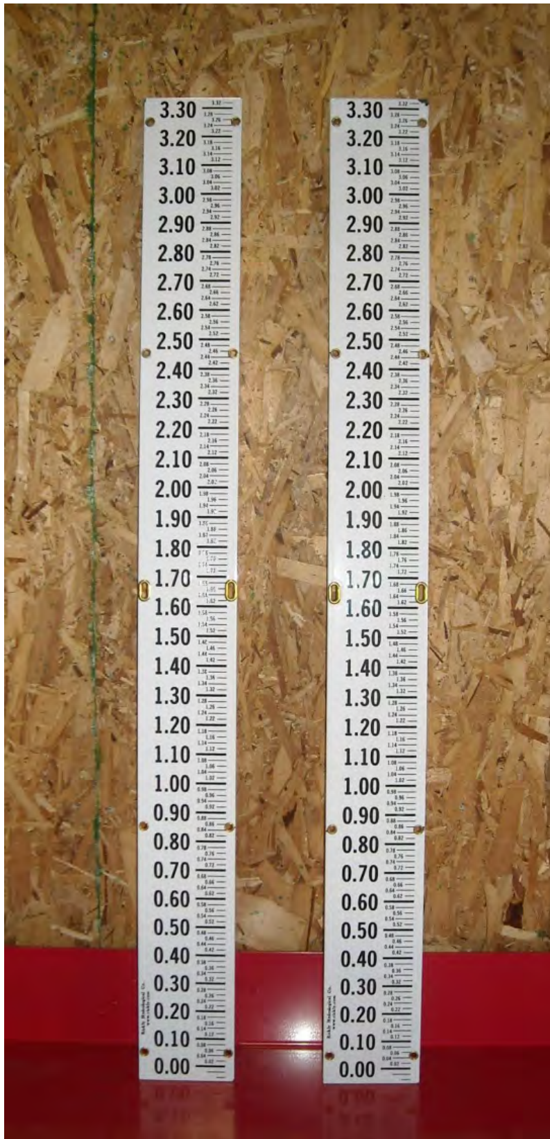
FIGURE 6.3 Graduated water level gauging staffs to be installed in the wetlands subbasins.
