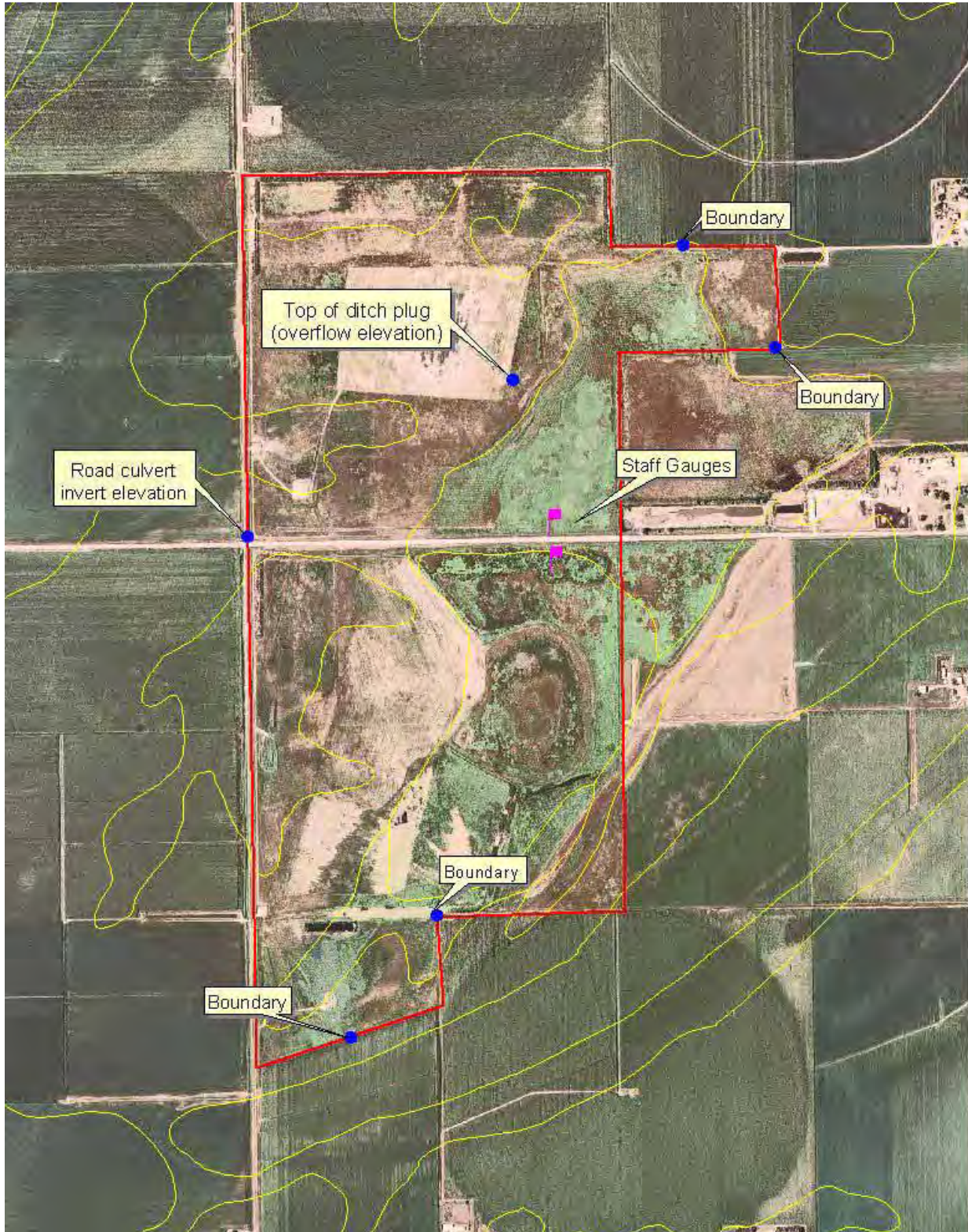
FIGURE 6.1 Locations proposed by the Nebraska Game and Parks Commission for the surveying of topographic elevations and the installation of permanent water level gauging staffs at the North Lake Basin Wildlife Management Area. Surveying was completed and construction of the staff gauges commenced in March 2009.
