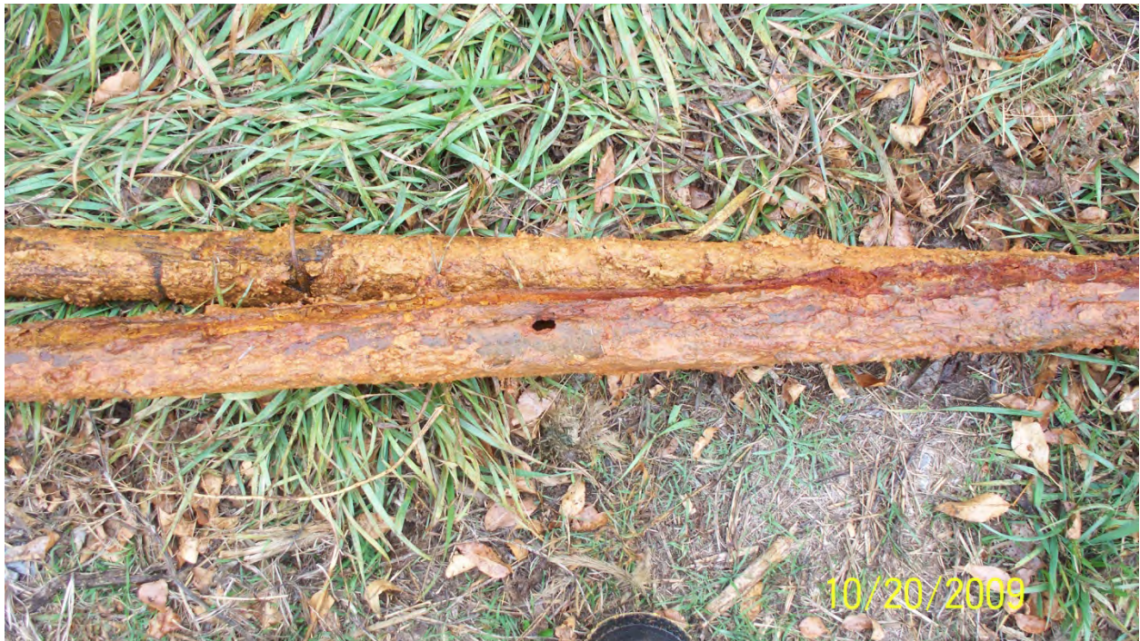
FIGURE 3.1b Corrosion and perforation identified in the steel riser pipe of well GWEX4, October 2009.
