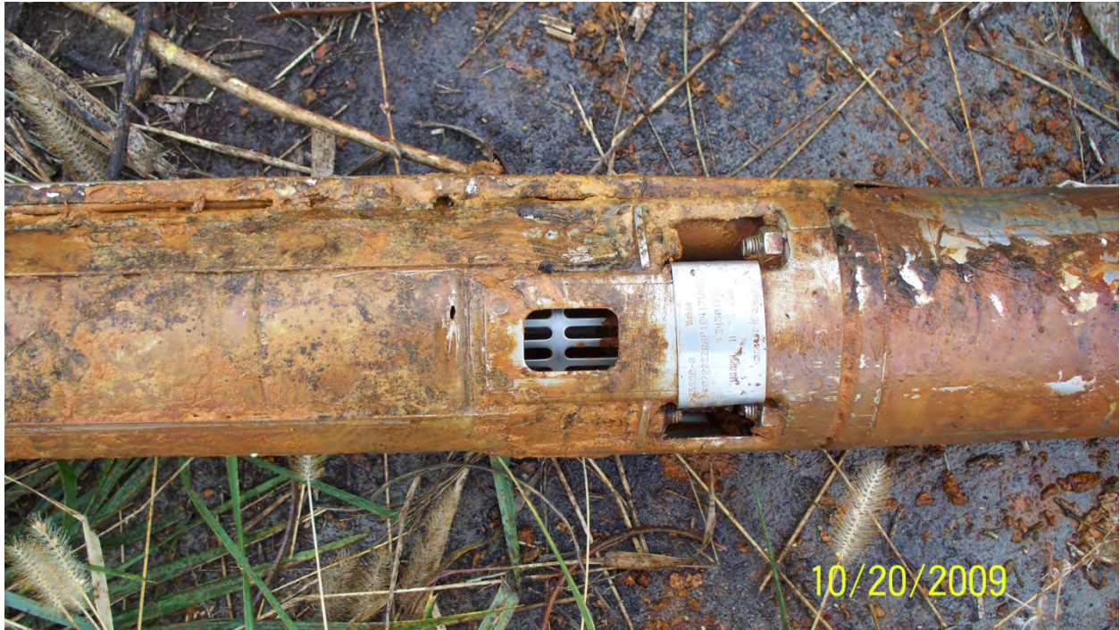
FIGURE 3.1c Corrosion and perforation identified in the downhole pump casing of well GWEX4, October 2009.
