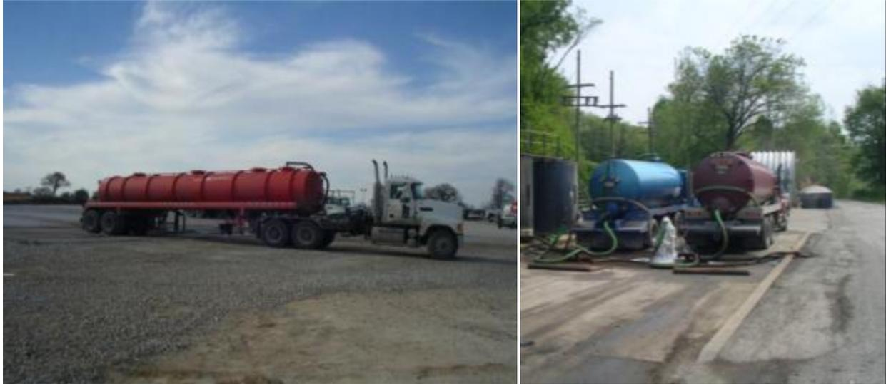
**Figure 12 – Pumping Unit Used to Move Water to Next Well Site**
