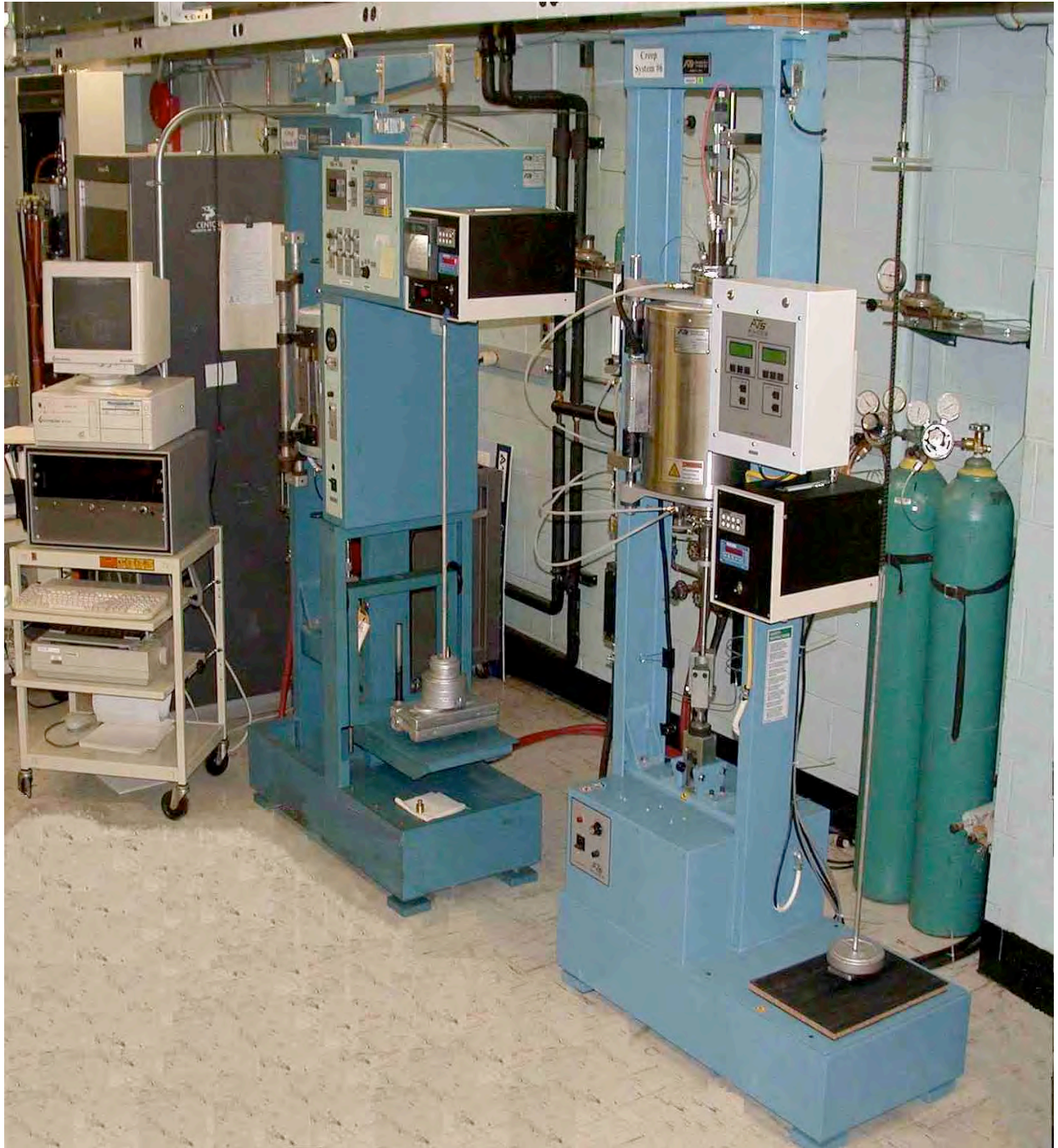
Figure 5. Overall view of lever-arm creep test facility for air and gas environments.
