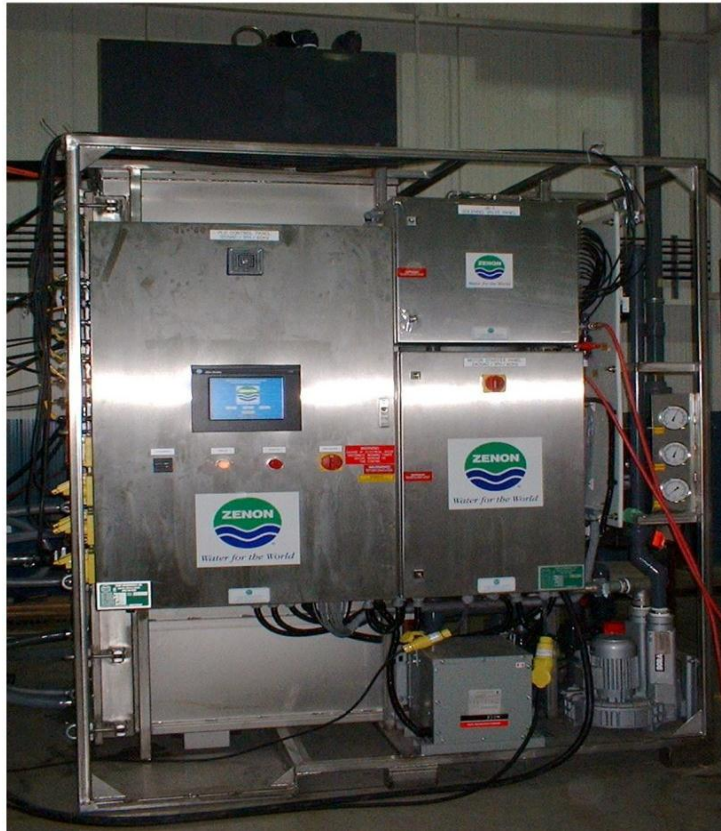
Figure 5.8: Pictogram of a typical pilot-scale GE ZeeWeed® 500 UF membrane filtration system (Permission to use photograph granted by GE Power & Water)
