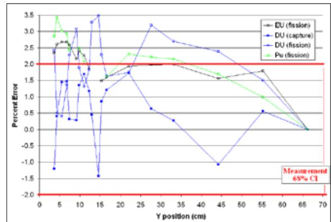
Fig. 11. Calculated foil reaction rate errors obtained using NEAMS tools.
