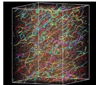
Fig. 7. Simulated dislocation-defect structure after plastic deformation in Fe-Cr-Ni steel.
