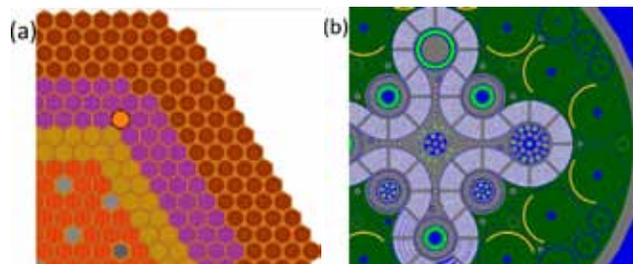
Fig. 9. Comparison of reactor core geometries: (a) Monju and (b) ATR.
