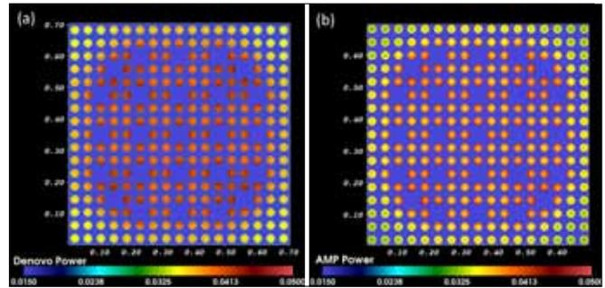
Fig. 1. Translation of Denovo output to AMP: (a) Cross section of fuel assembly showing Denovo-calculated power distribution. (b) The same data represented in the AMP mesh
