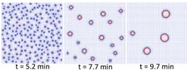
Fig. 6. Marmot 2D simulation of fission gas bubble growth during fuel annealing.
