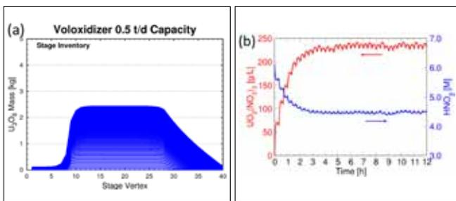
Fig. 5. Representative output data from reprocessing simulations: (a) Voloxidizer  $U_3O_8$  inventory profile. (b) Uranium and nitric acid outlet concentrations during dissolver startup transients.
