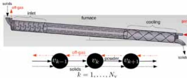
Fig. 4. Voloxidizer calciner with network representation of flows and holdup.
