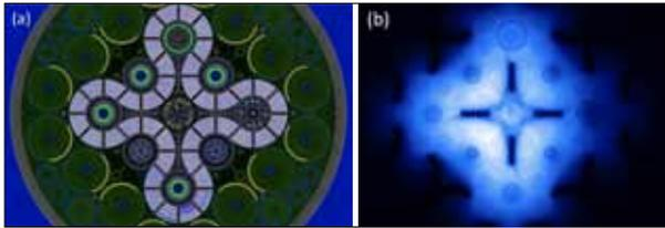
Fig. 2. Modeling the ATR core: (a) Sharp representation of core geometry. (b) Proteus prediction of thermal neutron flux.
