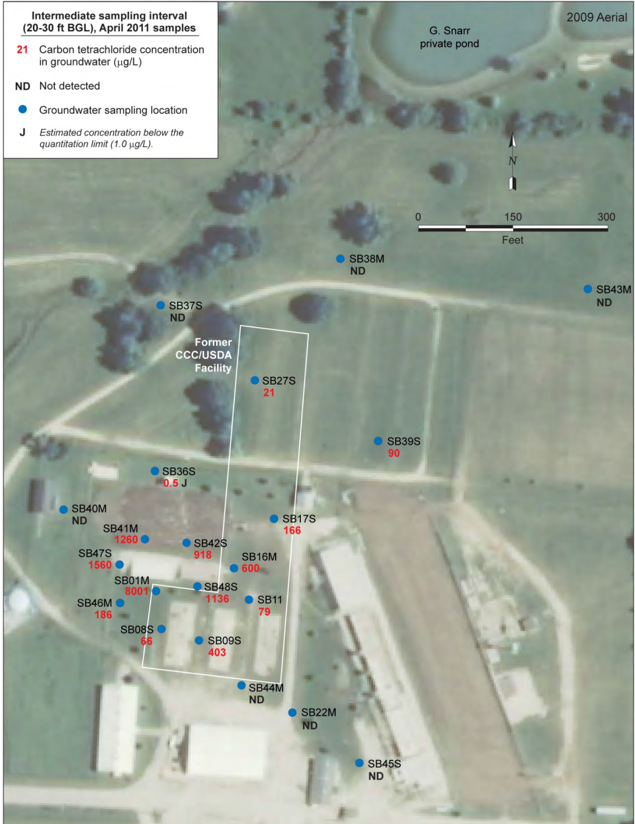
FIGURE 3.11 Lateral distribution of carbon tetrachloride in groundwater, as determined in the April 2011 sampling of temporary monitoring points in the intermediate sampling interval (20-30 ft BGL). Source of photograph: NAIP (2009).
