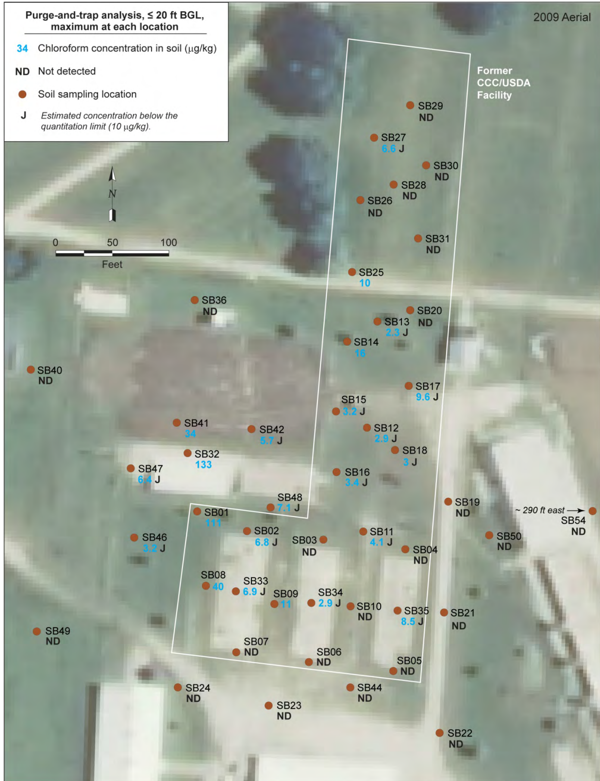
FIGURE 3.5 Lateral distribution of chloroform in shallow soils (≤ 20 ft BGL), as determined by purge-and-trap analysis. The maximum detected value is shown for each location. Source of photograph: NAIP (2009).
