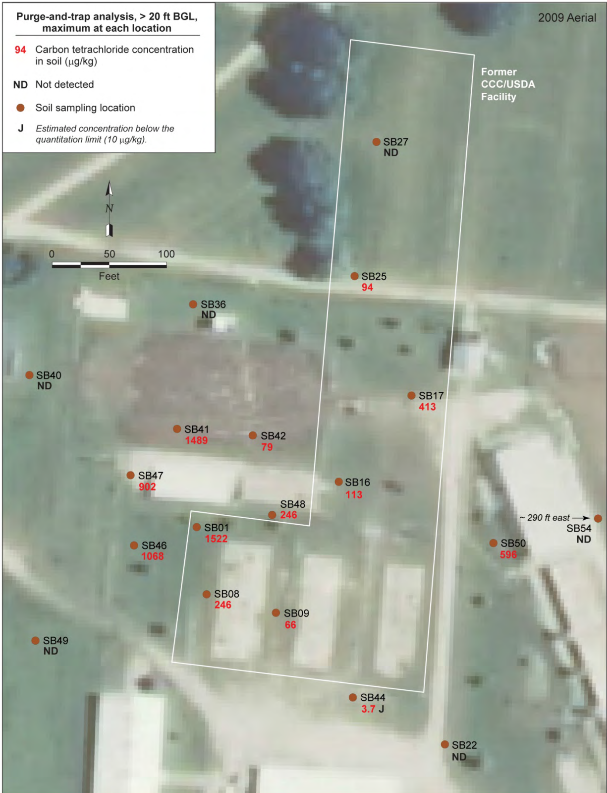
FIGURE 3.4 Lateral distribution of carbon tetrachloride in deeper soils (> 20 ft BGL), as determined by purge-and-trap analysis. The maximum detected value is shown for each location. Source of photograph: NAIP (2009).
