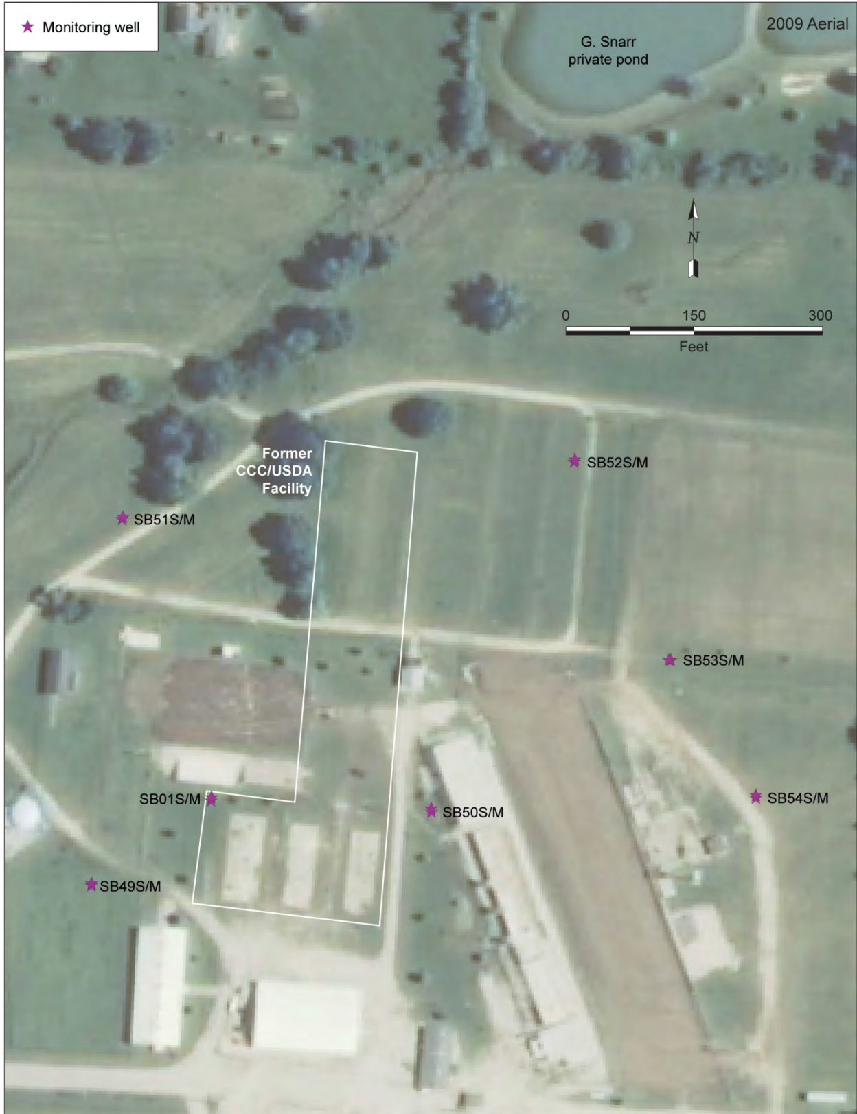
FIGURE 2.12 Locations of permanent monitoring wells equipped with automatic groundwater level recorders in May 2011. Source of photograph: NAIP (2009).
