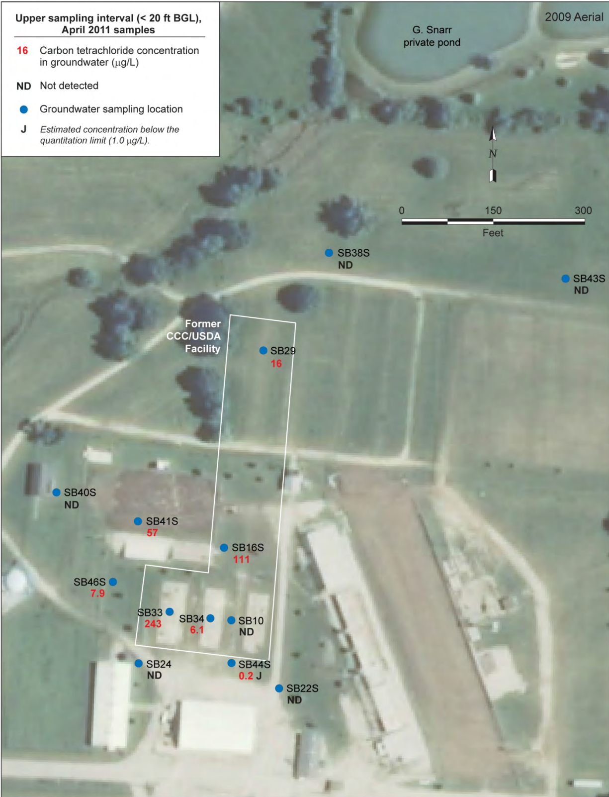
FIGURE 3.10 Lateral distribution of carbon tetrachloride in groundwater, as determined in the April 2011 sampling of temporary monitoring points in the upper sampling interval (< 20 ft BGL). Source of photograph: NAIP (2009).
