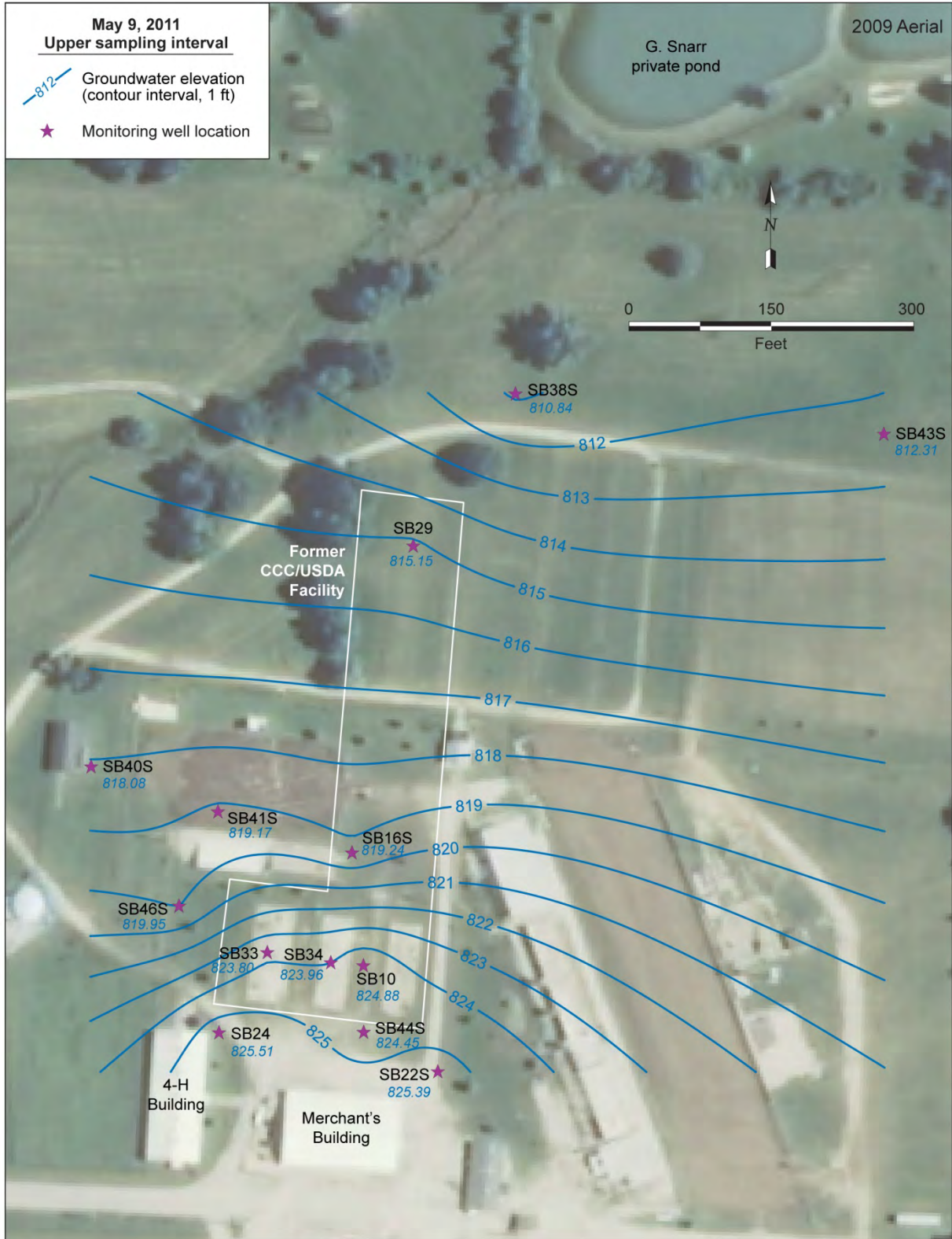
FIGURE 4.12 Interpreted potentiometric surface based on groundwater levels measured by hand in monitoring wells completed in the upper sampling interval on May 9, 2011. Source of photograph: NAIP (2009).
