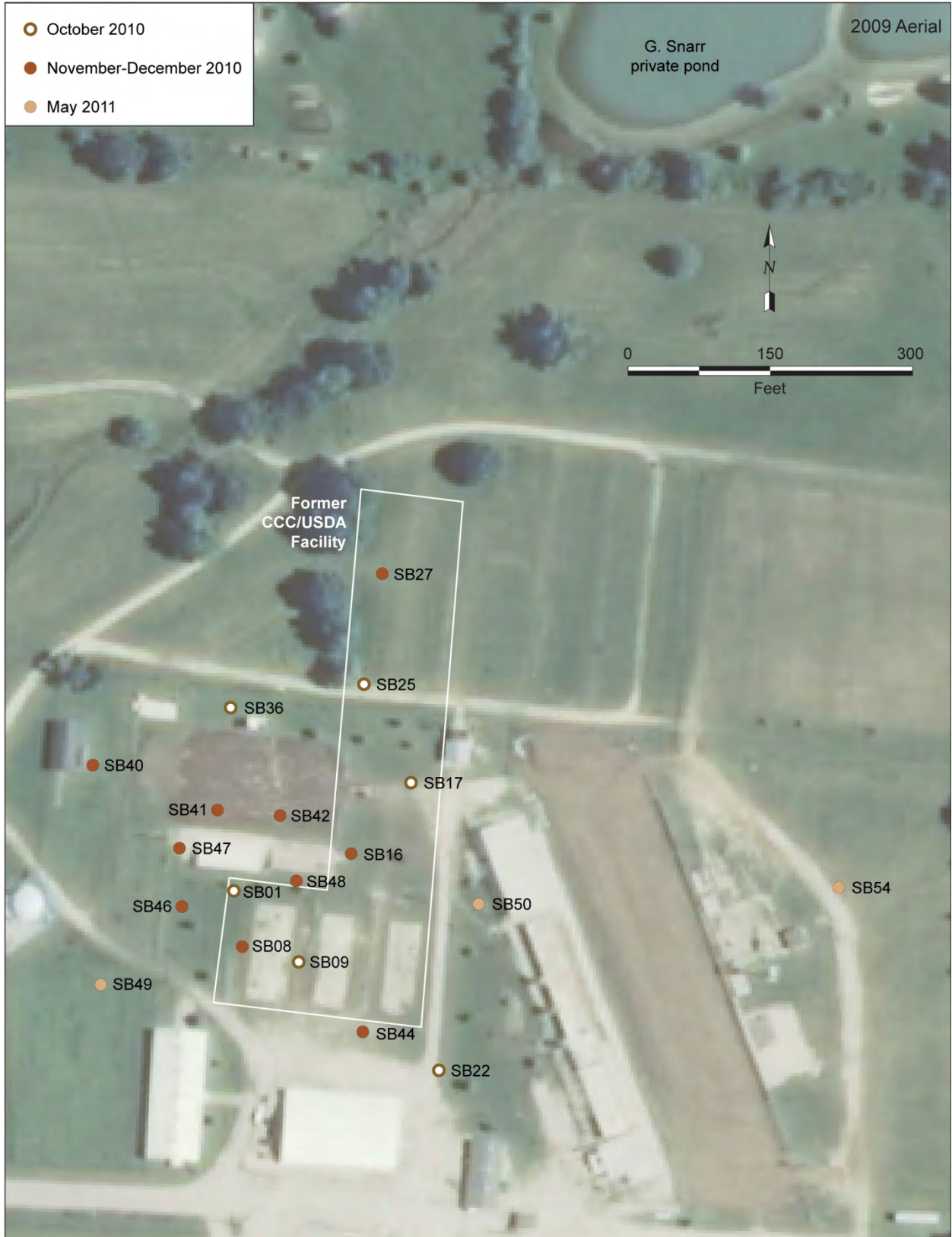
FIGURE 2.5 Locations of deeper soil sampling in October 2010, November-December 2010, and May 2011. Source of photograph: NAIP (2009).
