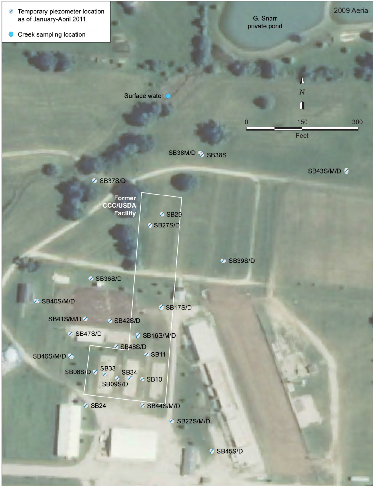
FIGURE 2.7 Locations of the 53 temporary groundwater monitoring points (piezometers) used for sampling and water level measurement in January-April 2011. Source of photograph: NAIP (2009).
