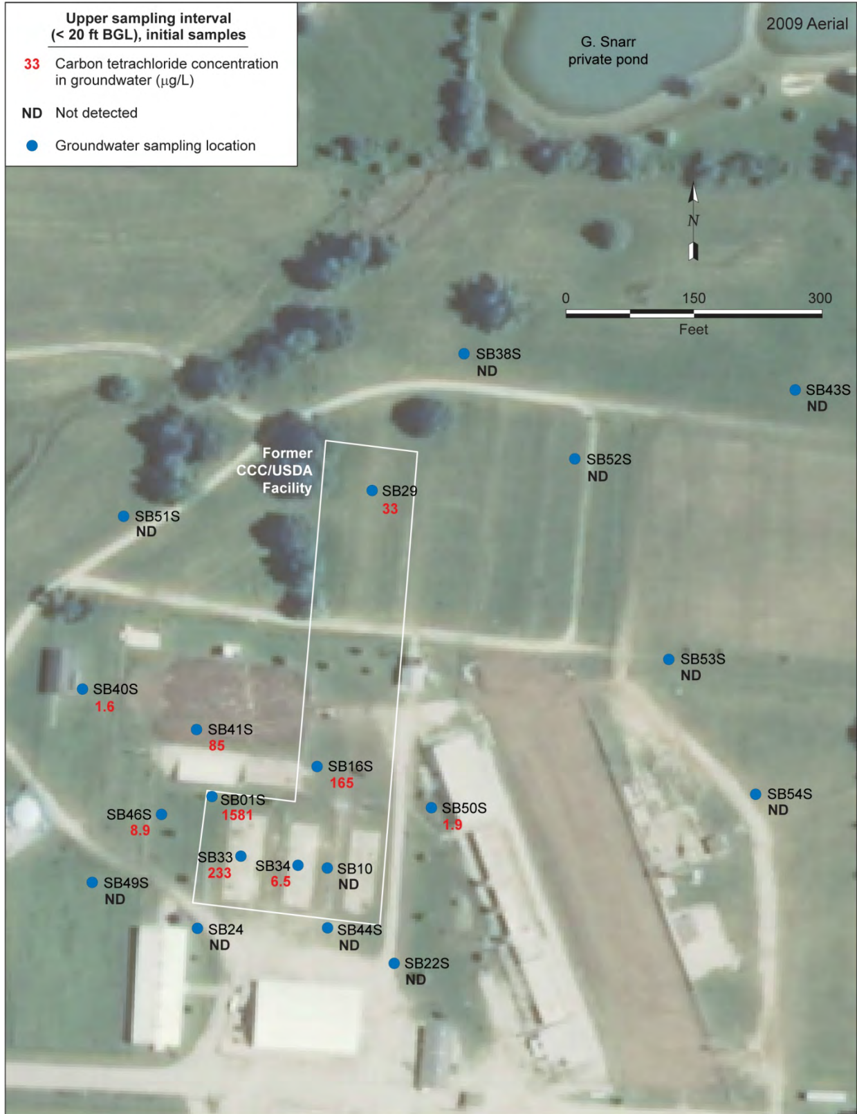
FIGURE 3.7 Lateral distribution of carbon tetrachloride in groundwater, as determined in the initial sampling (on various dates) of temporary and permanent monitoring points in the upper sampling interval (< 20 ft BGL). Source of photograph: NAIP (2009).
