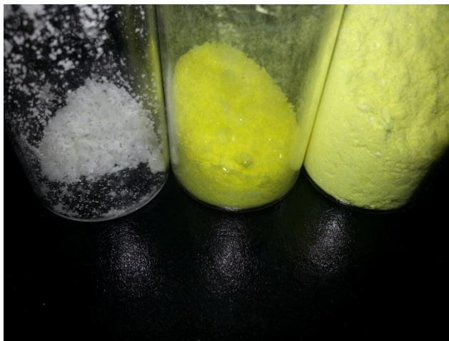
FIGURE 3 Photograph of Solids Isolated from Method 2: Hydrolysis Product (left), (\text{Bu}_4\text{N})_2[\text{Mo}_6\text{O}_{19}] (middle), and (\text{Bu}_4\text{N})_2[\text{Mo}_6\text{O}_{19}] and Hydrolysis Product Combined (right)
