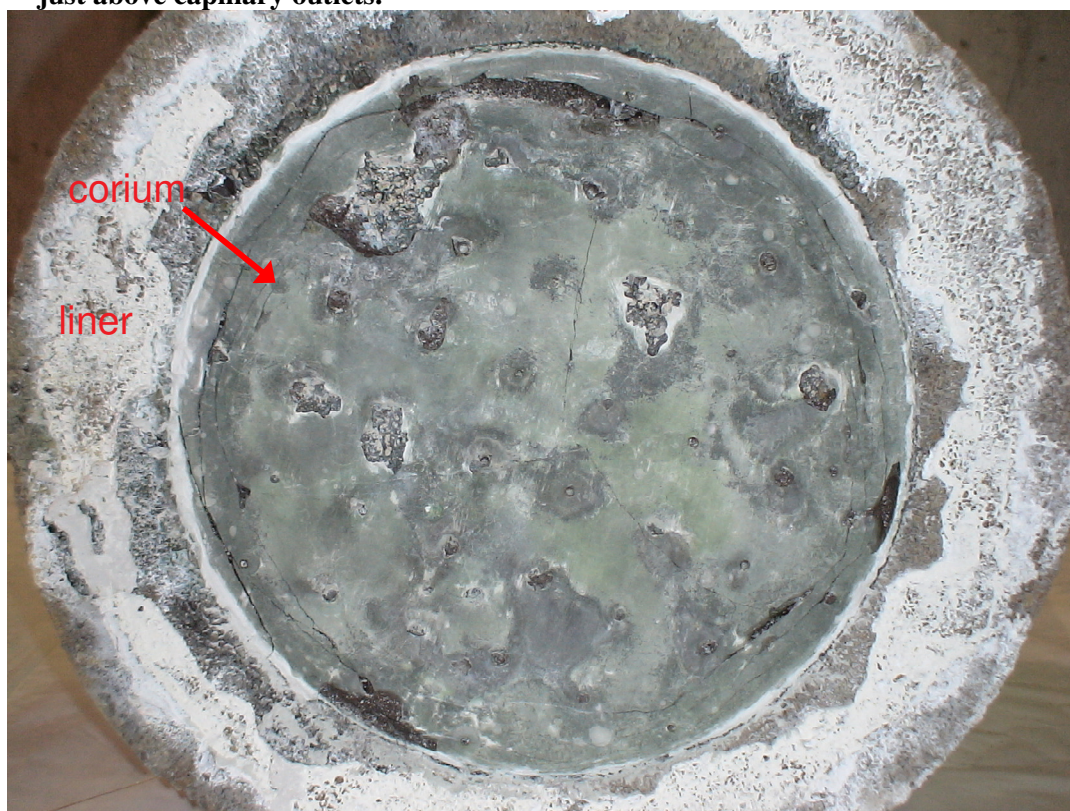
Figure A.18 Bottom view of ingot and liner. Note dimples at locations that were just above capillary outlets.
