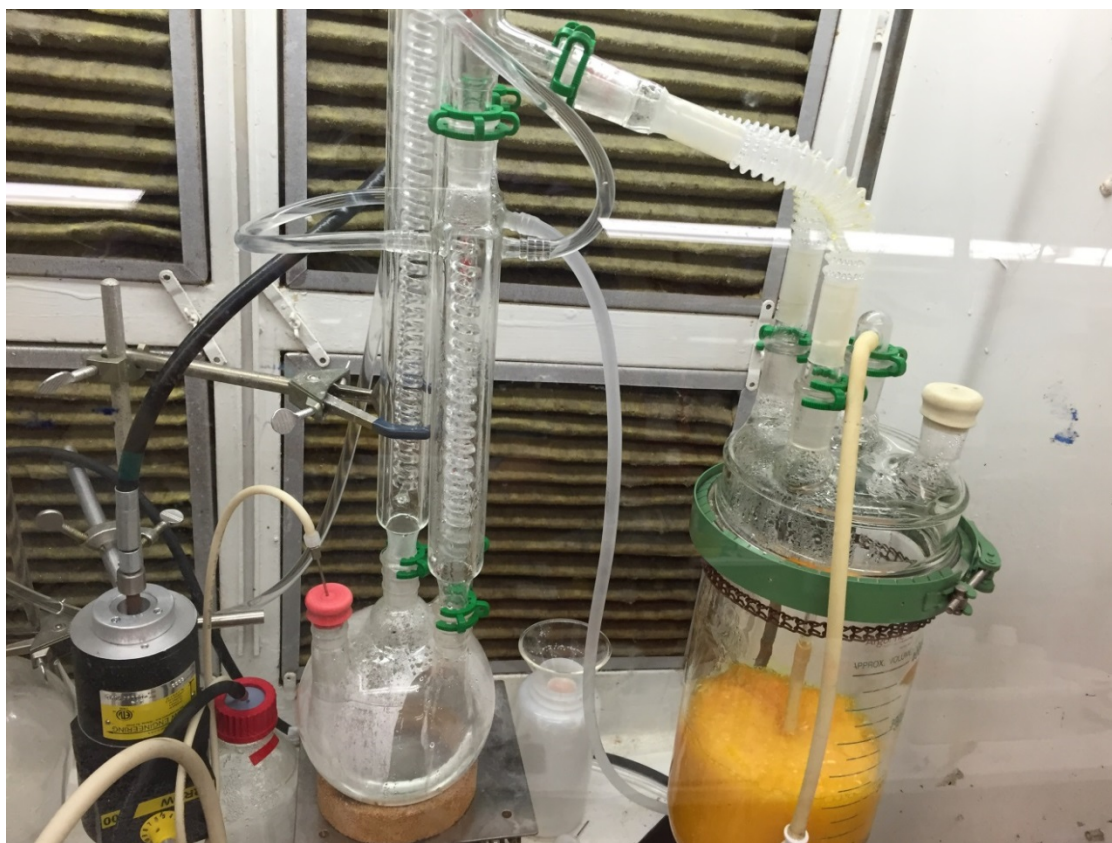
FIGURE 6 Flexible adapters used to connect condensers to dissolution vessel
