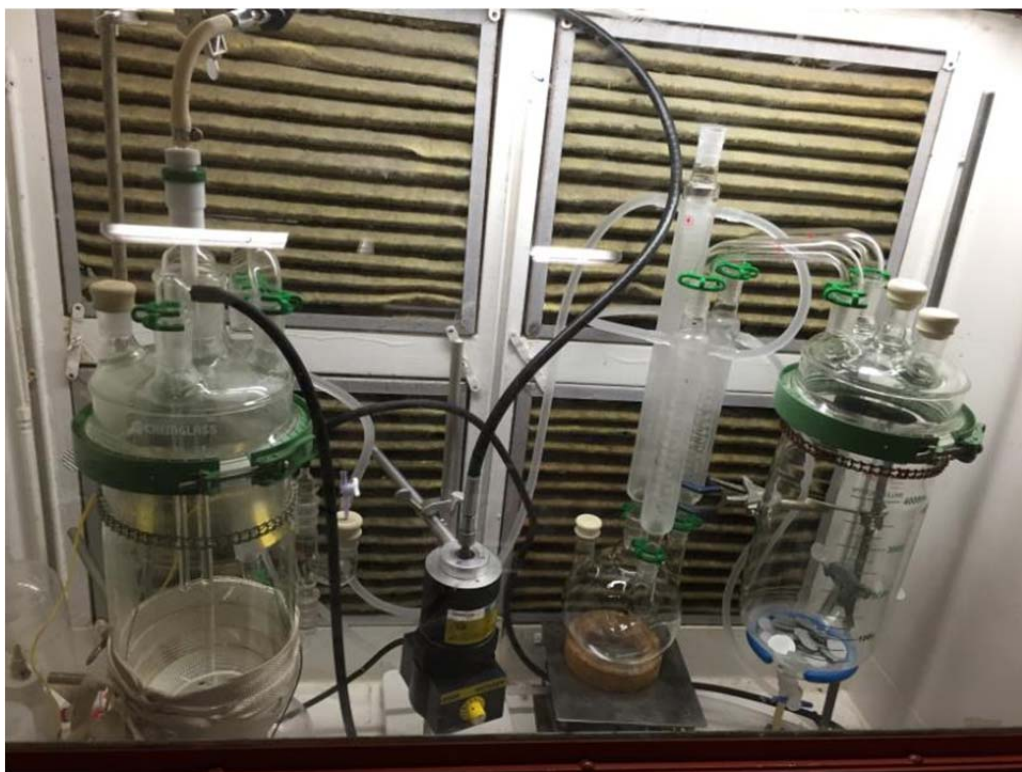
FIGURE 4 Setup used for dissolution of 300 g of sintered Mo disks
