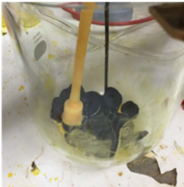
FIGURE 2 2-L vessel used for dissolution of 75 g Mo disks. Vapor released during dissolution was exhausted into ventilation.
