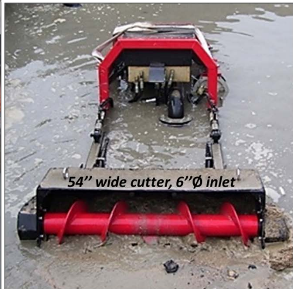
FIGURE 5-6 Tracked Radio-Remote-Controlled Cutter Suction Dredge (Source: Photos from Liquid Waste Technology, LLC, ROV SRD-6E specifications brochure)
