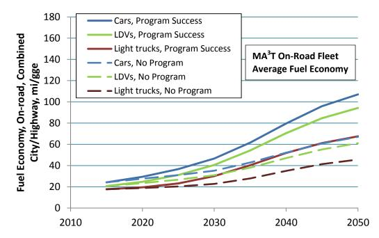
FIGURE 27 Average On-Road Fuel Economy of Cars, Light-Duty Trucks, and LDV Fleet for No Program (dashed lines) and Program Success (solid lines), Based on Market Projections of the MA<sup>3</sup>T Model
