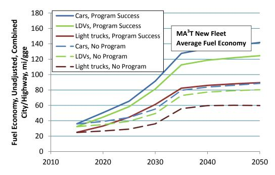
FIGURE 26 Fleet-Average Fuel Economy of New Cars, Light-Duty Trucks, and LDV Fleet for No Program (dashed lines) and Program Success (solid lines), Based on Market Projections of the MA<sup>3</sup>T Model
