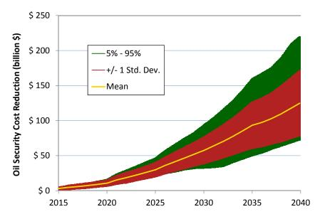
FIGURE 36 Estimated Reduction in Oil Security Costs Based on Projections of LDV Sales from the LAVE-Trans Model and HT Sales from the TRUCK Model, with Uncertainty Intervals
