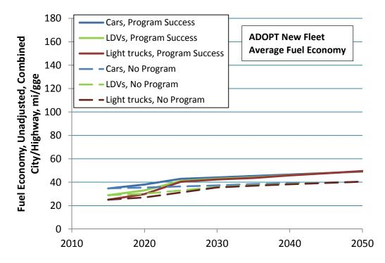
FIGURE 32 Fleet-Average Fuel Economy of New Cars, Light-Duty Trucks, and LDV Fleet for No Program (dashed lines) and Program Success (solid lines), Based on Market Projections of the ADOPT Model
