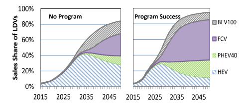
FIGURE 16 LDV Sales Shares by Powertrain Type for No Program (left) and Program Success (right), Projected by the LAVE-Trans Model
