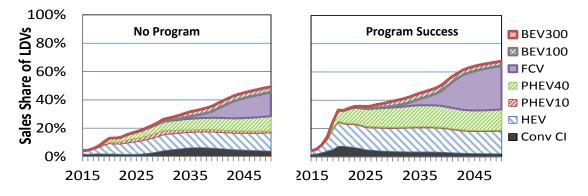
FIGURE 14 LDV Sales Shares by Powertrain Type for No Program (left) and Program Success (right), Projected by the LVCFlex Model
