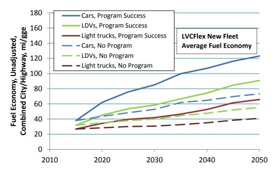
FIGURE 24 Fleet-Average Fuel Economies of New Cars, Light-Duty Trucks, and LDV Fleet for No Program (dashed lines) and Program Success (solid lines), Based on Market Projections of the LVCFlex Model
