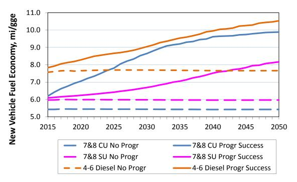
FIGURE 34 Fleet-Average Fuel Economy of New Medium- and Heavy-Duty Trucks for No Program (dashed lines) and Program Success (solid lines)
