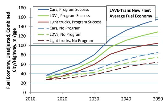
FIGURE 28 Fleet-Average Fuel Economy of New Cars, Light-Duty Trucks, and LDV Fleet for No Program (dashed lines) and Program Success (solid lines), Based on Market Projections of the LAVE-Trans Model
