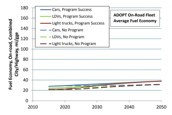
FIGURE 33 Average On-Road Fuel Economy of Cars, Light-Duty Trucks, and LDV Fleet for No Program (dashed lines) and Program Success (solid lines), Based on Market Projections of the ADOPT Model
