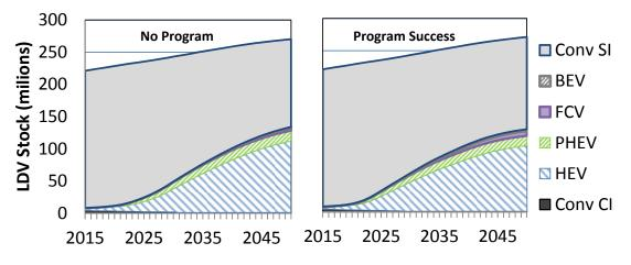
FIGURE 23 LDV stock by powertrain type for No Program (left) and Program Success (right), Projected by the ADOPT model
