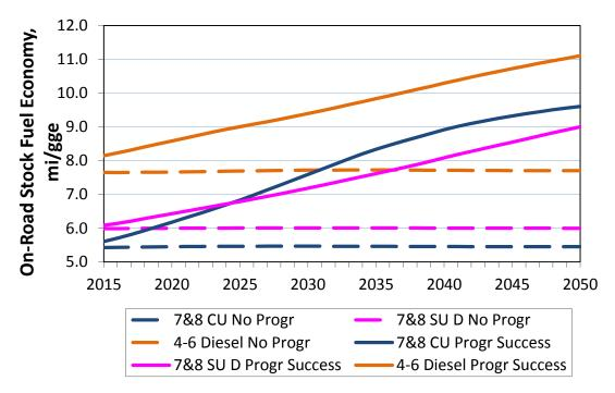
FIGURE 35 Average On-Road Fuel Economy of Medium- and Heavy-Duty Trucks for No Program (dashed lines) and Program Success (solid lines)
