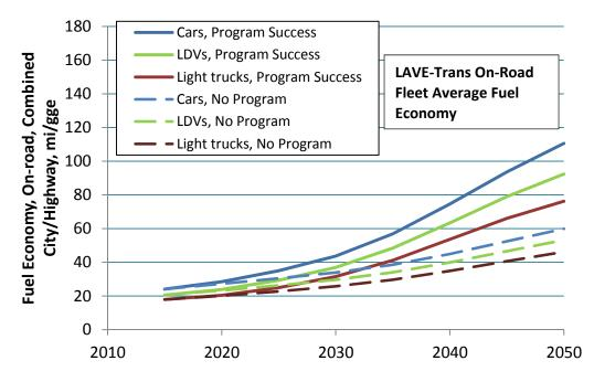
FIGURE 29 Average On-Road Fuel Economy of Cars, Light-Duty Trucks, and LDV Fleet for No Program (dashed lines) and Program Success (solid lines), Based on Market Projections of the LAVE-Trans Model
