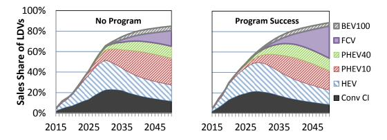
FIGURE 17 LDV Sales Shares by Powertrain Type for No Program (left) and Program Success (right), Projected by the ParaChoice Model
