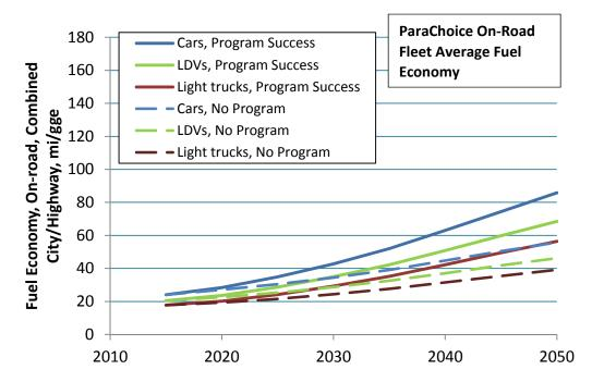
FIGURE 31 Average On-Road Fuel Economy of Cars, Light-Duty Trucks, and LDV Fleet for No Program (dashed lines) and Program Success (solid lines), Based on Market Projections of the ParaChoice Model
