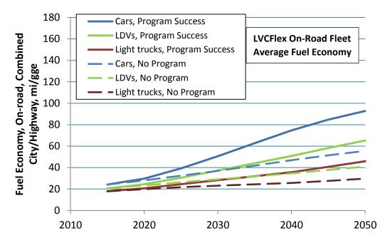
FIGURE 25 Average On-Road Fuel Economy of Cars, Light-Duty Trucks, and LDV Fleet for No Program (dashed lines) and Program Success (solid lines), Based on Market Projections of the LVCFlex Model
