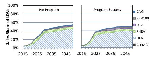
FIGURE 18 LDV Sales Shares by Powertrain Type for No Program (left) and Program Success (right), Projected by the ADOPT Model
