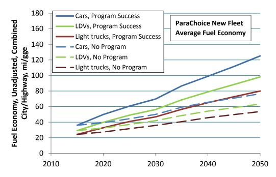
FIGURE 30 Fleet-Average Fuel Economy of New Cars, Light-Duty Trucks, and LDV Fleet for No Program (dashed lines) and Program Success (solid lines), Based on Market Projections of the ParaChoice Model
