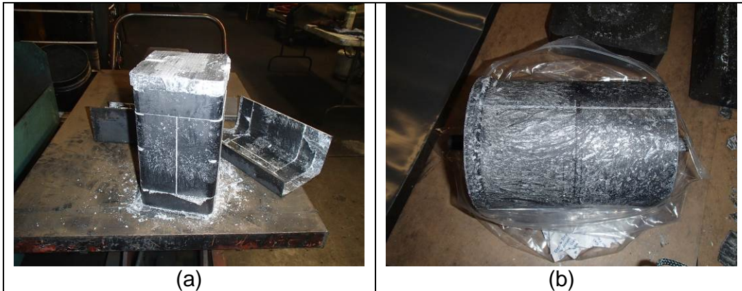
Figure 10-34. Prototype after the PCM infiltration.
