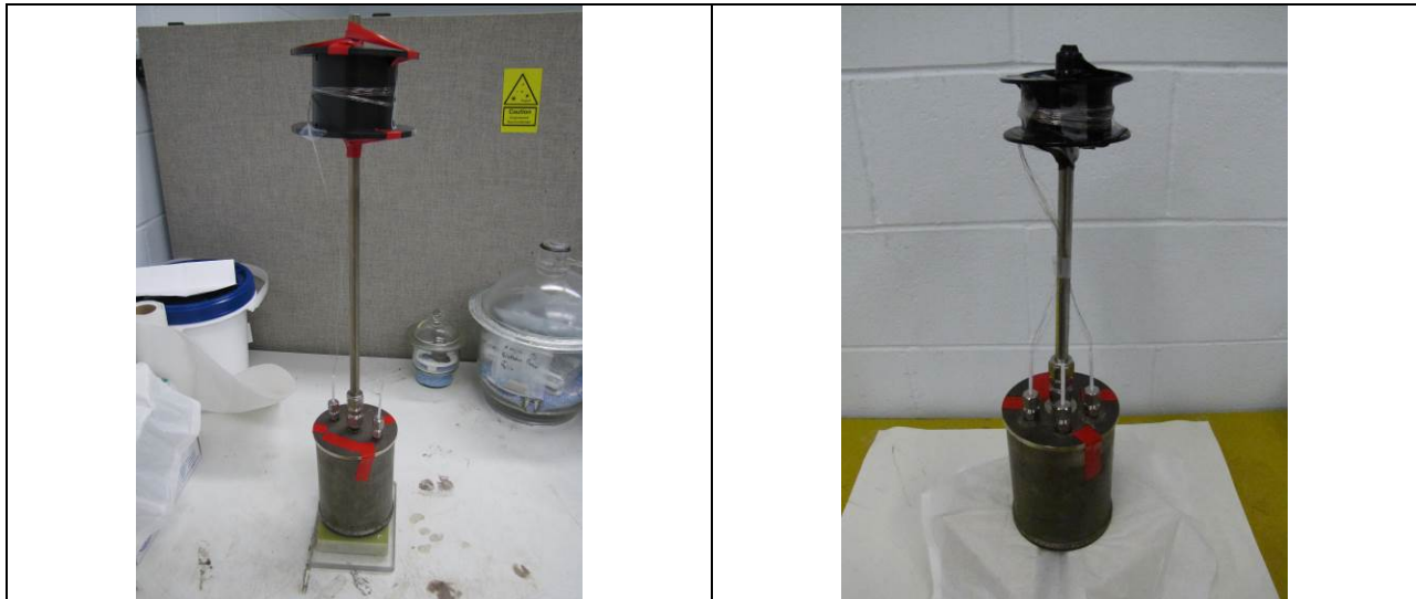
Figure 10-39. Prototypes after installation of top plate and TCs: (a) 1-2 and (b) 1-3.
