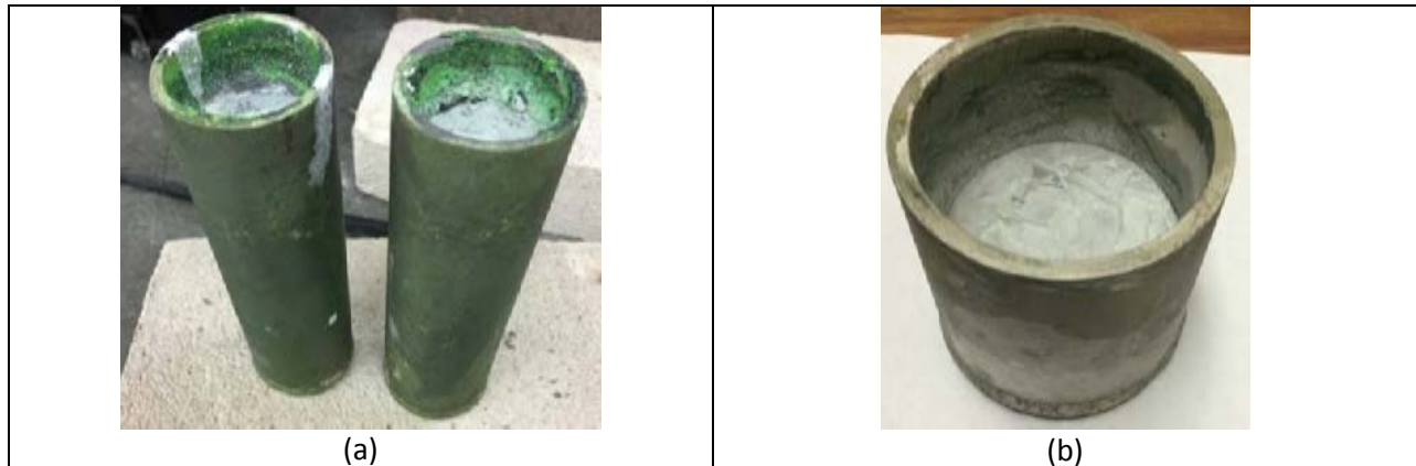
Figure 9-53. Photographs of the crucibles after corrosion tests: (a) Two nickel crucible used in Test 1 to 7 and (b) nickel crucible used in Test 8 where anhydrous salt coupled with argon sparging was used.
