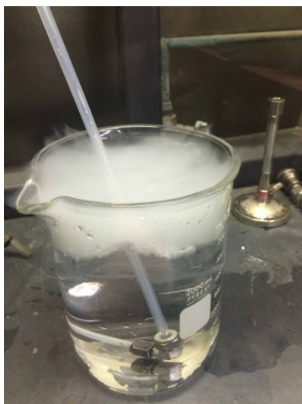
Figure 9-52. HCl fog formed above the water surface in the beaker. Detailed information on the experimental setup is shown in Figure 9-4.
