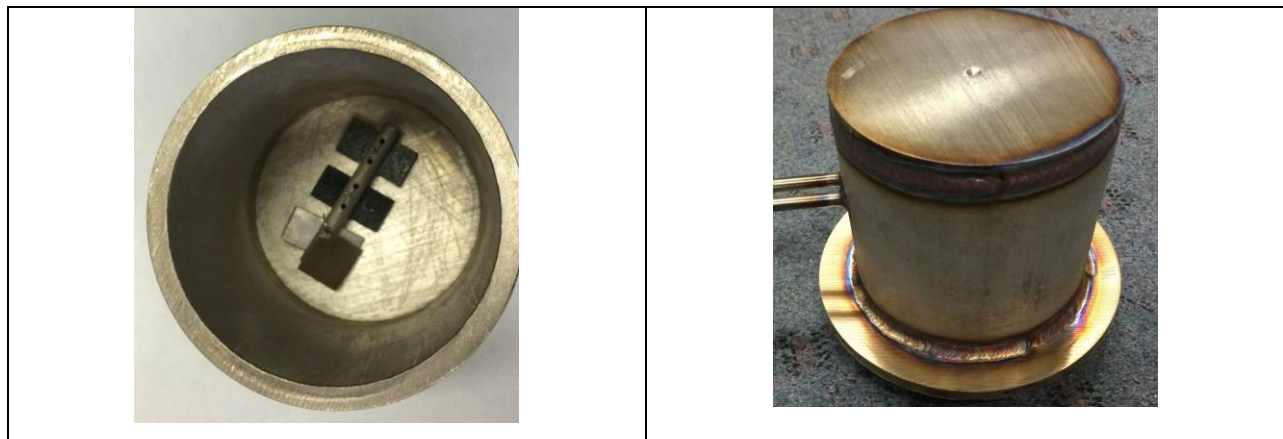
Figure 9-3. The inner nickel crucible with samples inside (left), and welded 316 stainless steel container with an inner nickel crucible filled with samples and salt powder (right).
