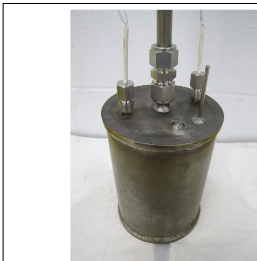
Figure 10-42. Prototype 1-2 after top welding completed.
