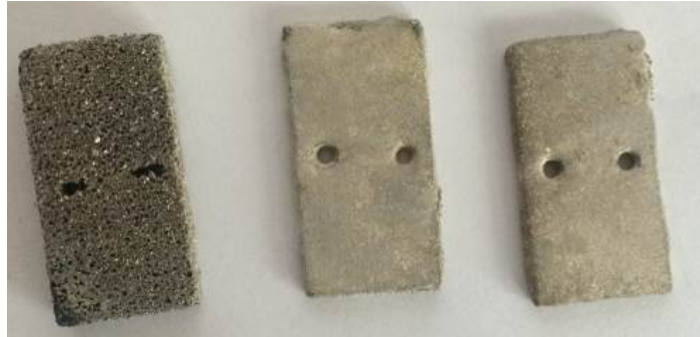
Figure 9-42. Photographs of 3-dip SiC-coated graphite foam (1 coupon, left) and BNi-coated 800H (2 coupons, middle and right) after Test 7.
