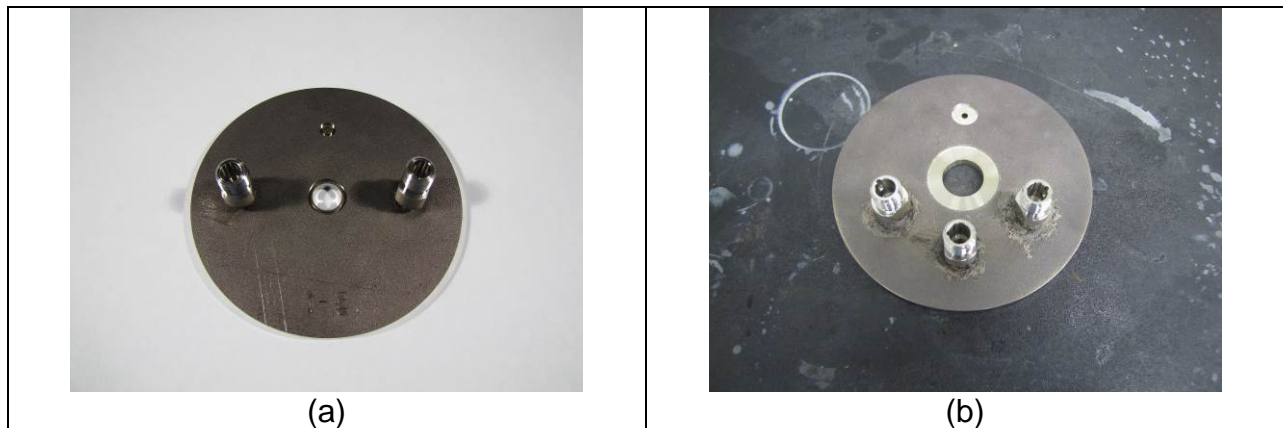
Figure 10-38. Top plates for prototypes after feedthroughs installed: (a) 1-2 and (b) 1-3.
