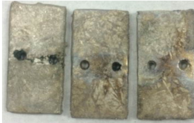
Figure 9-36. Photographs of three BNi-4-coated 800H samples after Test 6c.
