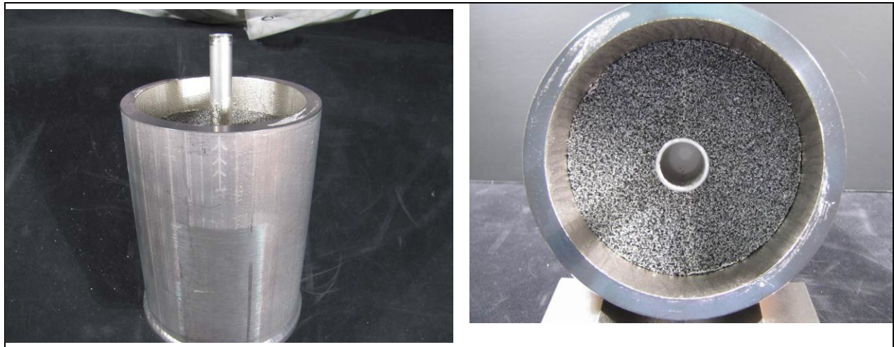
Figure 10-33. The first series prototype (1-4) after the vacuum brazing process.
