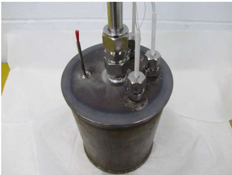
Figure 10-44. Prototype 1-3 after top welding completed.
