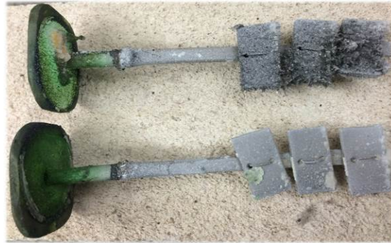
Figure 9-19. Photographs of uncoated graphite foam and BNi-4-coated 800H immediately after Test 5.
