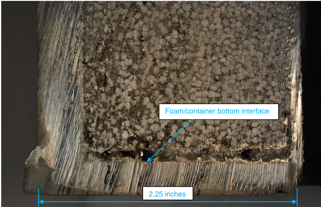
Figure 11-26. Bottom section of prototype 1-2 after 750°C/250 h exposure.
