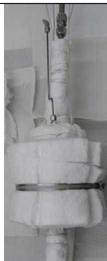
Figure 10-43. Prototype 1-2 after placing insulation.
