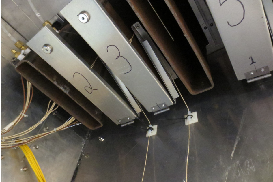
Figure 96: Closure flaps used to remotely actuate a riser blockage
