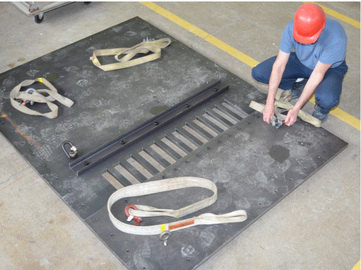
Figure 12: Top plate which bears the weight of the twelve riser ducts
