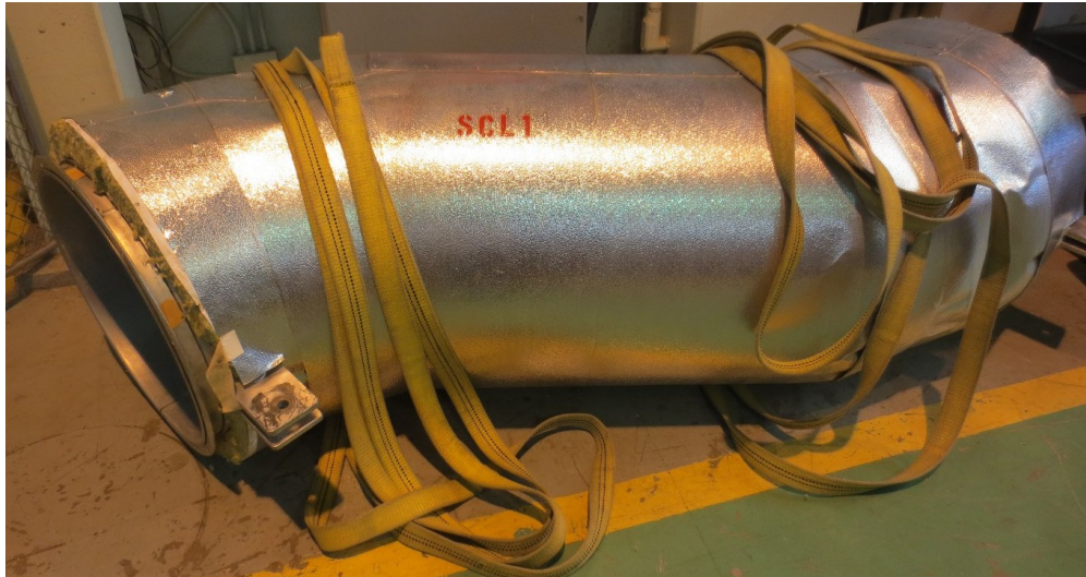
Figure 121: Removed south chimney section of air-based NSTF
