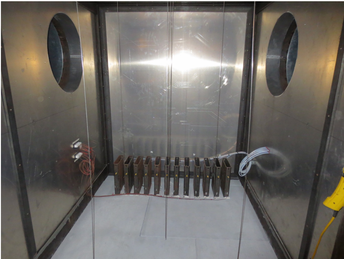
Figure 13: View into the outlet plenum from opened east wall. False west wall visible behind riser tubes
