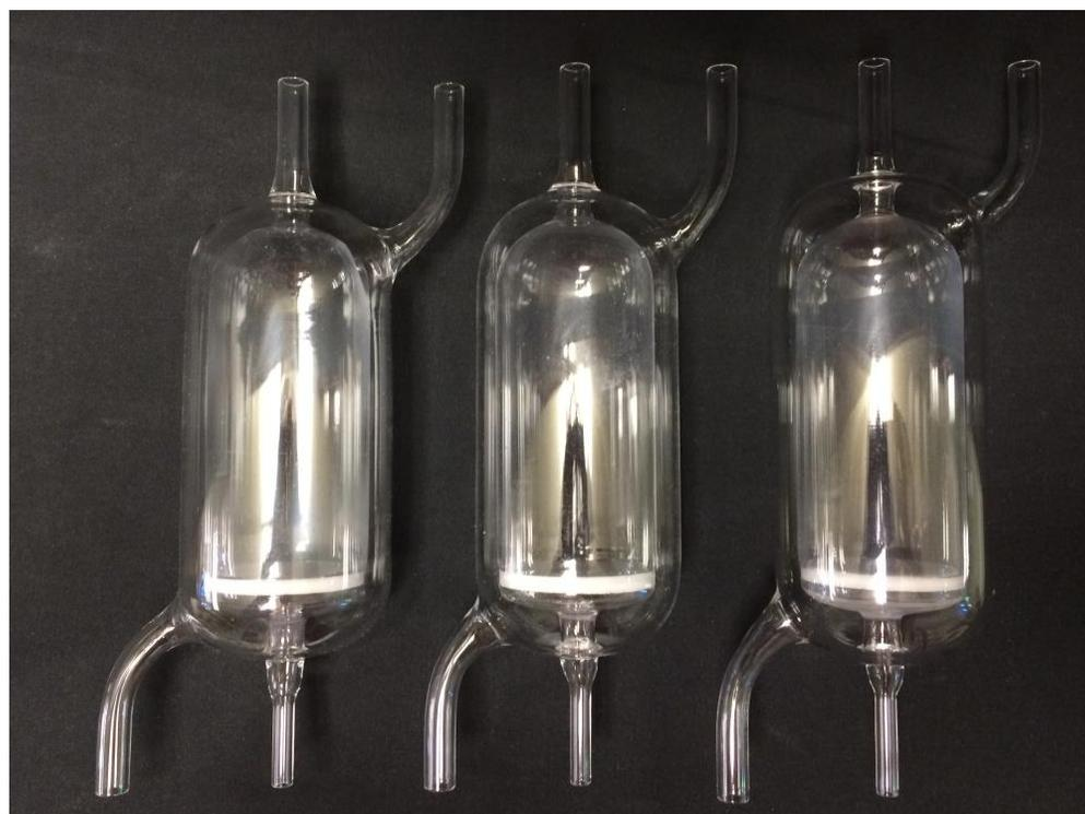
**FIGURE 11** Quartz irradiation vessels used during linac Mo-ABO trials. The vessels were quartz with a quartz-fritted funnel, and a quartz jacket for water cooling.
