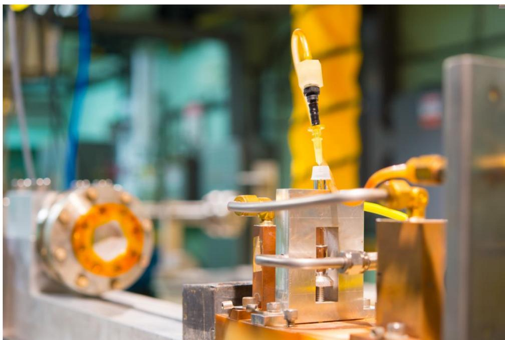
**FIGURE 1** <sup>99</sup>Mo-ABO irradiation system at VDG. Beam line exit window can be seen on the left. The <sup>99</sup>Mo-ABO target holder is on the right.
