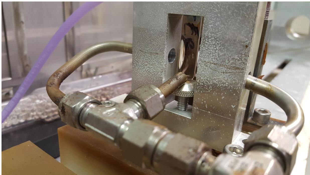
**FIGURE 2** Three-pronged compressed air cooling system of  $^{99}\text{Mo}$ -ABO irradiation system at the VDG. The sample is located within the center of the aluminum block.
