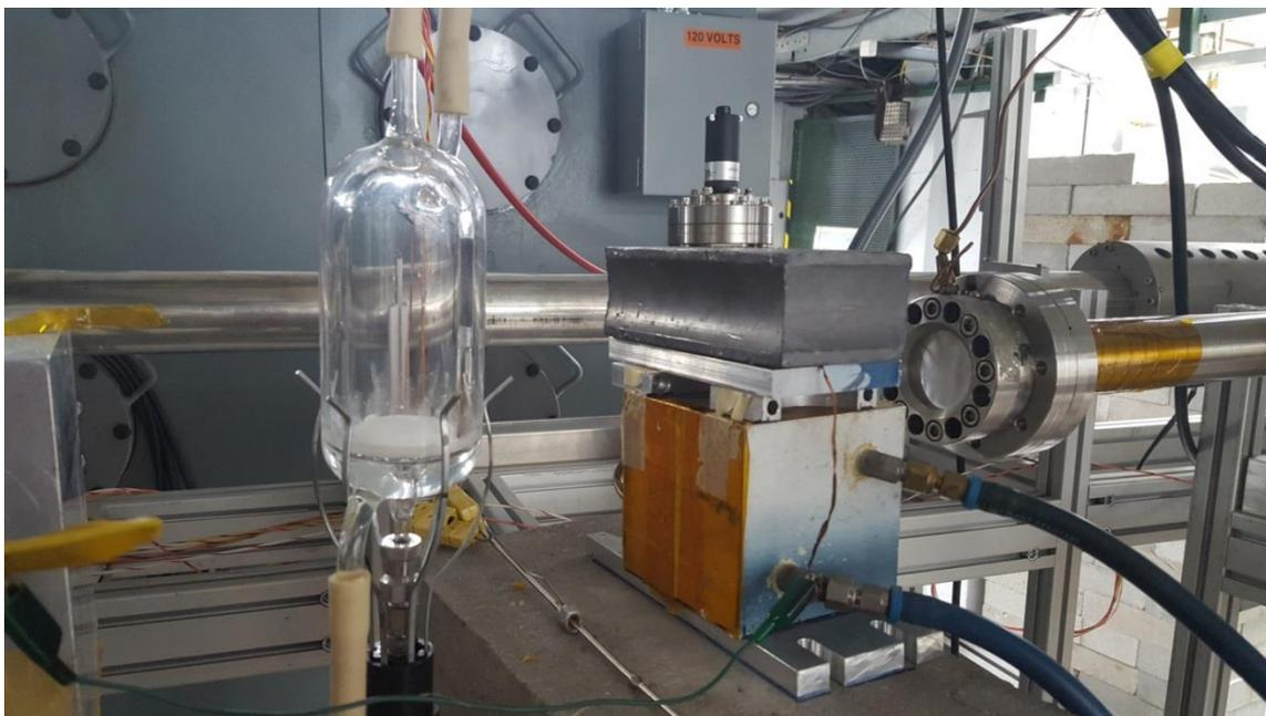
**FIGURE 23** Mo-ABO precipitated in quartz vessel prior to irradiation. An aluminum window was used during these irradiations. The beam was spread with magnets and collimated with a lead brick and water-cooled beam stop. Hose clamps were used during all irradiations, not shown here.
