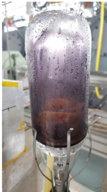
**FIGURE 26** Discoloration of Mo-ABO solid (visible through the darkened quartz walls). The movement of the Mo-ABO solid from the frit was attributed to the introduction of the wash solution from the bottom of the vessel.
