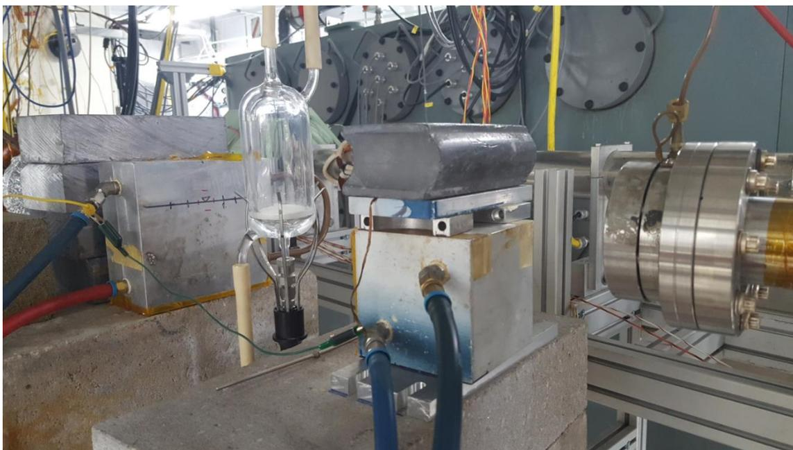
**FIGURE 24** Alternative view of Mo-ABO precipitated in quartz vessel prior to irradiation. Water-cooled beam stops can be seen between the beam window and the irradiation vessel, as well as behind the irradiation vessel. Hose clamps were used during all irradiations, not shown here.
