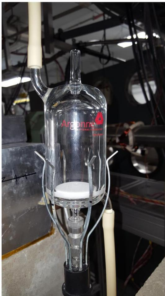
**FIGURE 22 Jacketed quartz irradiation vessel with Mo-ABO precipitated on the frit. Cooling lines are shown in the image. Chilled water from a recirculating bath was introduced from the bottom and expelled from the top. A thin layer of Mo-ABO is almost invisible to the eye.**
