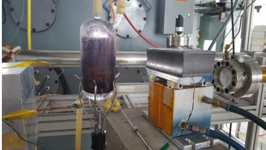
**FIGURE 25** Mo-ABO precipitated in quartz vessel after irradiation. The quartz darkened from exposure to the electron beam. Hose clamps are observed for the water cooling lines. Condensation can be seen on the exterior of the vessel. The condensation was from atmospheric water and does not represent a breach of containment.
