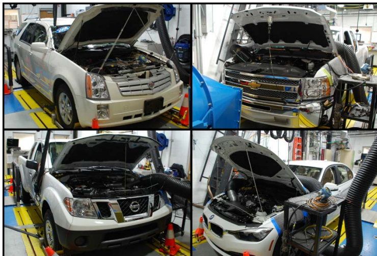
Figure 3.3.1. Vehicles installed on chassis dyno for fuel economy testing.
