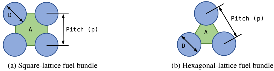
Figure 4.3: Fuel bundles in (a) square-lattice, typically seen in light water reactor designs; and (b) hexagonal-lattice, typically seen in sodium fast reactor designs.
