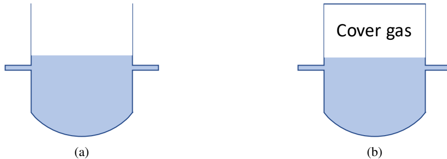
Figure 4.12: The PBLiquidVolume concept used in SAM. (a) PBLiquidVolume with ambient pressure as its reference pressure; (b) PBLiquidVolume with an external CoverGas to specify its reference pressure.
