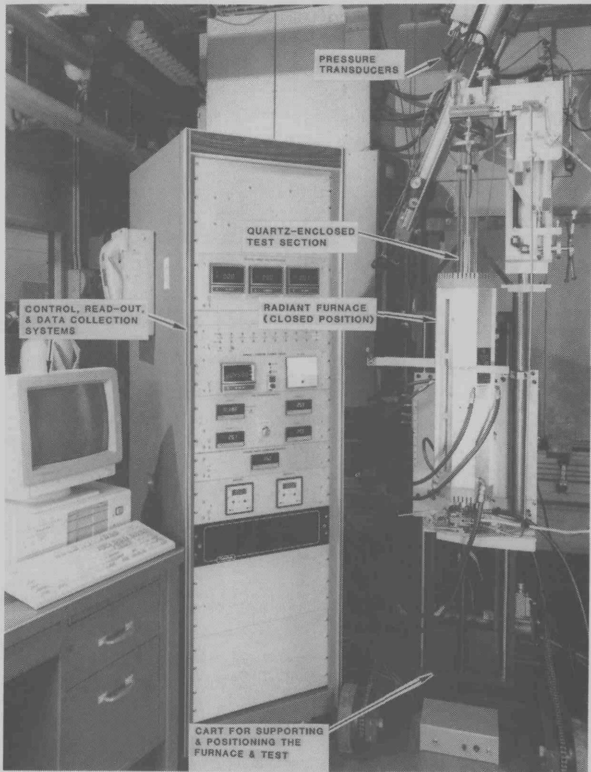
Fig. 1. Whole Pin Furnace Test Apparatus (ANL Neg. No. 7775)
