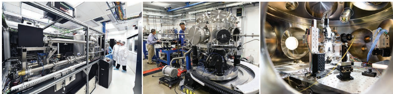
Fig. 1. The DCS Laser Shock Station. Above, left to right: the 100-J laser system, the highly flexible interactive chamber with translation stage and 135° rotation, and the sample holder and optics for x-ray and optical diagnostics inside the interactive chamber. Below: A schematic of the Laser Shock Station. From X. Wang et al., Rev. Sci. Instrum. 90 , 053901 (2019). Published under license by AIP Publishing
