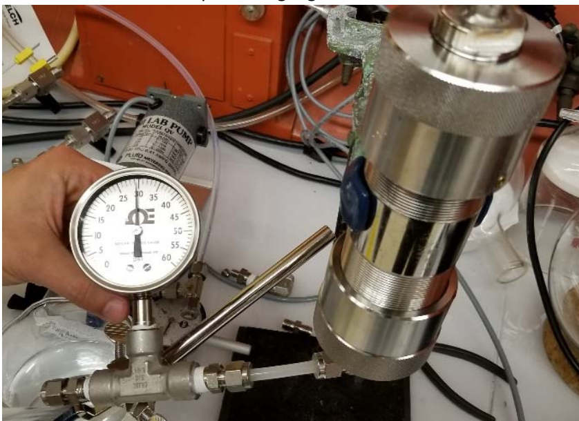
Figure 7: Column with pressure gauge attached
