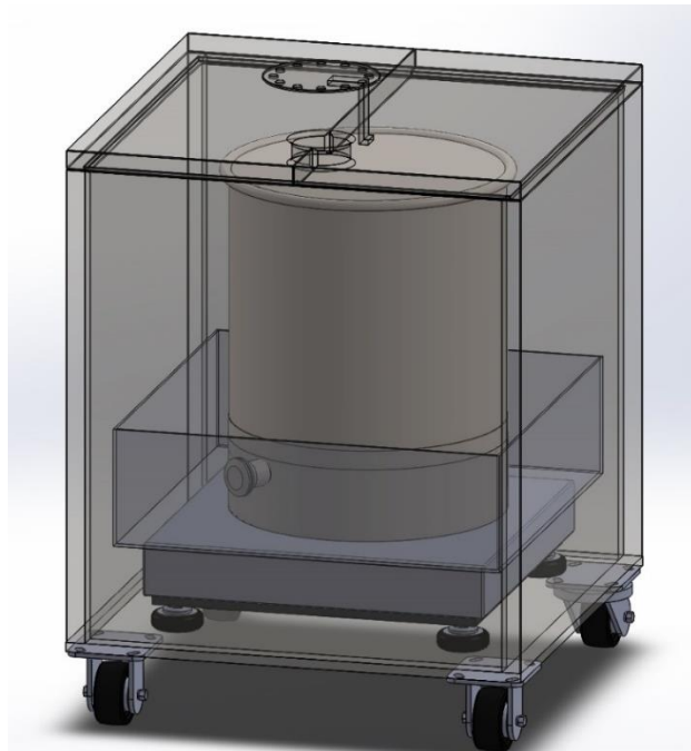
FIGURE 2.3.2.7.1 Drawing of the verification tank resting on its balance inside the shielded verification cart
