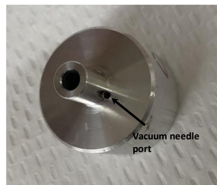
FIGURE 2.4.2.4.4 D-type aluminum needle adapter with side port for vacuum line
