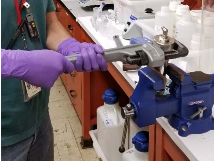
Figure 4: Tightening the top collar using a pipe-wrench and vice. Make sure inlet and outlet point the same direction.
