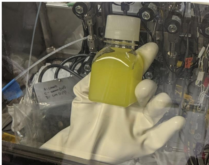
FIGURE 3.3.1.1 Uranyl peroxide precipitate in target solution that was extracted from the system prior to the first irradiation
