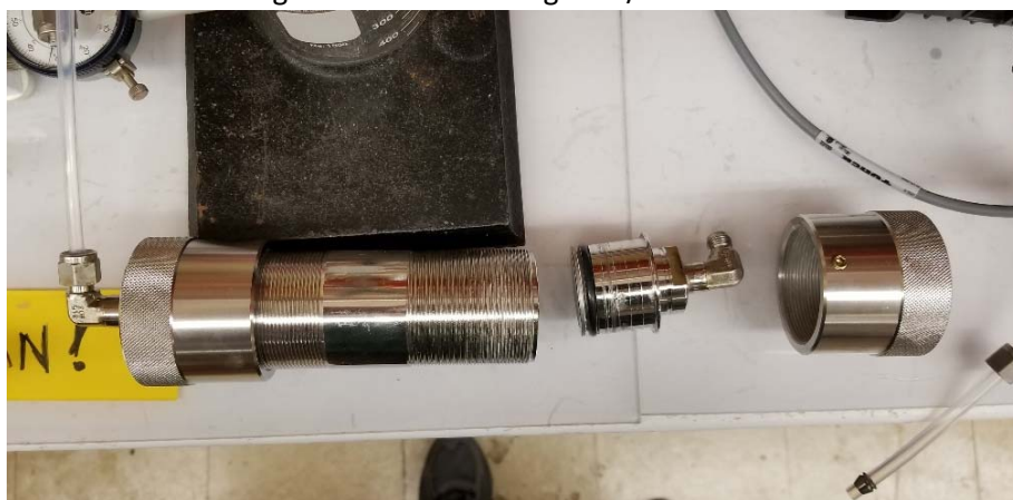
Figure 1: Column with bottom frit and collar in place and connected to tubing. Top frit and collar also included
