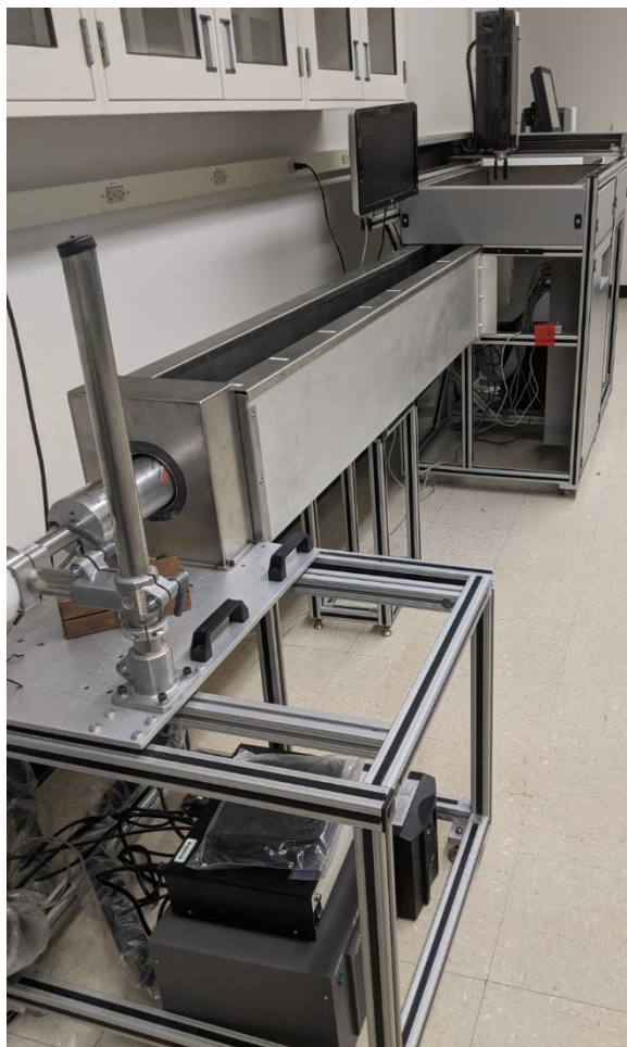
FIGURE 2.5.2.2 Mechanically cooled coaxial detector coupled to an autosampling unit with a shielded canyon for counting
