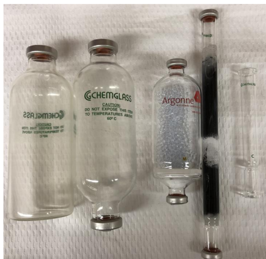
FIGURE 2.4.2.4.1 LMC glassware, plastic coated except for the fritted-glass column. From left to right: flat-bottom bottle, double-sided bottle, 51-mm fritted-glass column containing ~20 mL of glass beads, AgC/ZrO/AC column, charcoal filter column (shown empty). All glassware uses crimps to hold septa in place.
