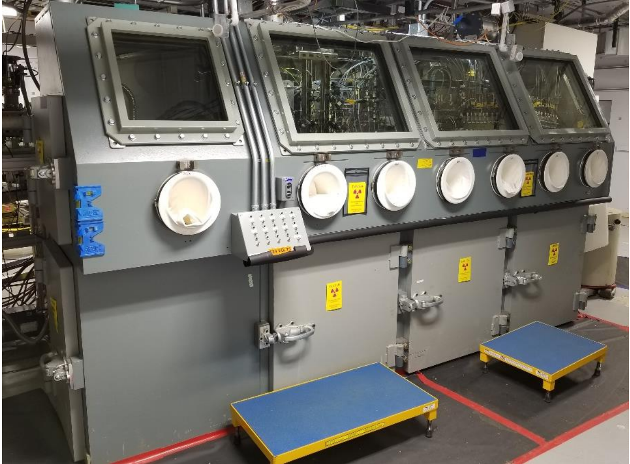
FIGURE 2.3.2.2.1 Image of the recovery glovebox with access port on the left. The three main windows and three cabinets discussed are to the right of the switch panel in the image.
