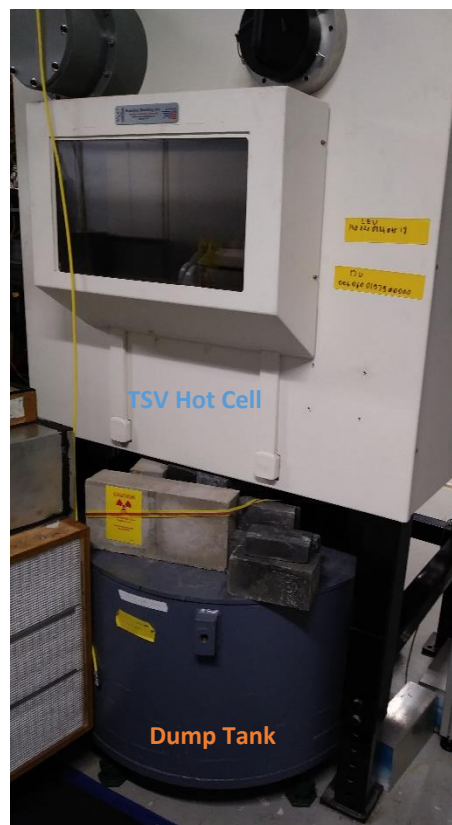
FIGURE 2.3.2.5.1 Image showing the relationship between the Dump Tank and TSV Hot Cell. These were connected via L-shaped transfer lines shielded by lead bricks (seen in picture). Image showing the relationship between the Dump Tank and TSV Hot Cell. These were connected via L-shaped transfer lines shielded by lead bricks (seen in picture).
