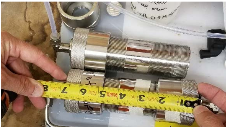
Figure 5: Overall length of the column is 6 \frac{3}{4} " once tightened.
