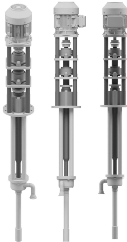
Figure 8 – Isometric and elevation views of the custom designed high-temperature pump.
