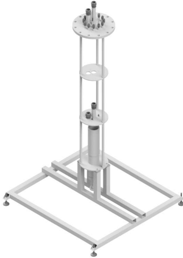
Figure 15 – Isometric view of the test section mounted to its assembly stand. Test section assembly begins by mounting the baseplate to the vertical support struts. Then the test section is assembled vertically from the baseplate, layering on each component above.
