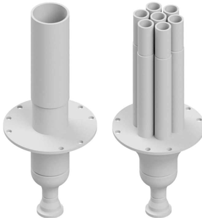
Figure 2 – Solid models of the Full-Scaled (left) and Pseudo-Scaled (right) test sections. These sections have been designed to represent a single handling socket and an array of scaled sockets, respectively.
