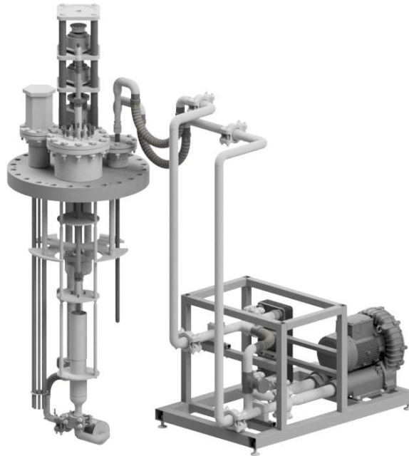
Figure 27 – Isometric view of the argon cooling system connected to F-STAr’s cooler. The loop and F-STAr are connected by flexible bellows hoses which will absorb any thermal expansion, dampen vibrations, and accommodate some misalignment.
