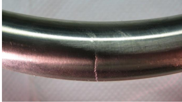
Figure 3. 7 A picture of the U-bend tube specimen after termination of the SCC test [26].
