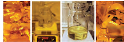
Add HNO 3 Heating After cooling Collect to GB
