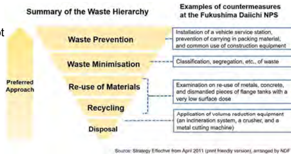
Fig. Summary of waste hierarchy at the NDA, UK, and countermeasures at the Fukushima Daiichi NPS
