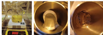
HNO 3 dissolution Dry up filter Residue after incineration filter incineration
