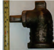
A 480-mil throat ID Terry nozzle and elbow connector. The outlet is a rounded square of 9/16 inch.
