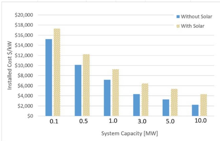
**Figure 3-15 Estimated Capital Costs for H-mcs-PSH plant with and without Solar Component (Source: T. Eldredge and H. Medina from Liberty University)**
