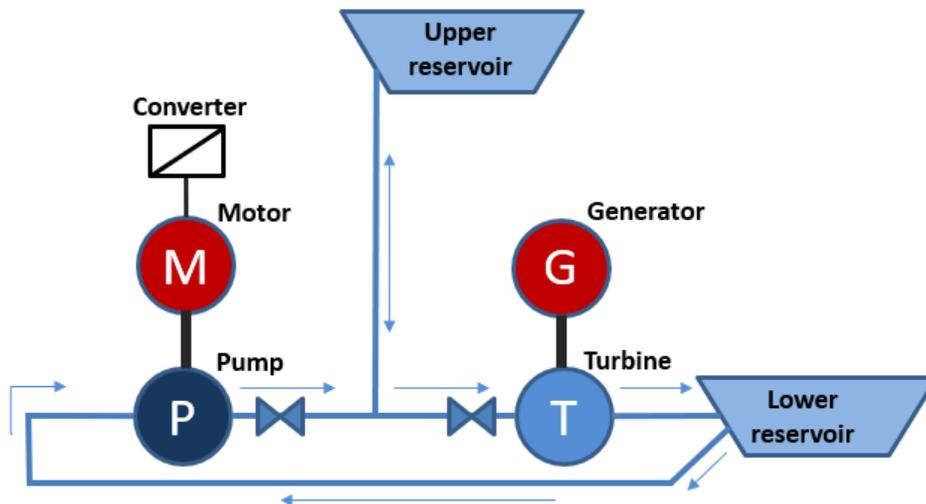
**Figure 2-6 Illustration of Quaternary PSH Design with Hydraulic Short Circuit**
