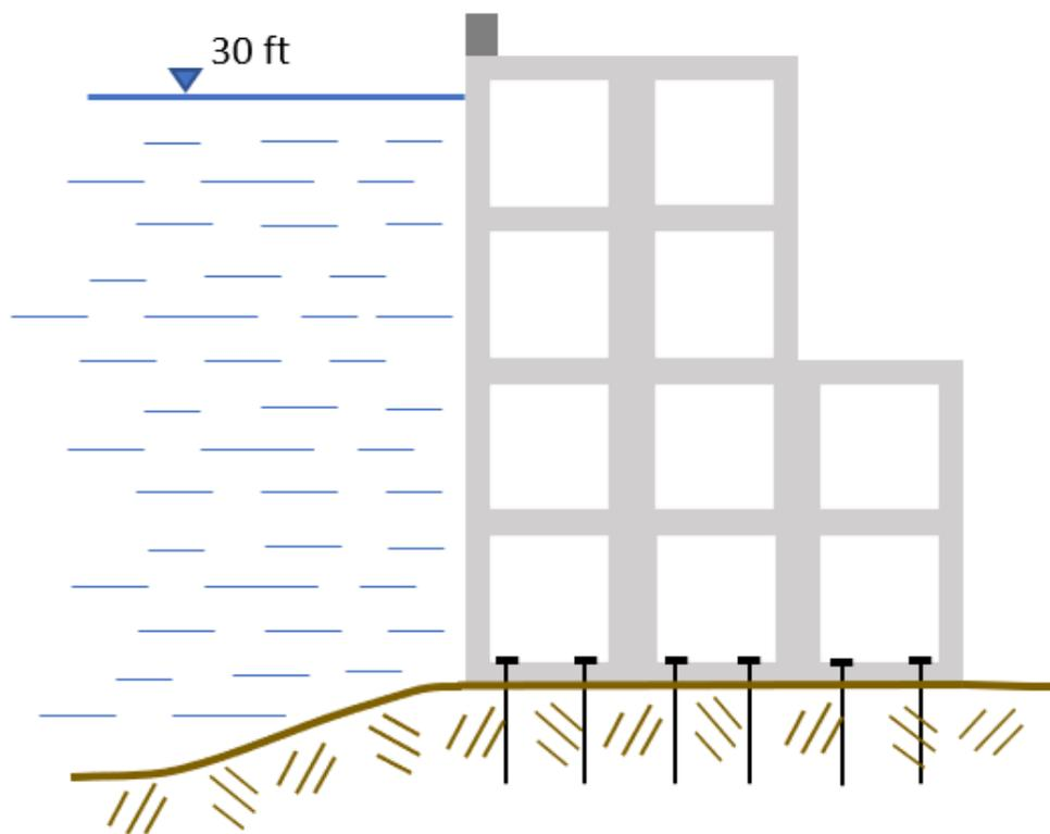
**Figure 5-6 Cross-section of a Modular Dam for 30-ft Reservoir**
