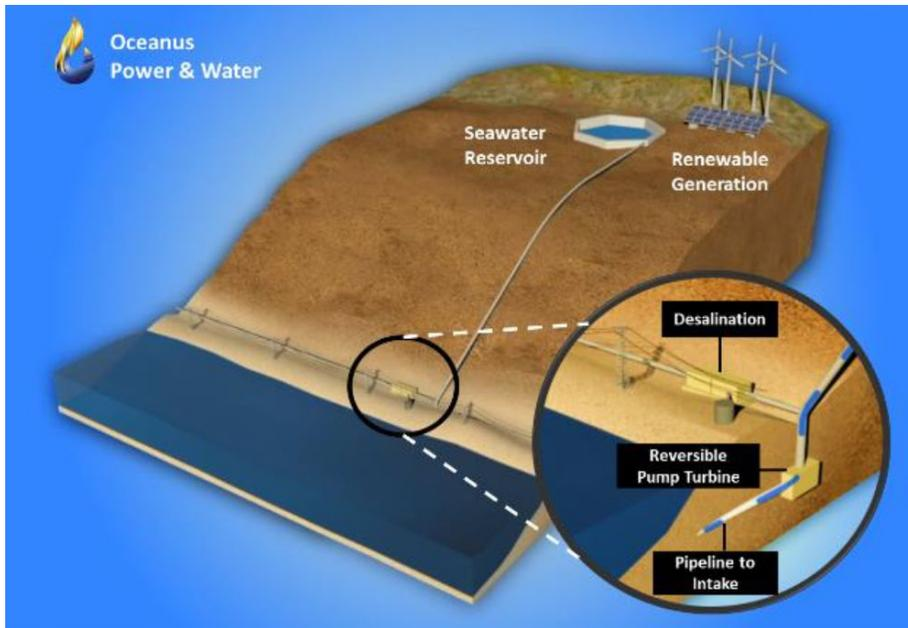
**Figure 3-9 Combined PSH and Desalination Plant (Source: Oceanus Power & Water)**
