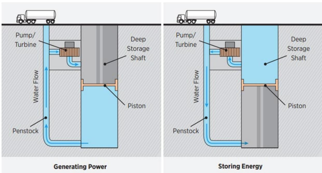
**Figure 4-3 Hydraulic PSH Concept (Source: DOE, 2016)**
