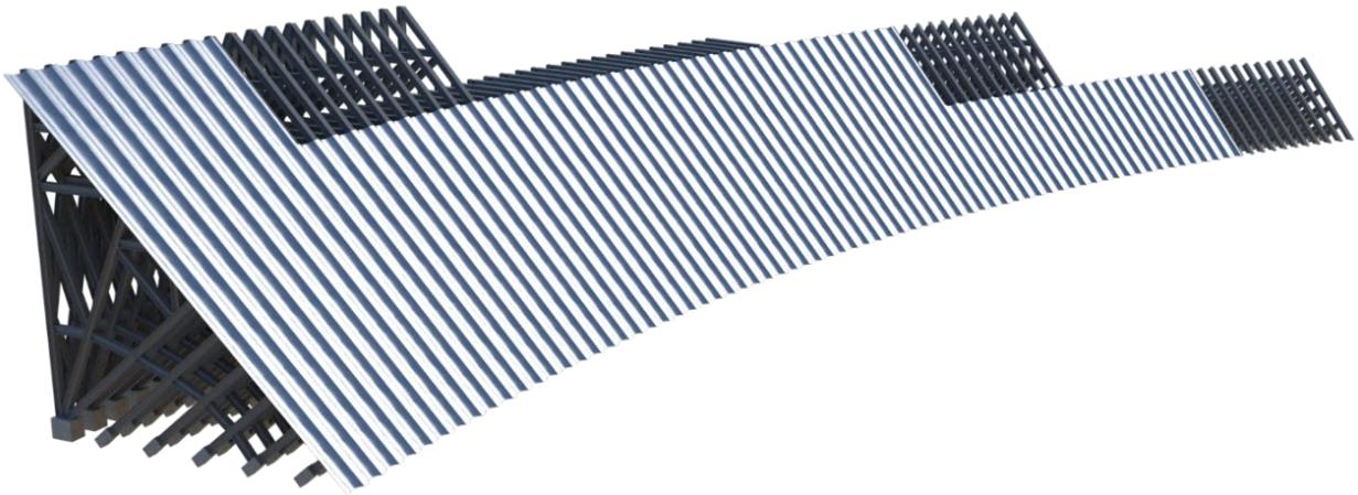
**Figure 5-9 Modular Assembly of a Steel Dam (Source: SwRI)**
