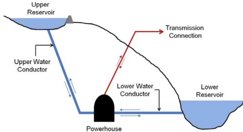
**Figure 2-1 Typical Configuration of a PSH Plant (Source: Koritarov et al., 2014)**
