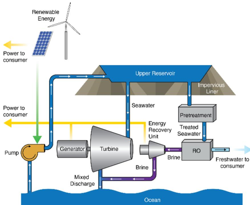
**Figure 3-10 IPHROCES Technology (Source: Oceanus Power & Water)**
