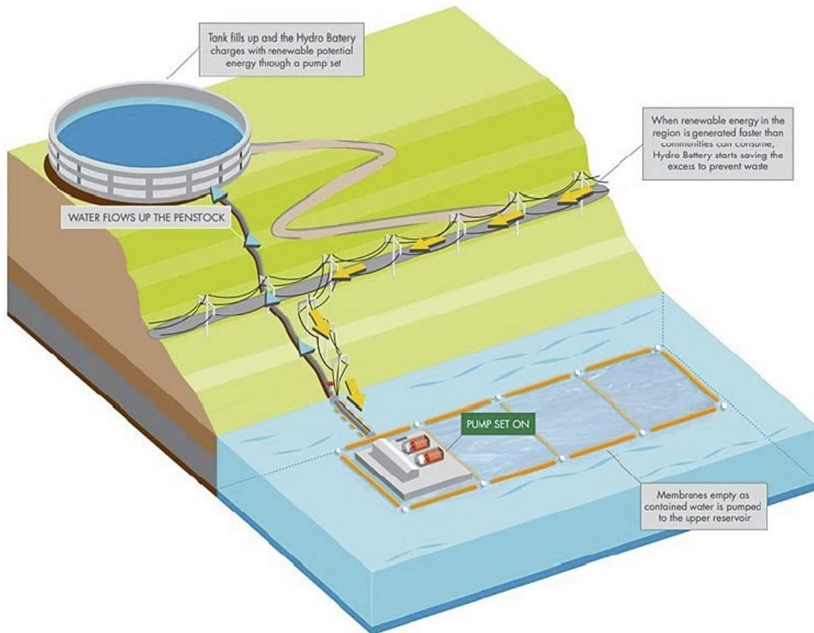
**Figure 3-2 SENA Hydro Battery Rendering (Source: Balducci et al., 2018)**
