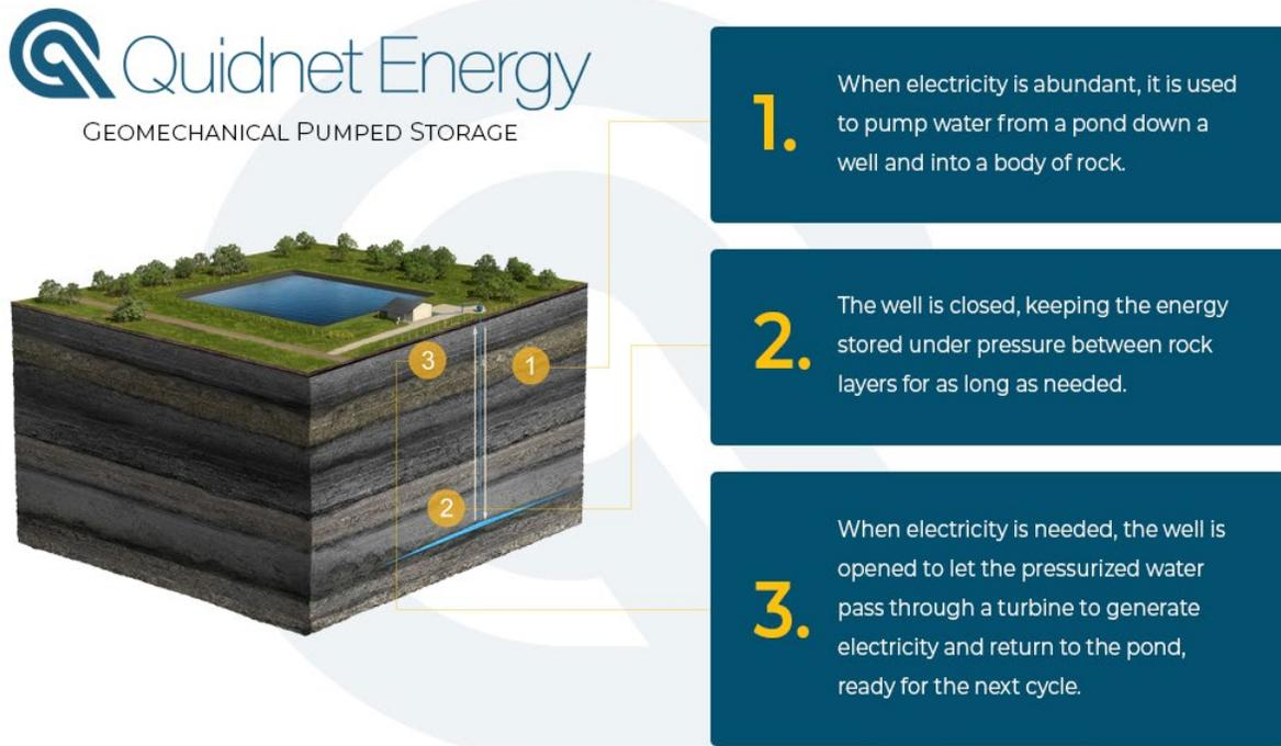
**Figure 3-5 Geomechanical PSH Technology (Source: Quidnet)**
