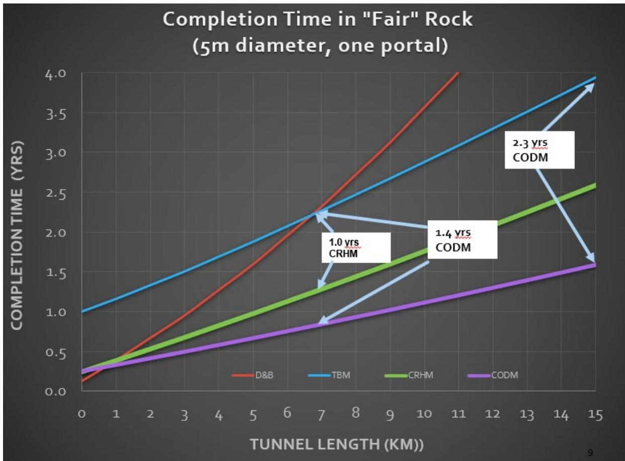
**Figure 5-5 Tunnel Completion Times for Different Excavation Methods as Function of Tunnel Length (Source: Kinetic Power, LLC)**
