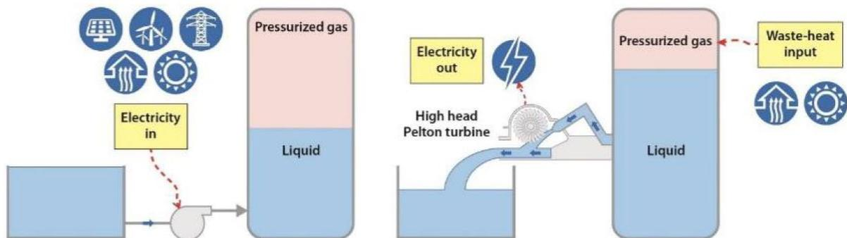
**Figure 3-16 GLIDES Pumping and Generating Cycles (Source: Abu-Heiba, 2019)**
