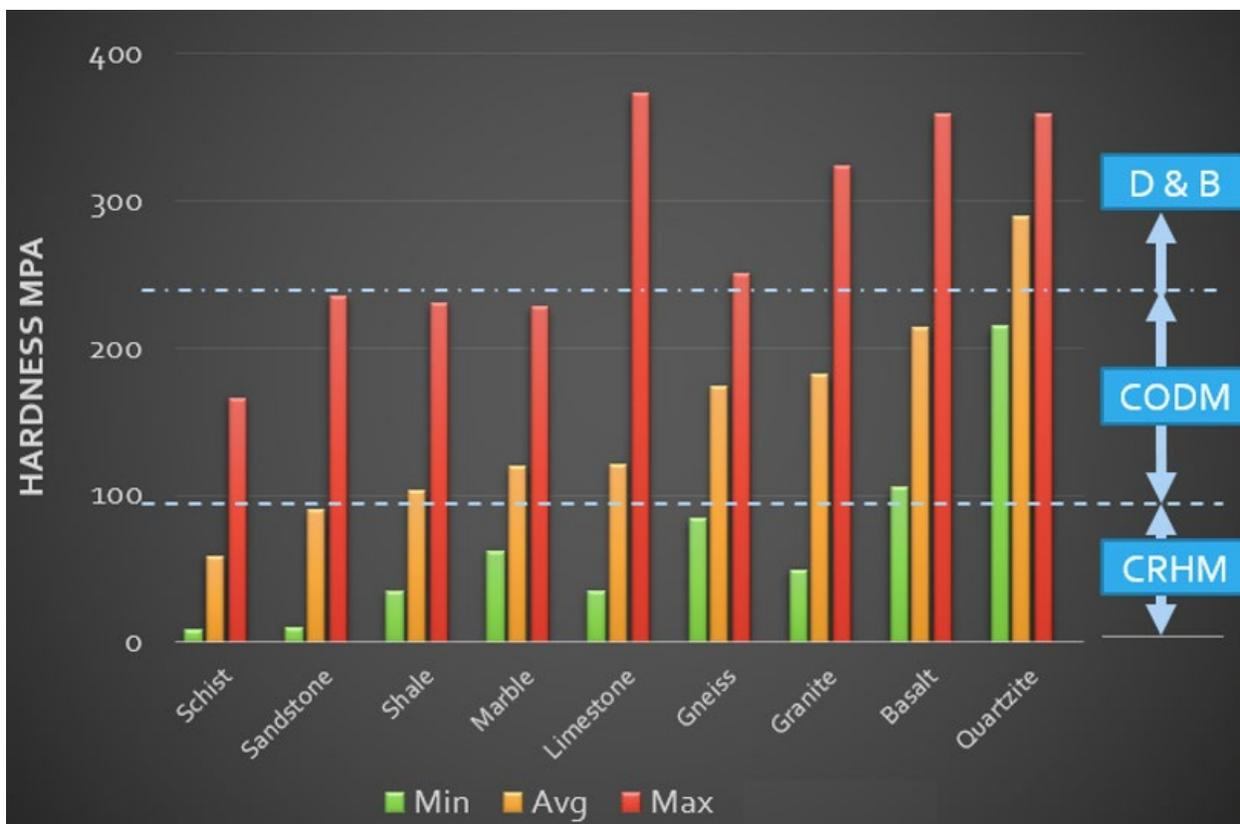
**Figure 5-4 Applicable Excavation Process for Rock Hardness (Source: Kinetic Power, LLC)**
