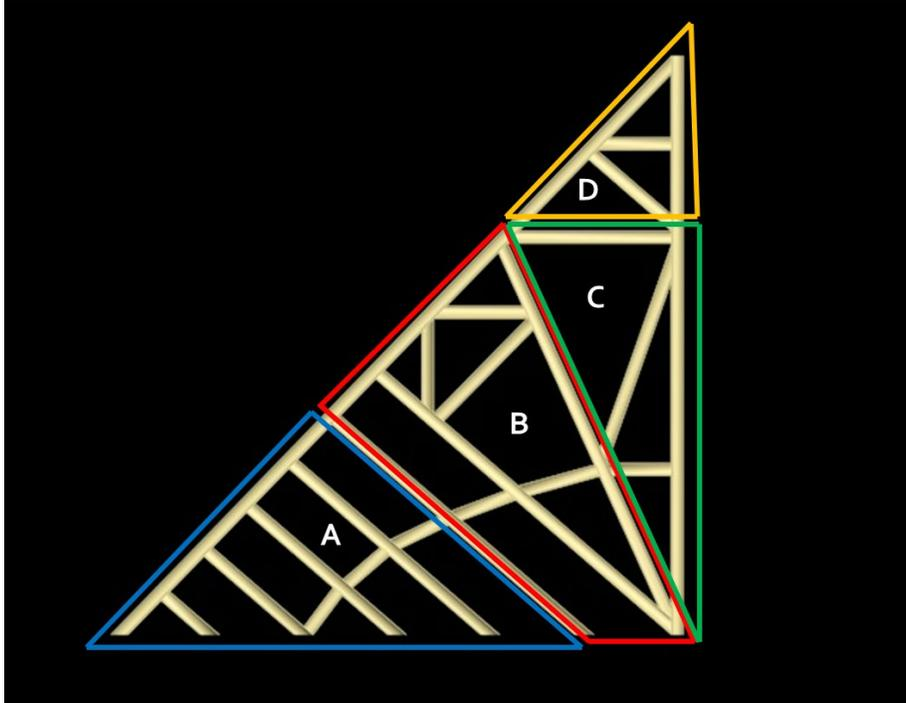
**Figure 5-8 Steel Frame Design Consisting of Four Segments: A, B, C, and D (Source: SwRI)**
