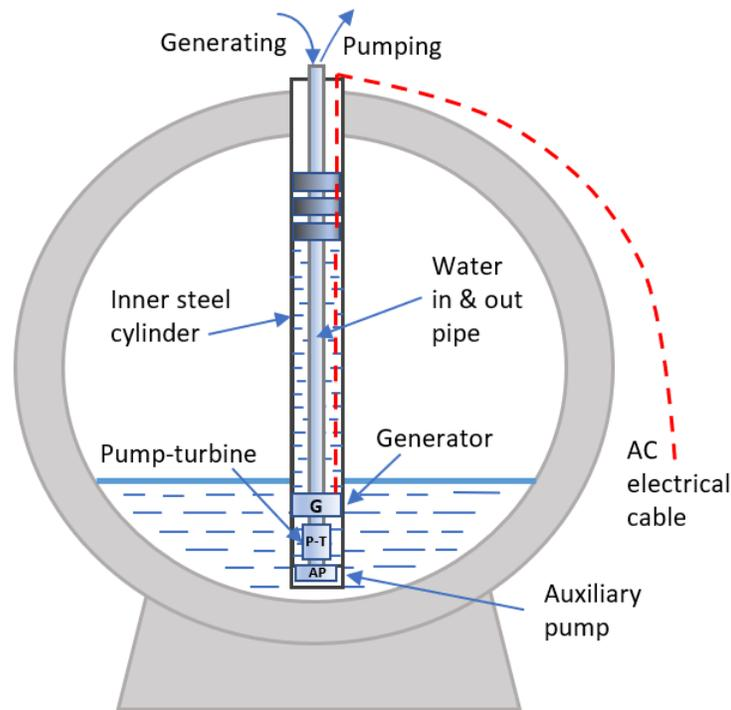
**Figure 4-1 Cross Section of the Submersed Sphere**
