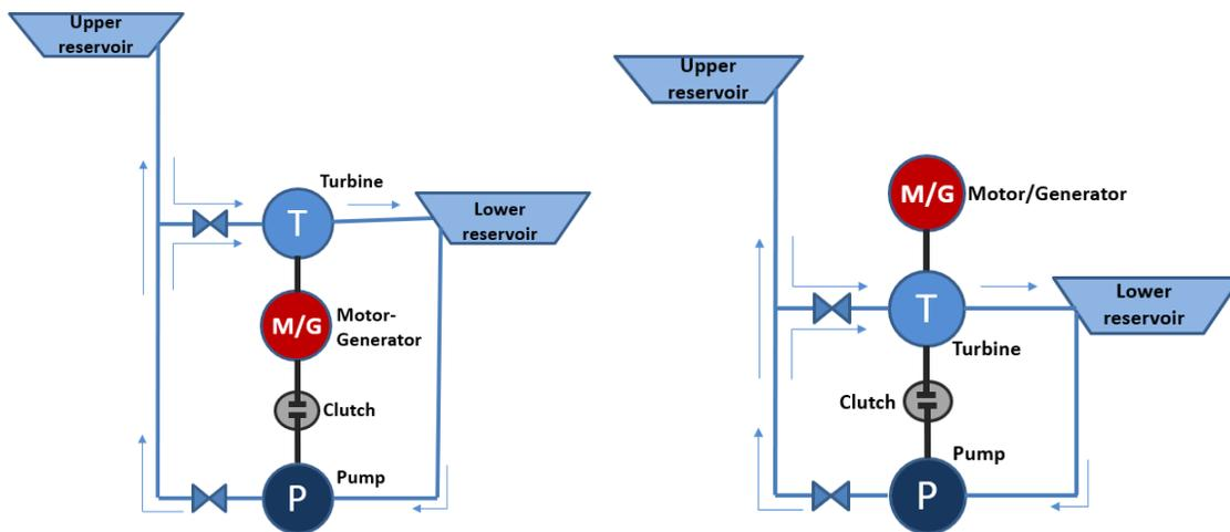
**Figure 2-5 Two Configurations of Ternary PSH Technologies with Hydraulic Bypass (Source: Koritarov et al., 2013b)**
