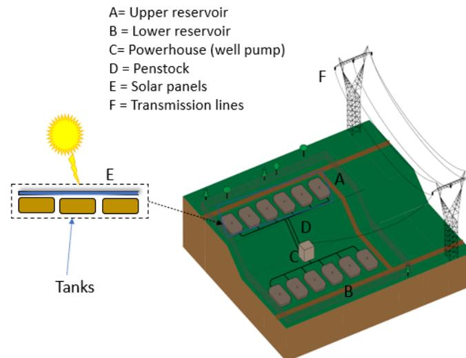
**Figure 3-13 Hybrid Modular Closed-Loop Scalable PSH Technology (Source: T. Eldredge and H. Medina from Liberty University)**
