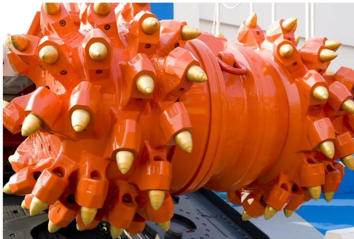
**Figure 5-3 Cutting Head of RHM (Photo credit: Shutterstock)**
