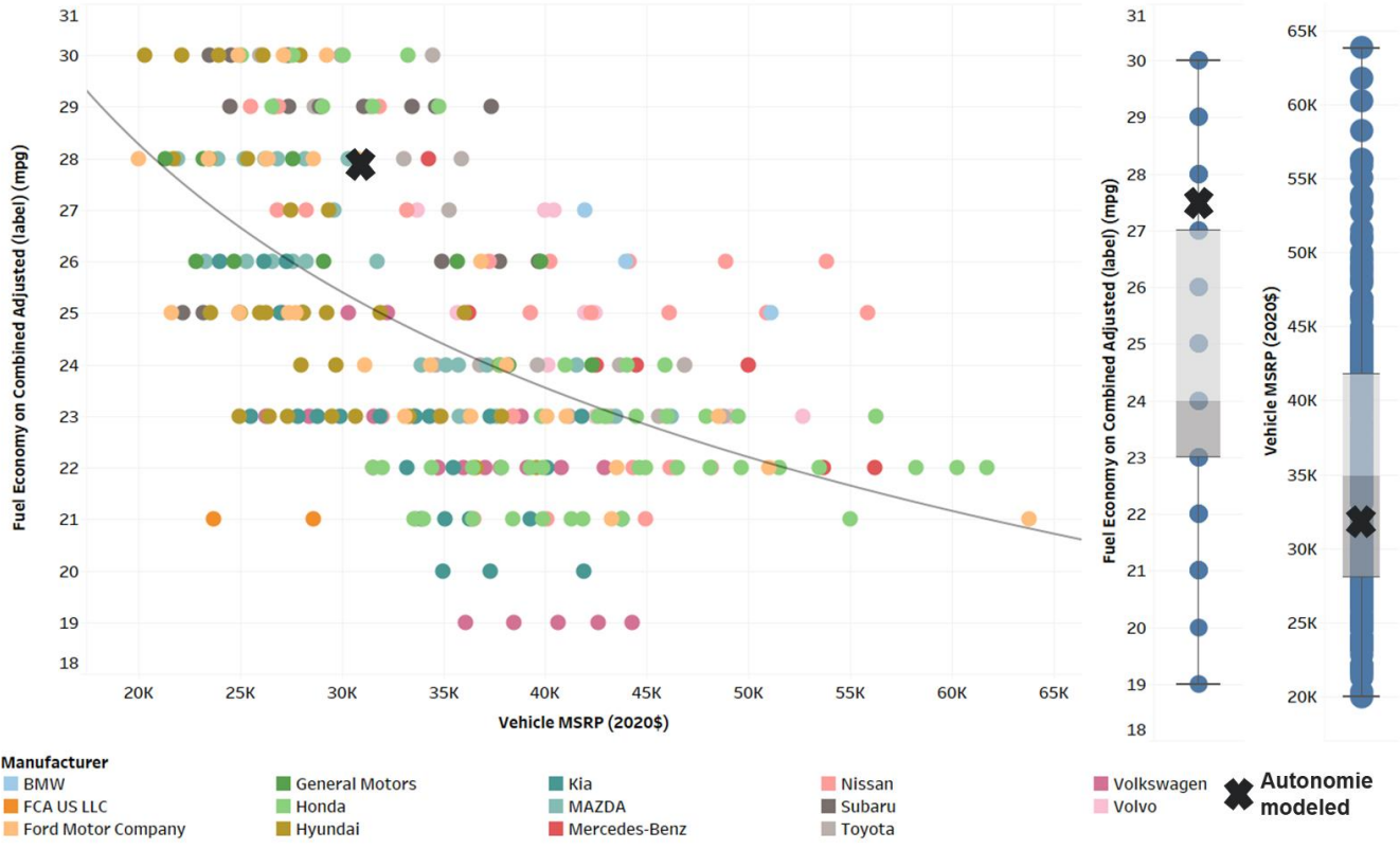
Figure A.2. Fuel Economy and Vehicle MSRP trend line of conventional small SUVs in the market from MY2020
