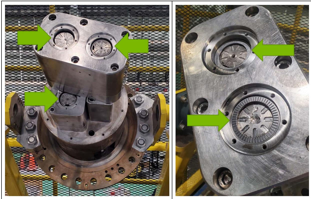
**Figure 20: The bottom of the GTA with no thrust bearing assemblies, indicated by green arrows (left). The bottom of the GTA with the thrust bearings included (right). The right-top arrow shows the bottom of a shaft with the thrust race in place. The right-bottom arrow shows the bottom of a shaft with the thrust race and bearing in place.**
