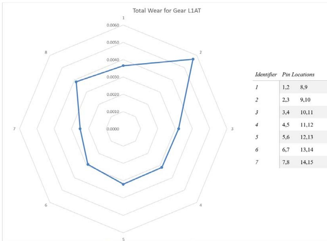
**Figure 16: Total wear measurements for gear L1AT made by taking the difference in over-pin dimensions [inches].**
