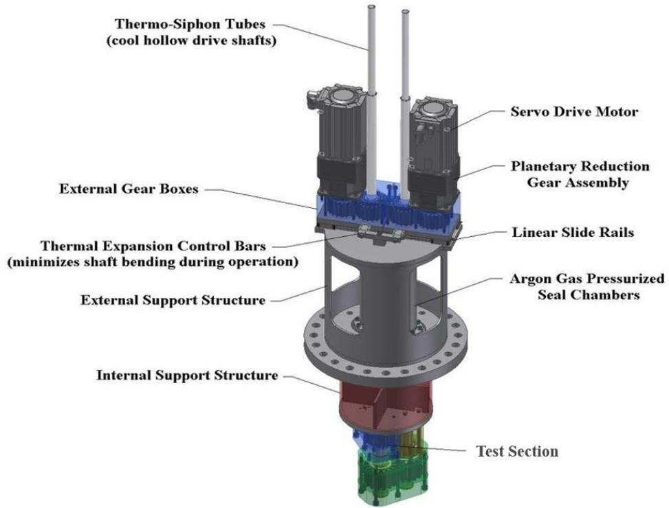
Figure 2: Overview of the Gear Test Assembly
