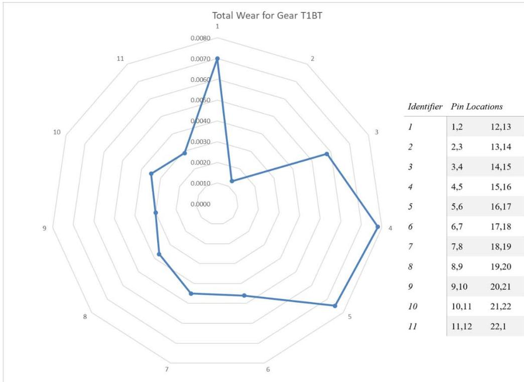
**Figure 18: Total wear measurements for gear T1BT made by taking the difference in over-pin dimensions [inches].**
