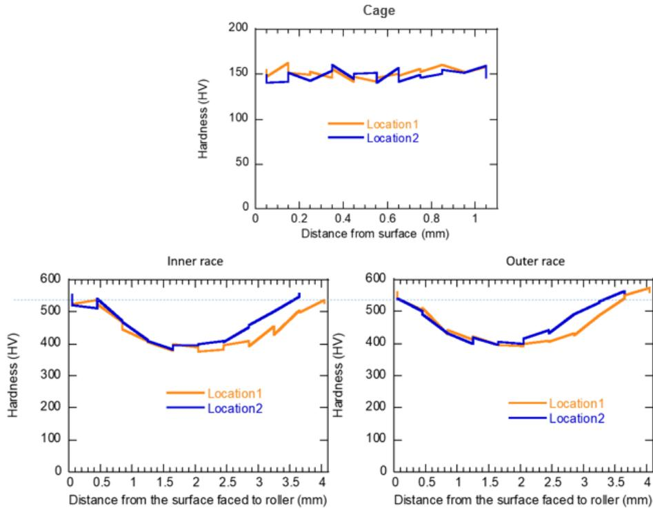
**Figure 5: Hardness data taken from the failed tapered roller bearing.**
