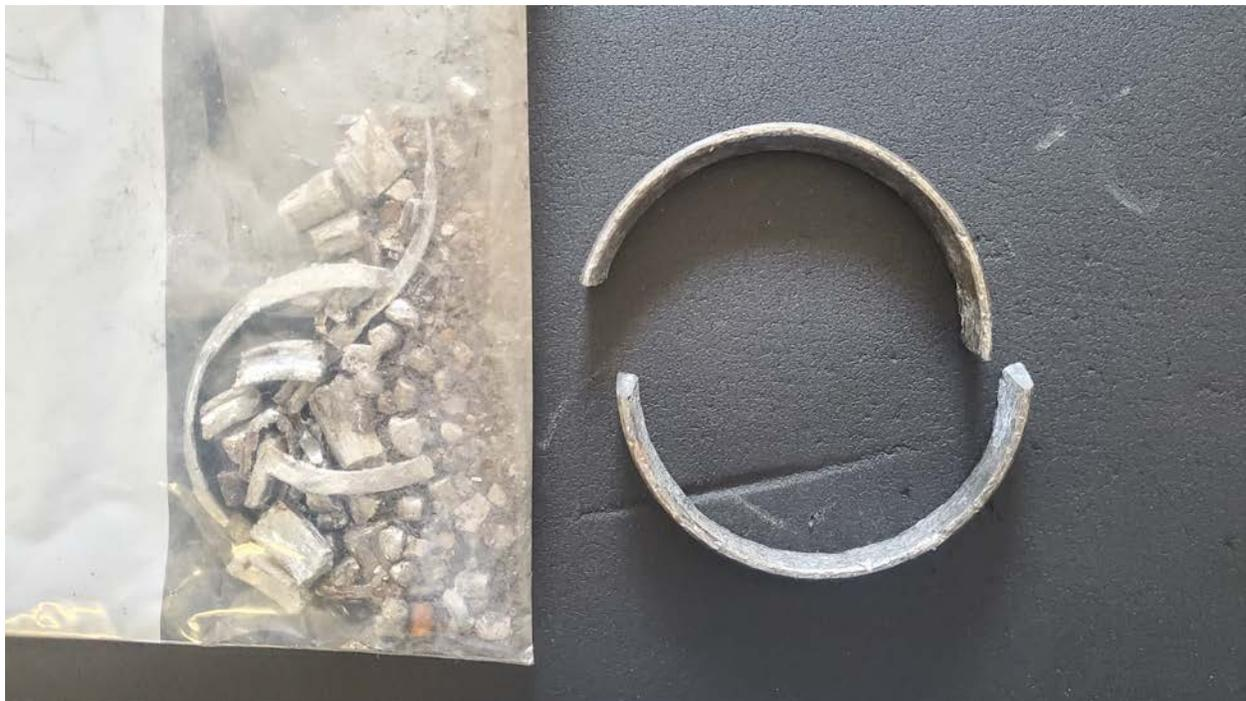
**Figure 10: Remains of the fragmented tapered roller bearing from Experimental Campaign #4.**
