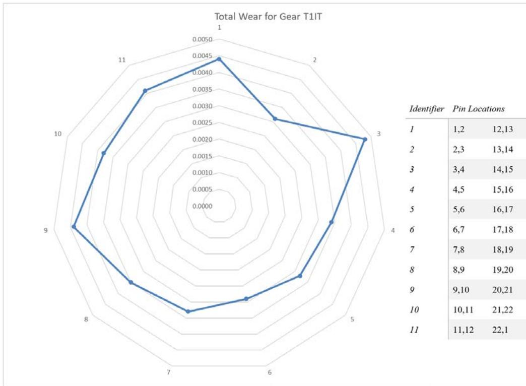
**Figure 19: Total wear measurements for gear T1IT made by taking the difference in over-pin dimensions [inches].**
