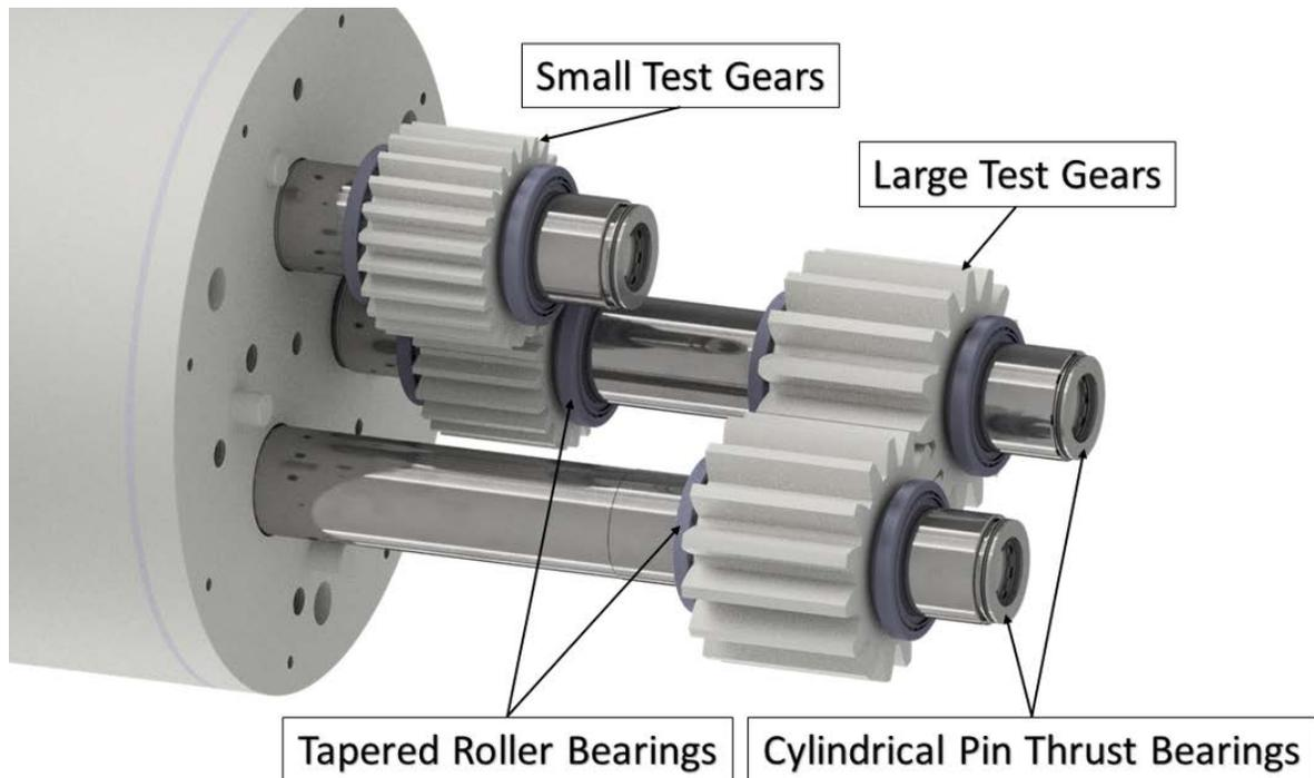
Figure 3: Overview of the submerged mechanical components tested in the GTA.
