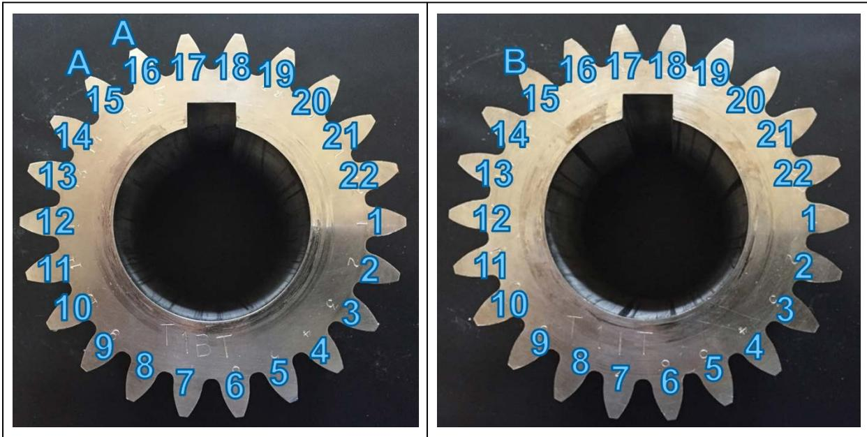
Figure 15: Pictures of the T1BT and T1IT gears with the gear teeth numbering labelled. The "A" and "B" notation are used to indicate where the gears mesh.
