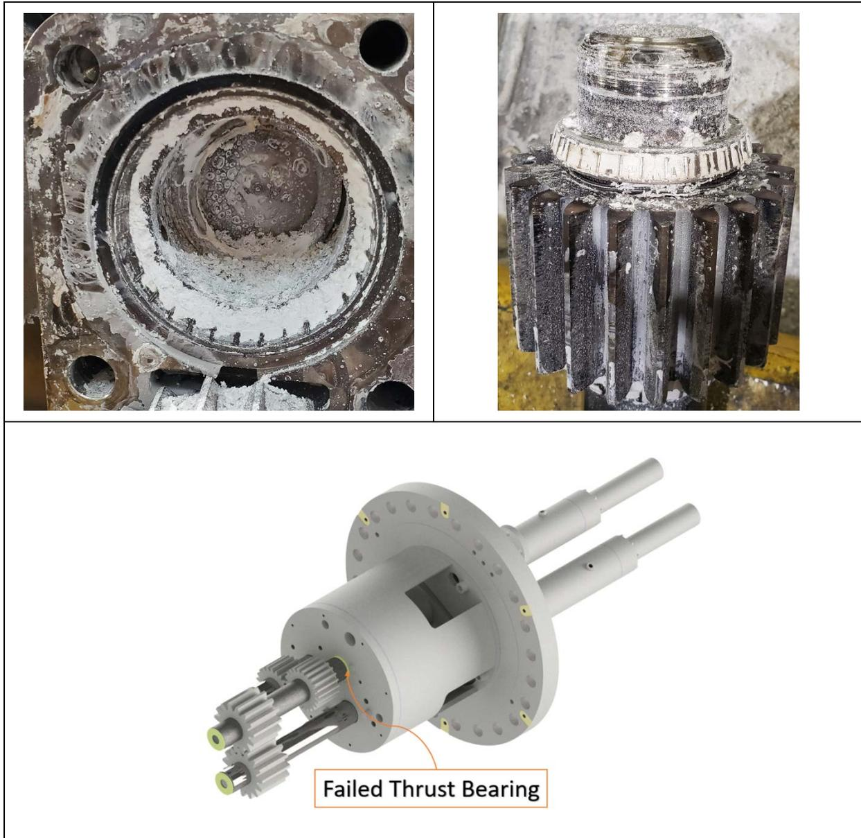
**Figure 9: Remains of failed thrust bearing in gearbox (left) and on shaft (right) from Experimental Campaign #3. Location of failed thrust bearing (bottom).**
