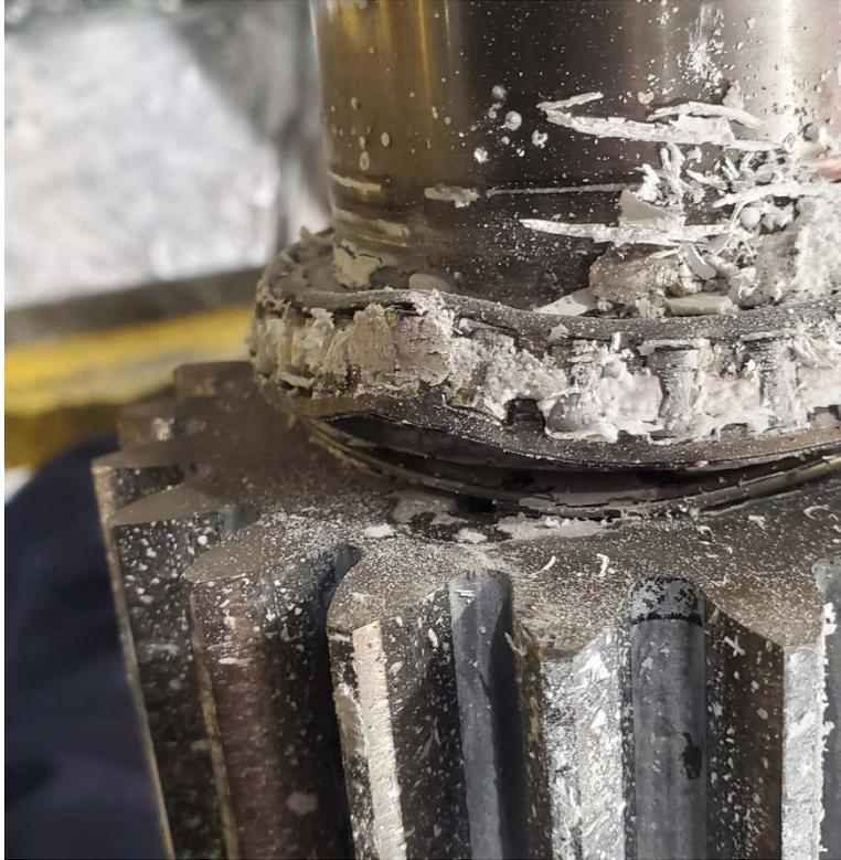
**Figure 11: Damaged tapered roller bearing from Experimental Campaign #4.**
