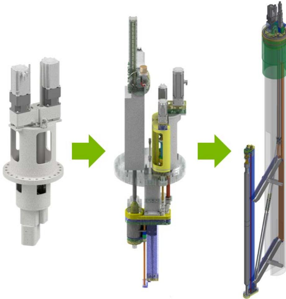
**Figure 1: Progressive experimental plan for the development of a compact fuel handling mechanism. Gear Test Assembly (left), Gripper Test Assembly (mid), Fuel Handling Mechanism (right)**
