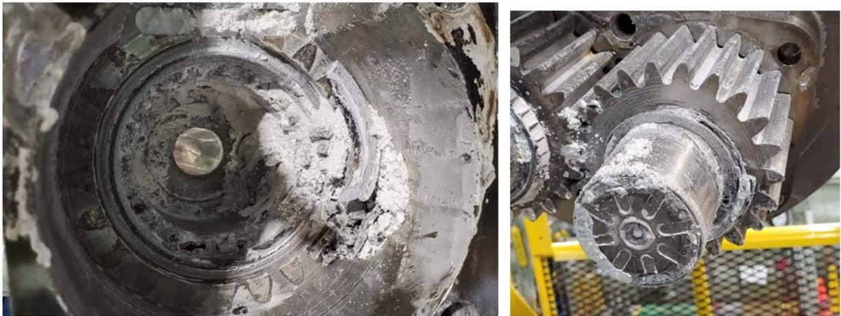
**Figure 7: Remains of bearing in gearbox (left) and on shaft (right).**
