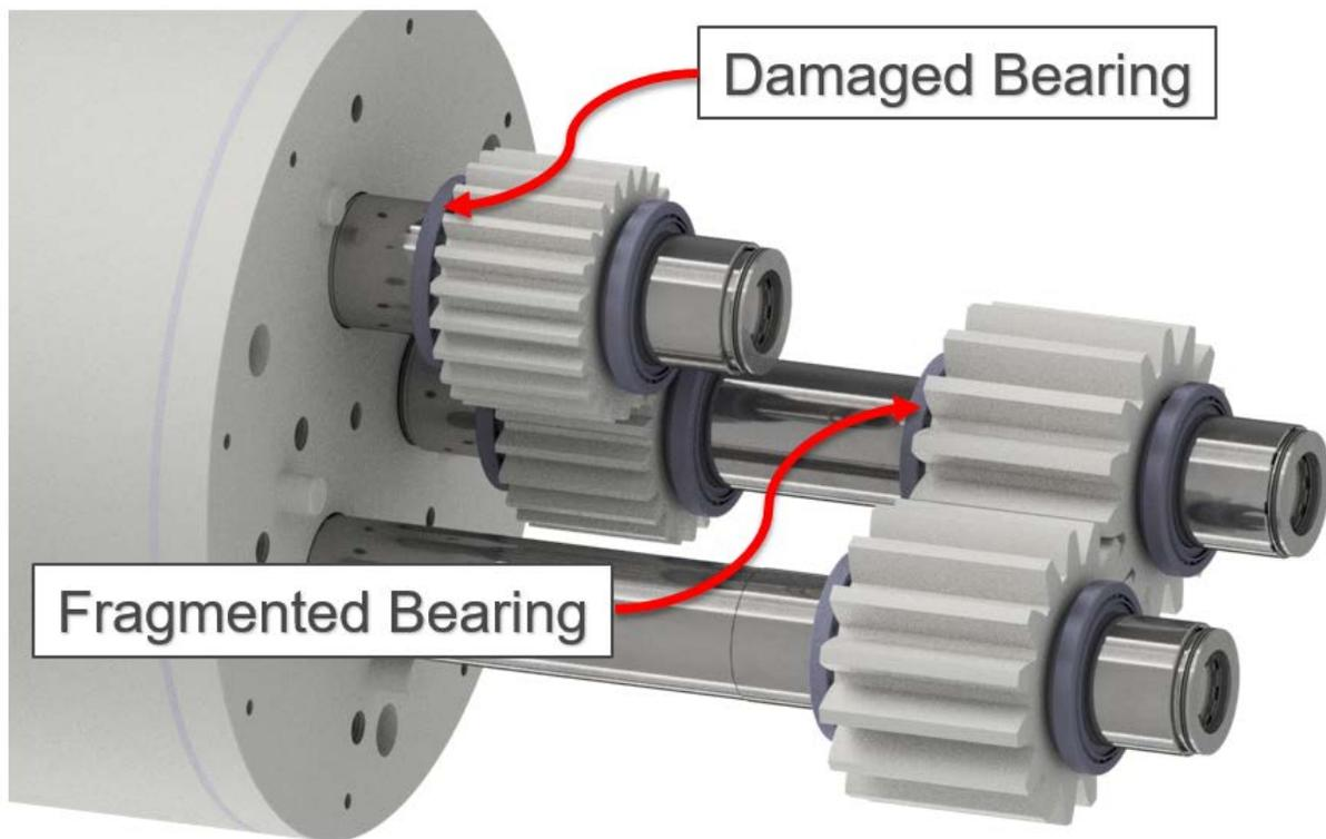
**Figure 12: Locations of bearing failures from Experimental Campaign #4.**
