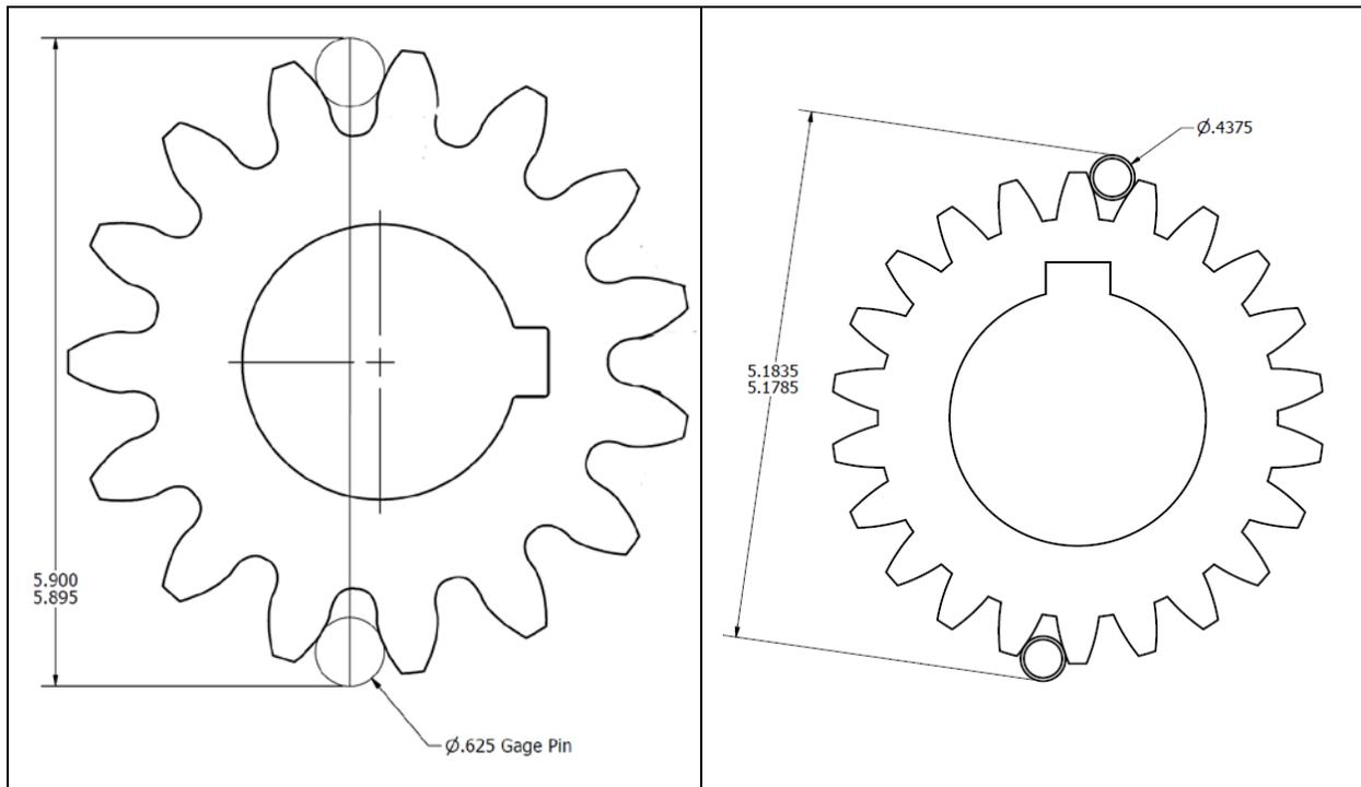
**Figure 13: Ideal over-pin dimensions for gears L1AT/L1IT (left) and T1BT/T1IT (right).**
