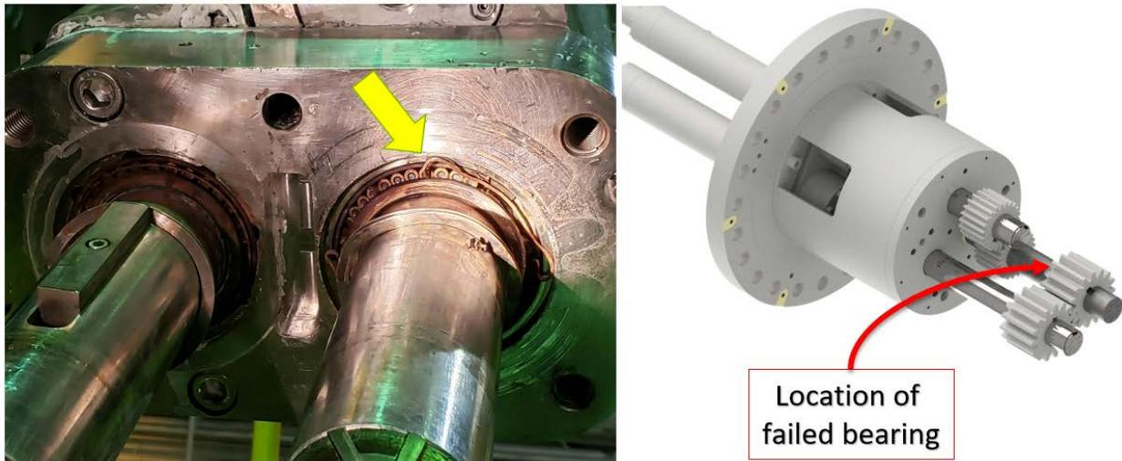
Figure 4: View of the tapered roller bearing that failed in Experimental Campaign #1.
