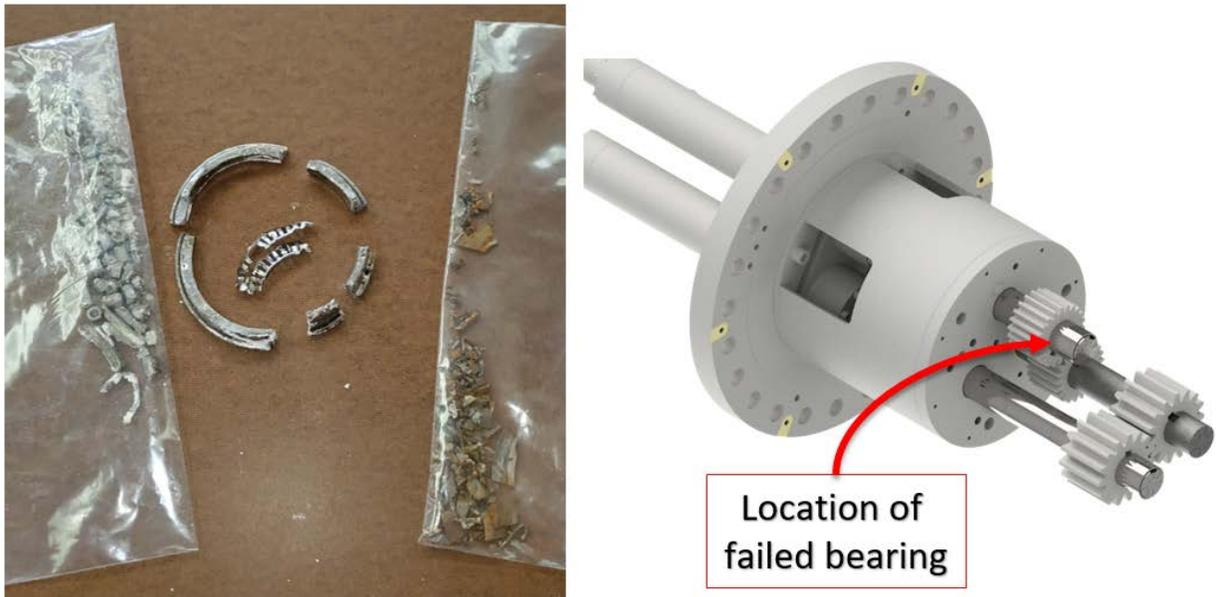
**Figure 6: Remains of failed tapered roller bearing (left) and location of failed bearing (right) from Experimental Campaign #2.**
