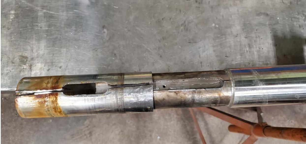
**Figure 8: Damaged shaft sleeve following Experimental Campaign #2.**
