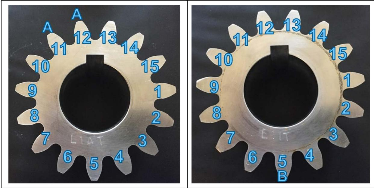
Figure 14: Pictures of the L1AT and L1IT gears with the gear teeth numbering labelled. The "A" and "B" notation are used to indicate where the gears mesh.
