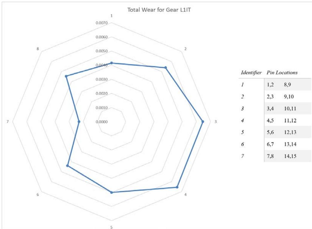
**Figure 17: Total wear measurements for gear L1IT made by taking the difference in over-pin dimensions [inches].**
