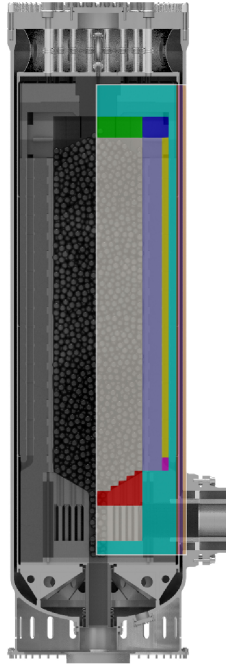
Figure 2.1: Schematic of the core of the generic pebble bed reactor ( Stewart et al. (2021) ).
