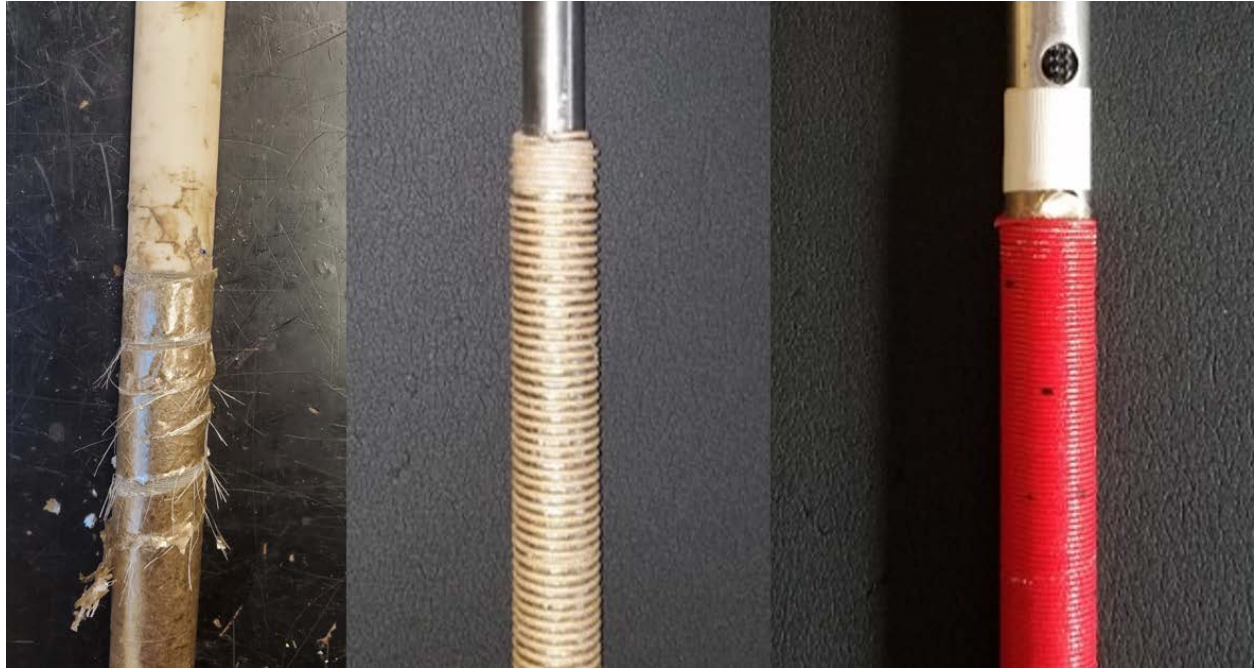
Figure 6: Progression of MILS prototyping with the ceramic-nickel prototype (left), NCC-mica prototype (mid), and constantan-fiberglass prototype (right) .
