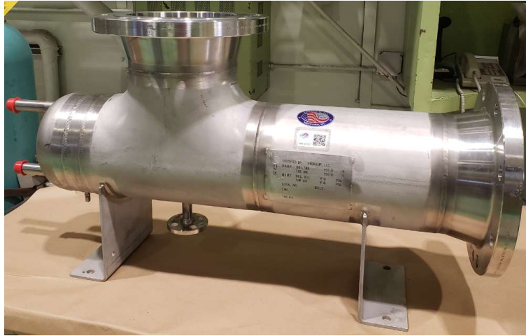
Figure 34: THETA secondary loop sodium-to-air heat exchanger
