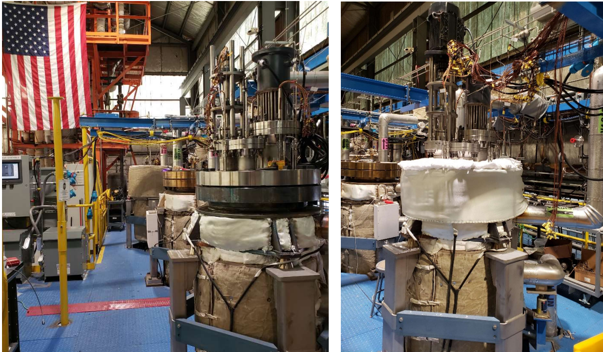
Figure 3: THETA installed in METL test vessel #4. Left: uninsulated without pump motor installed. Right: insulated with pump motor installed.
