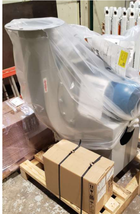
Figure 40: Photo of the high-pressure air blow for the air-to-sodium heat exchanger. (PN: Cincinnati Fan HP-8D19)
