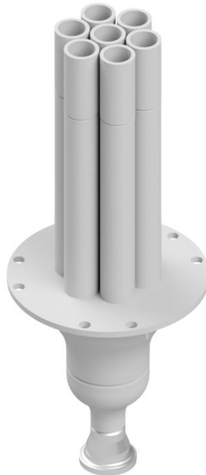
Figure 8 – Updated Pseudo-Scaled Test Section with a new 2-inch pitch and resized flow conditioners.
