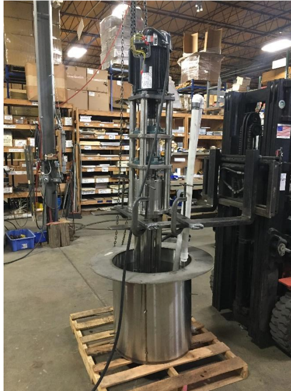
Figure 18 – Completed pump setup at vendor for initial validation testing.
