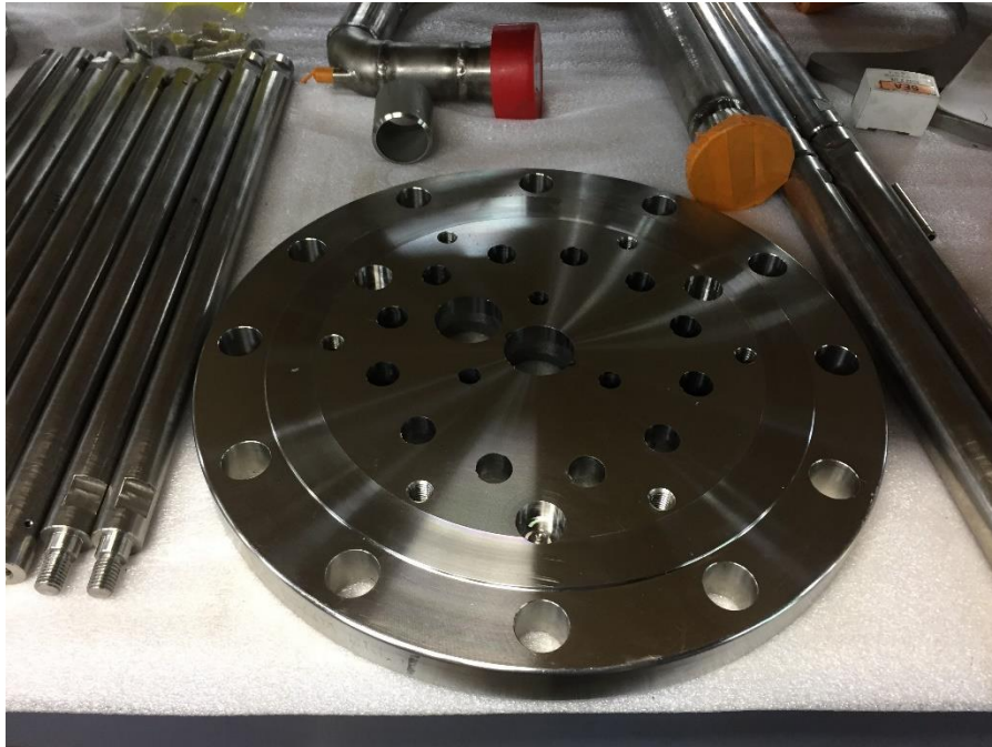
Figure 22 – Bottom view of the Test Section Flange. Note that this view is prior to the fittings being welded.
