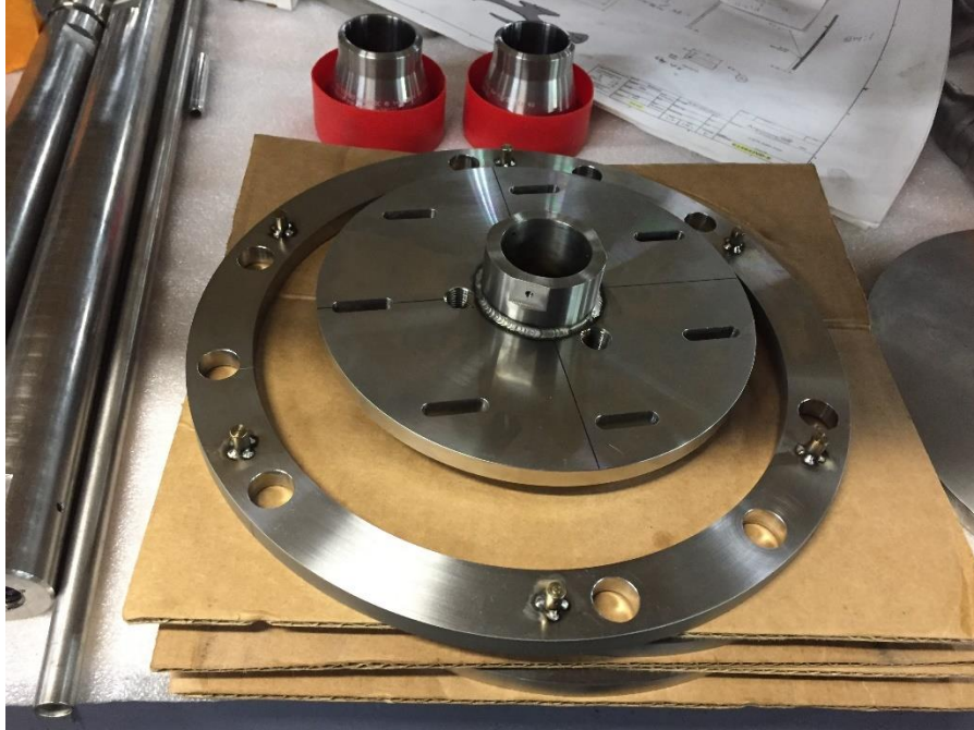
Figure 23 – Rabbit Tube alignment (center) and Test Section Support Ring (outer).
