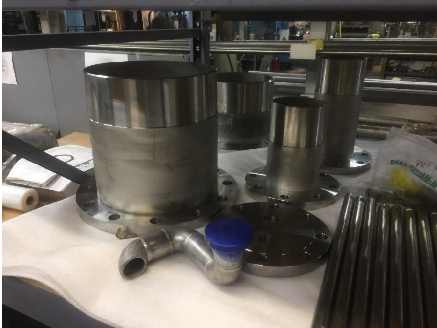
Figure 25 – View of the four main flange thermal stand-offs. On the left is the test section, in the center-back is the pump, in the center front is the cooler, and on the right is the heater.
