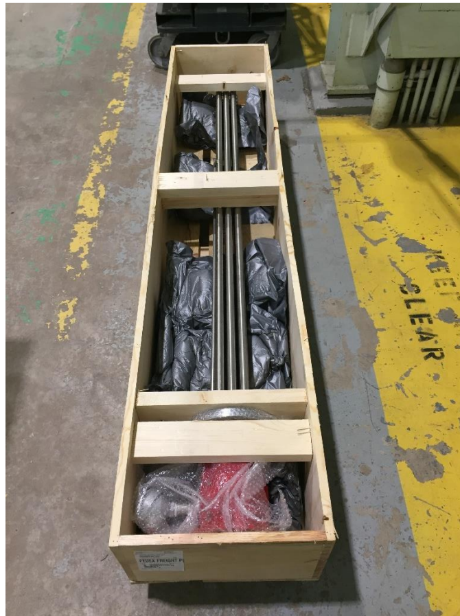
Figure 19 – Crated heater unit after arrival. The unit passed the resistance testing on the heating elements. However, MTR, dye-pen testing, and hydrostatic testing documentation were not included and were later found to be omitted during construction. Therefore, the unit was rejected and returned to the vendor for the required testing.
