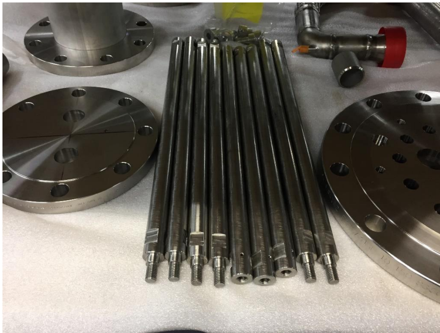
Figure 24 – Test Section Support Struts.
