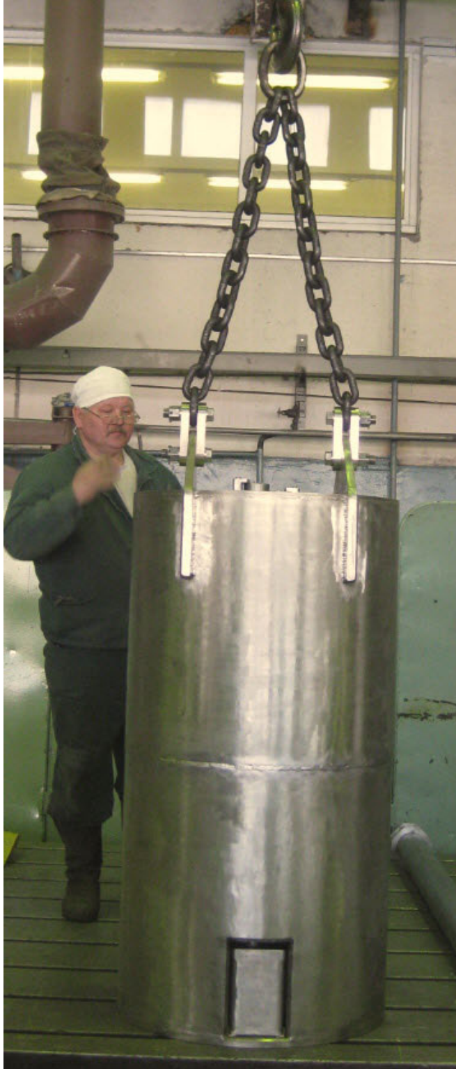
Figure VI.4.1.1. The fuel transfer cask shown during the manufacturing process.
