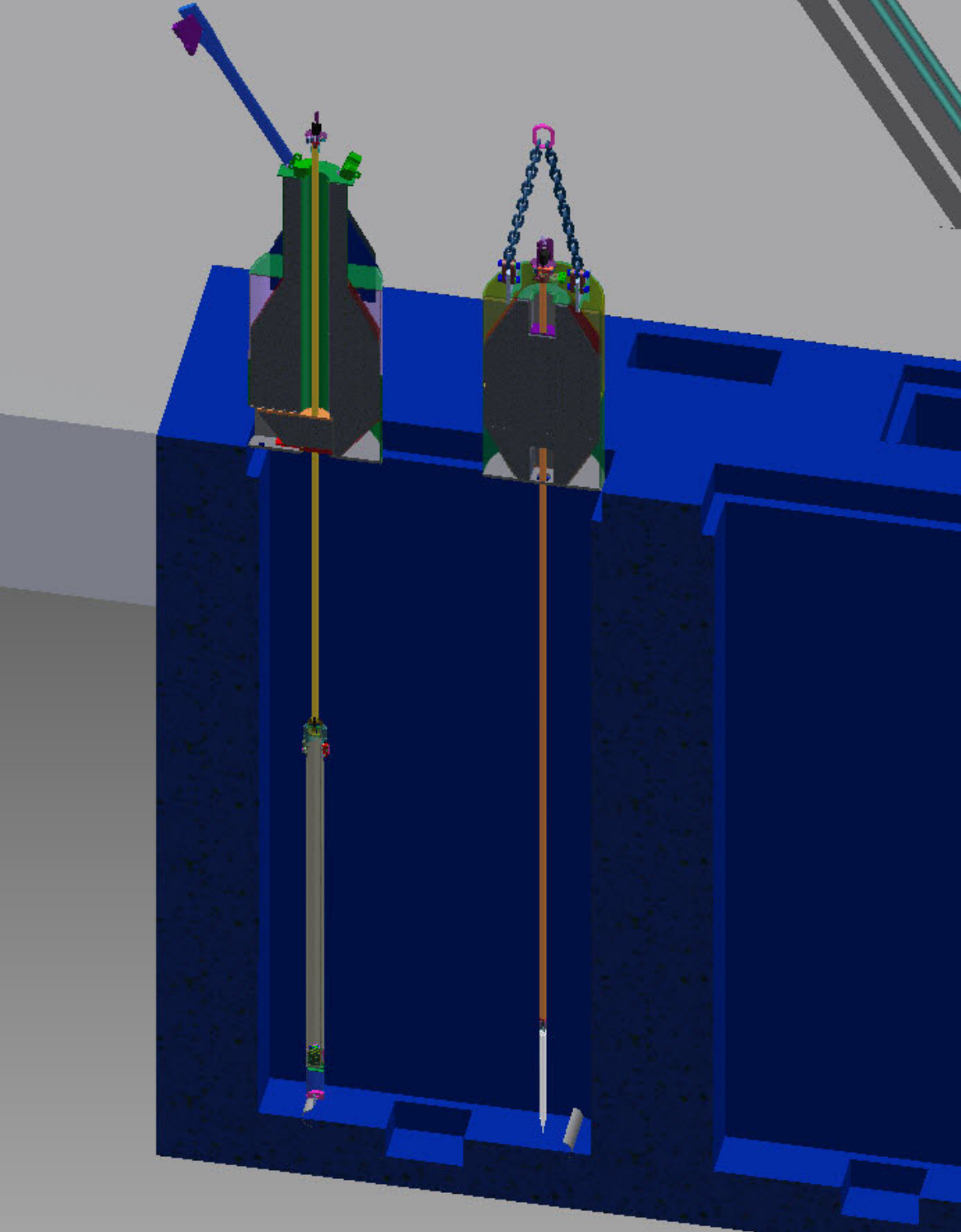
Figure VI.4.2.6. Cross section of the spent fuel pool showing both the target cask and the fuel cask in simulated loading condition. Long dipsticks are used to place/retrieve assemblies in the spent fuel pool.
