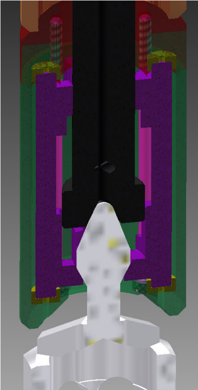
Figure VI.4.1.8. Section view of the fuel dipstick showing the rotating dog jaws and a fuel assembly.
