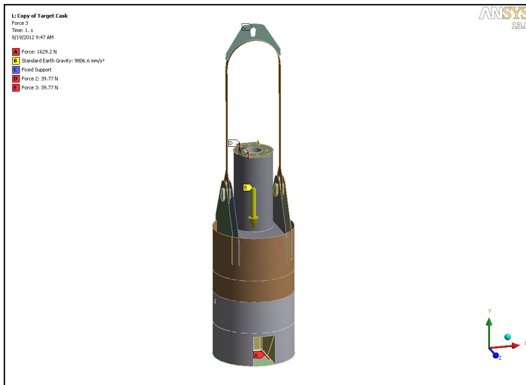
Figure VI.3.8.1. The target cask loads and the boundary conditions
