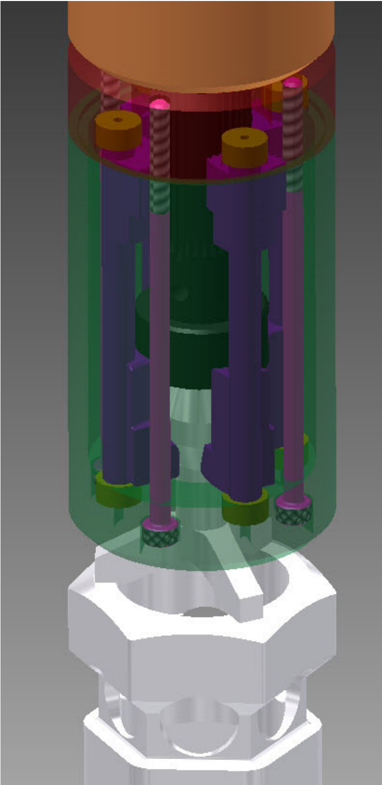
Figure VI.4.1.7. Bottom of the fuel dipstick shown engaged with a fuel assembly.
