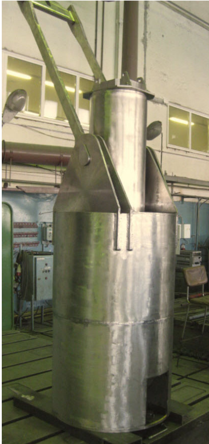
Figure VI.4.2.1. The target transfer cask, shown during the manufacture.
