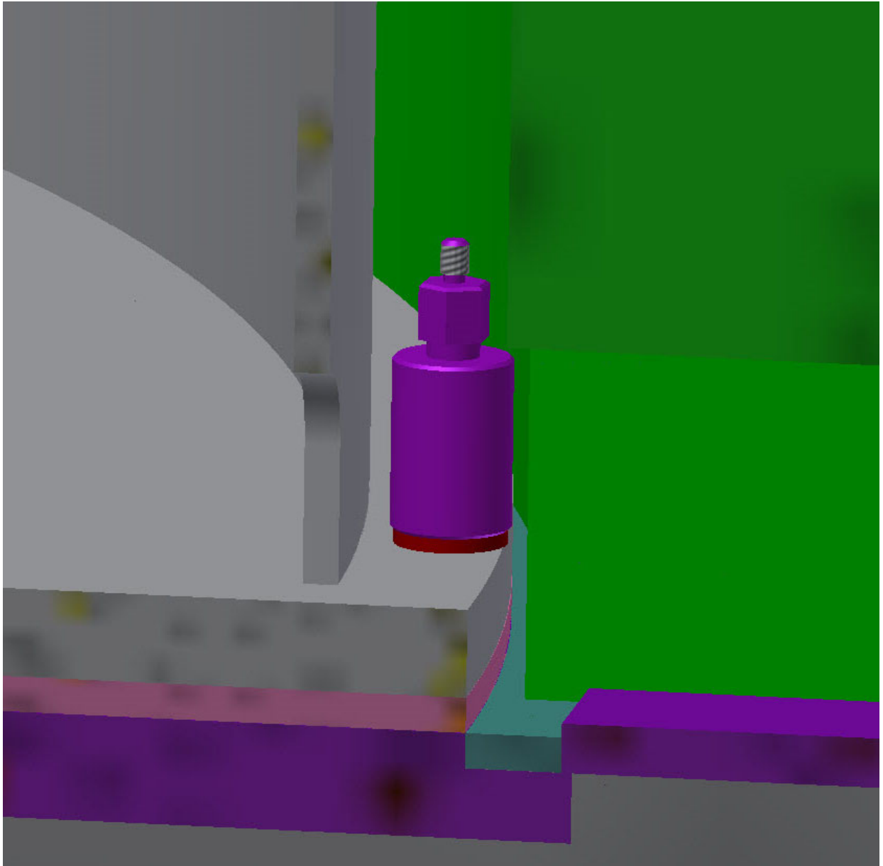
Figure III.7.7. Section view of the SCA tank flange shows one of the tank attachment nuts, the dielectric spacer plate under the gray tank, and the foundation plate. The biological shielding is the green region to the right of the nut and accompanying sleeve.
