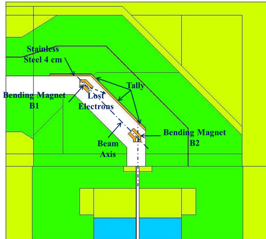
Figure IV.3.3. MCNPX model for calculating the energy deposition in the heavy concrete shield due to the electron losses from B1 bending magnet
