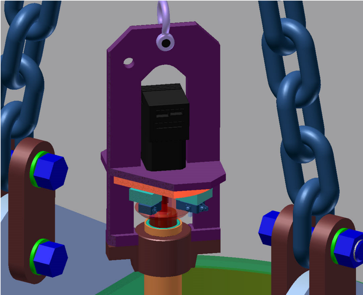
Figure VI.4.1.6. Top of fuel dipstick showing the step motor and the micro-switches.
