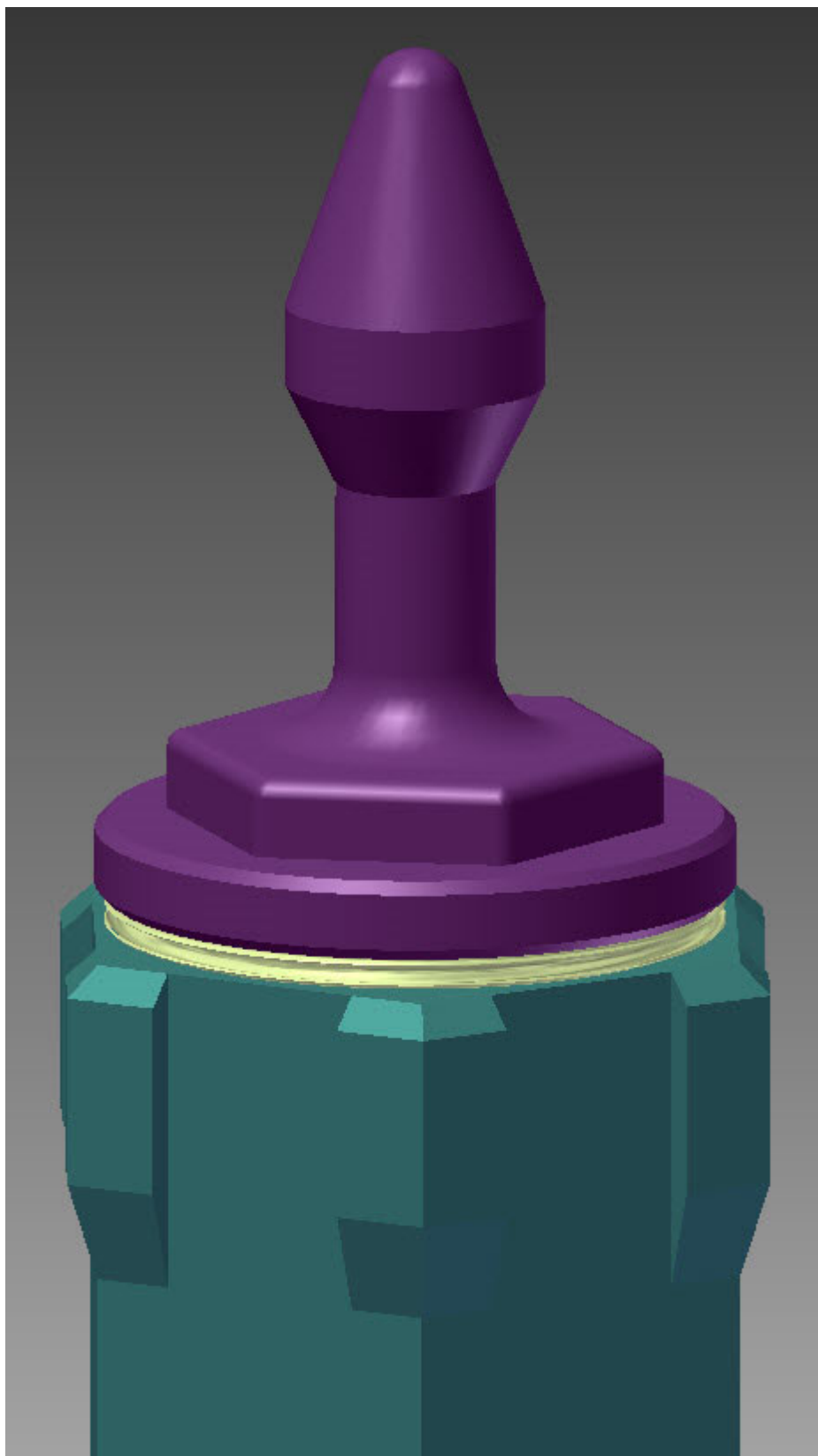
Figure VIII.4.2.1. Top of sample cassette, showing lifting knob and seal.
