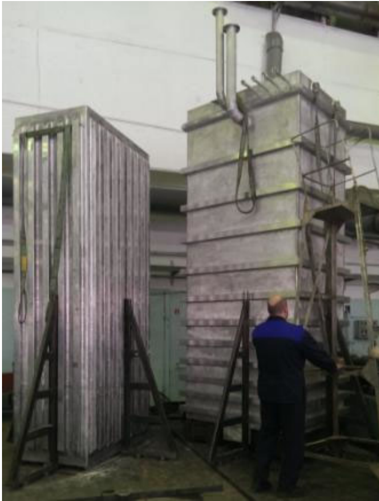
Figure V.4.1.9.23. The inner tank on the right and outer tank on the left of the fabricated spent fuel storage pool
