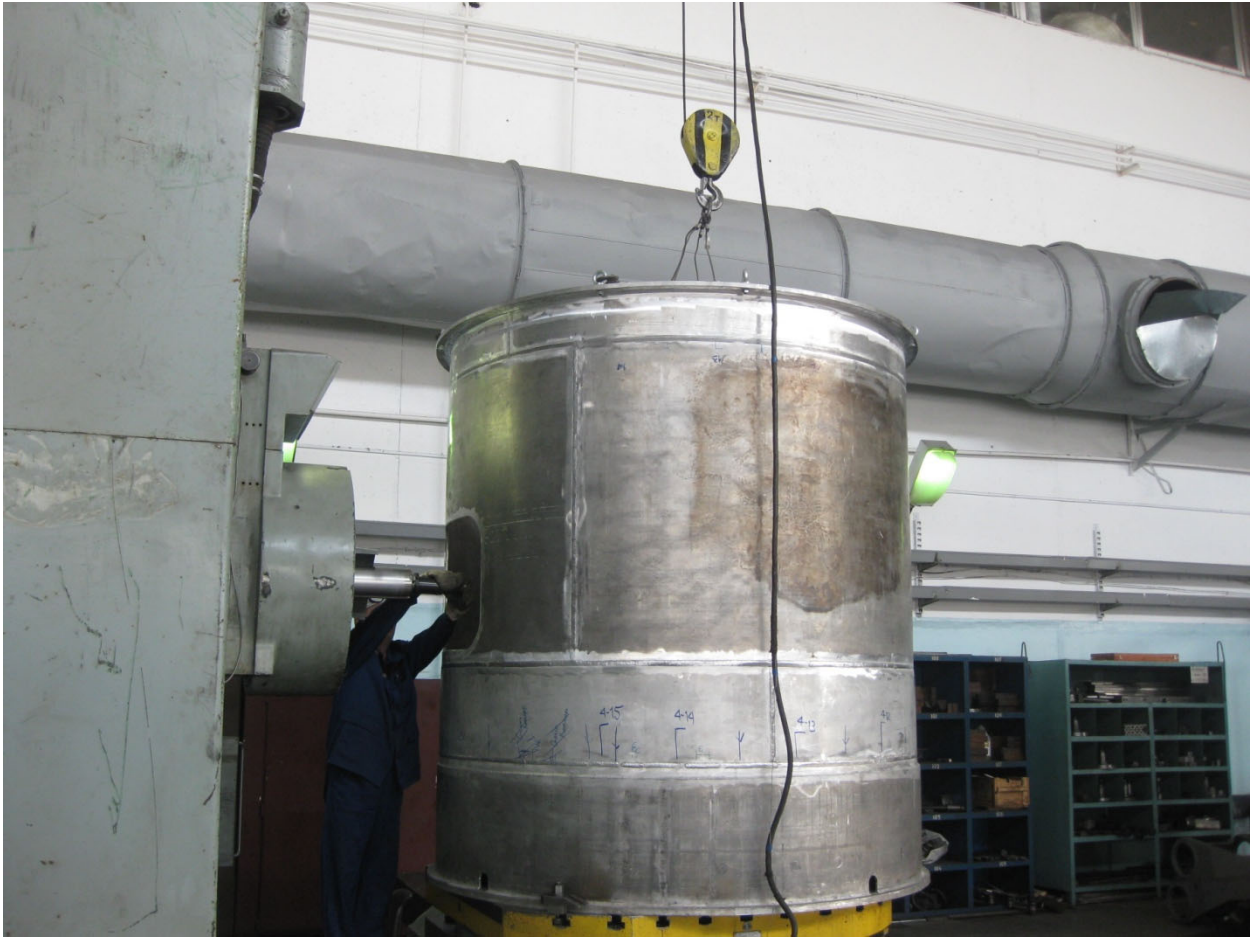
Figure III.7.6. SCA tank shown during the manufacturing process, the bottom of the cold neutron source well (left side of the tank) is being machined in this photo.
