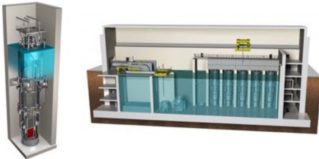
Figure A-3 VOYGR™ nuclear power module (left) and arrangement in reactor building (right) (Courtesy of NuScale Power)
