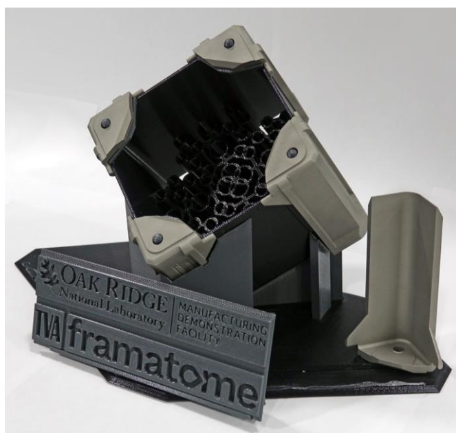
Figure 5. The fuel assembly channel fasteners printed at ORNL using the additive manufacturing technique and installed on ATRIUM 10XM fuel assemblies at Framatome’s nuclear fuel manufacturing facility in Richland, Washington.
