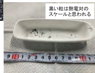
After test (1000°C steam environment)
