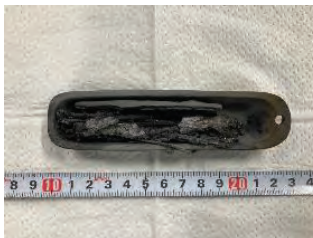
After test (1000°C H2 gas environment)
