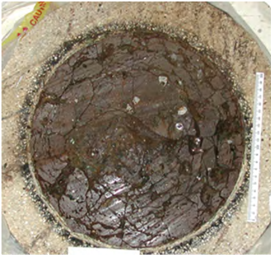
Figure D-8. Corium slab (30 cm outside diameter, 5 cm thick) sectioned from SSWICS post-test corium ingot (left); loading device for measurement of crust tensile strength (right)
