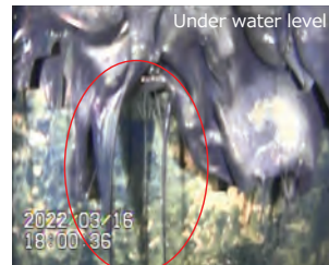
Solidified streams under water level
