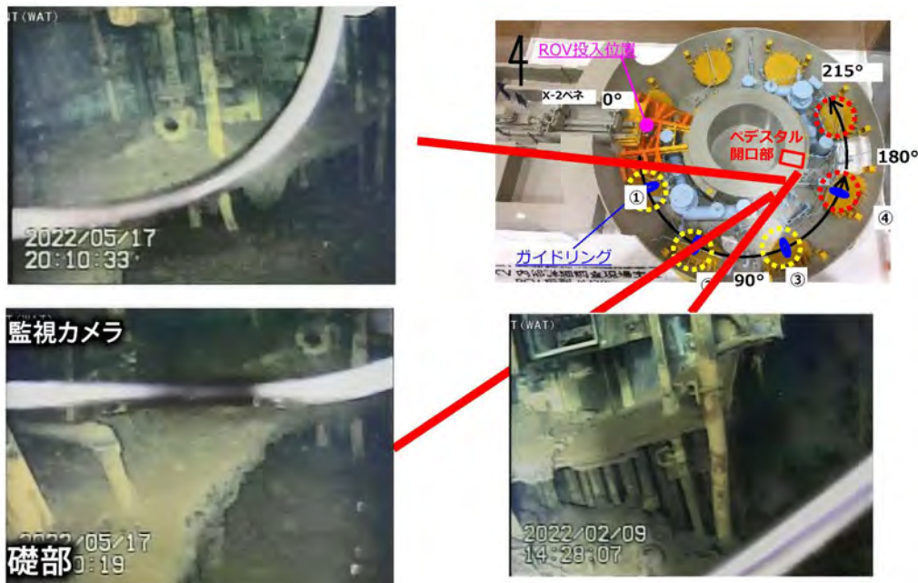
Figure D-1. Debris state in drywell near pedestal doorway; upper surface of the crust material is at ~ 1 meter elevation (Courtesy of TEPCO Holdings, [112])
