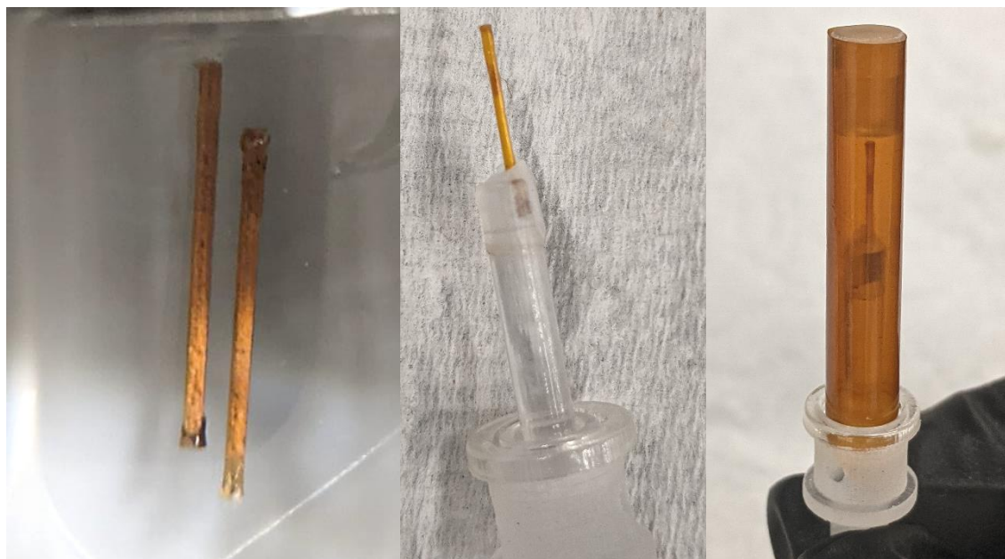
Figure 3: Images of a) \text{UO}_3 packed in 0.5 mm diameter Kapton tubing, b) packed tubing mounted on a sample holder, and c) mounted sample with an additional layer of Kapton as secondary containment.
