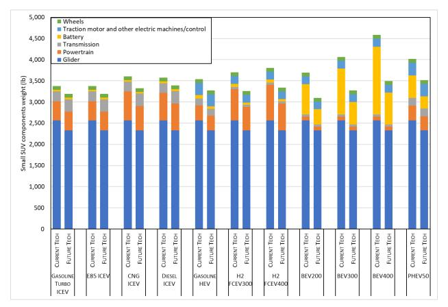
Figure 10. Small SUV component weight results (lb)
