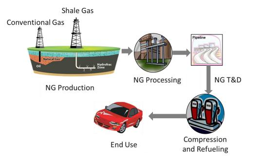
Figure 3. Key stages and activities of the CNG pathway (figure originally appeared in Elgowainy, et al. 2016)
