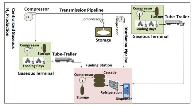
Figure 6. Hydrogen production and delivery pathways
