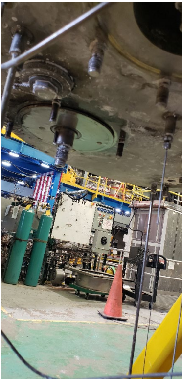
Figure 30: Labyrinth seal with pump shaft protruding, left. Labyrinth bottom plate removed and sodium scraped from the bottom of the vessel, middle. Sodium being cleaned from the shaft to allow for top portion of labyrinth seal to be removed, right.
