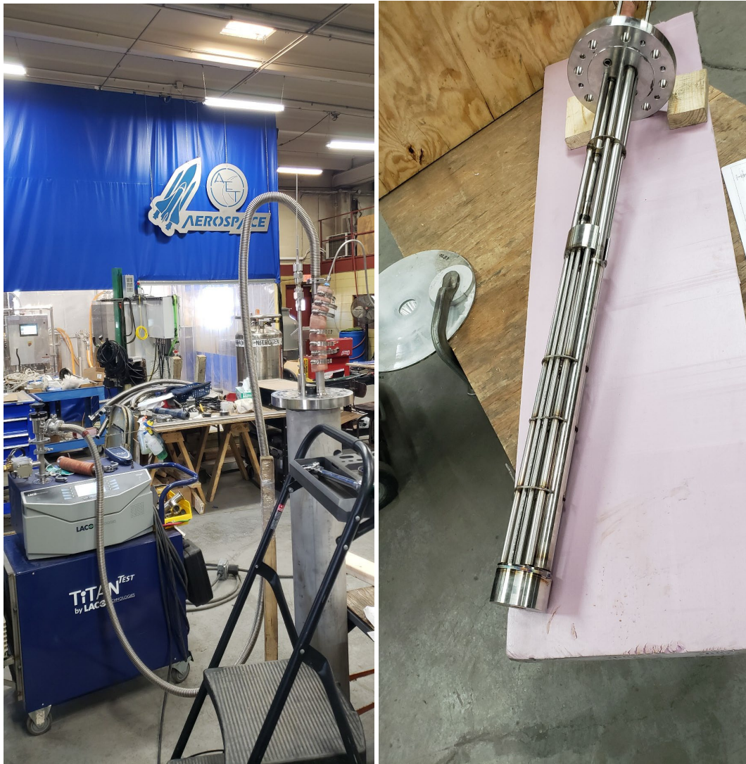
Figure 53: Photos at the IHX manufacturer before accepting the assembly. A helium leak check was performed under vacuum, as seen on left.
