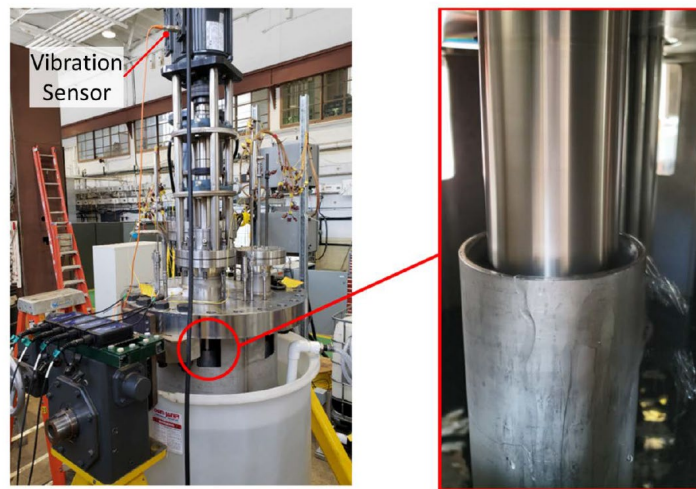
Figure 6: Photo showing water escaping the top of the column pipe
