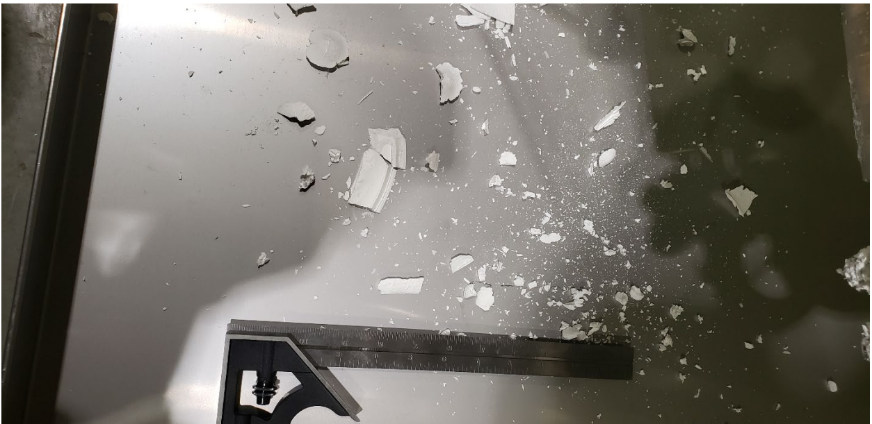
Figure 23: Photo showing sodium (bi) carbonate residue that was mechanically chipped off of the surfaces into a stainless-steel catch pan with ease. The bi(carbonate) was then processed in the METL burn stall with dry steam, wet steam, then water, all with no detectable chemical reaction.
