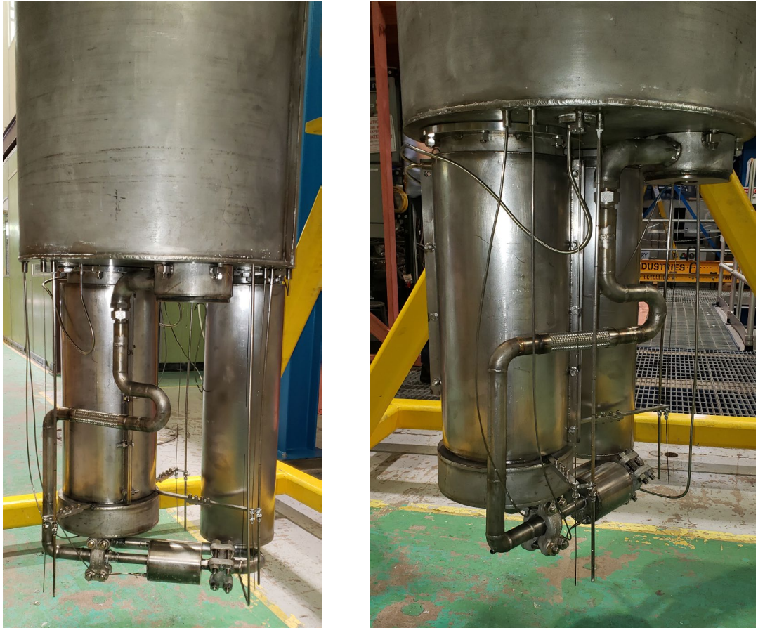
Figure 45: A photo showing the reassembled THETA cold pool components including the upgraded insulation and new thermal expansion piece that was replaced as a result of damage during carbonation volumetric expansion
