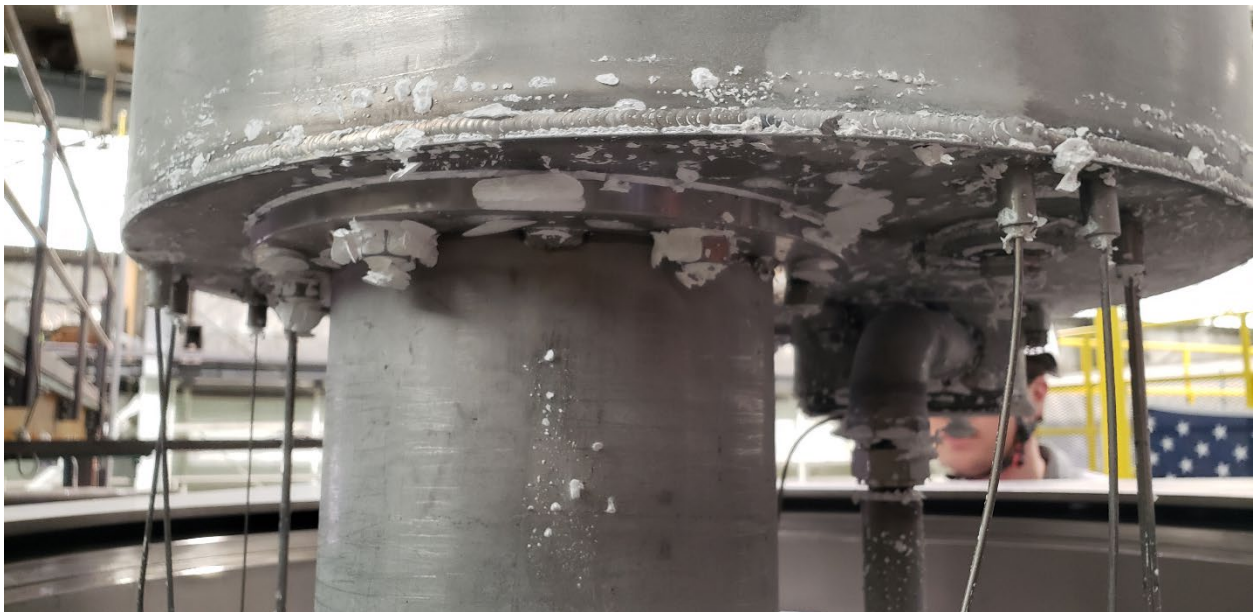
Figure 21: Photo of some of the sodium (bi)carbonate residue on the bottom of the hot pool inner vessel as THETA was being hoisted from the carbonation vessel.
