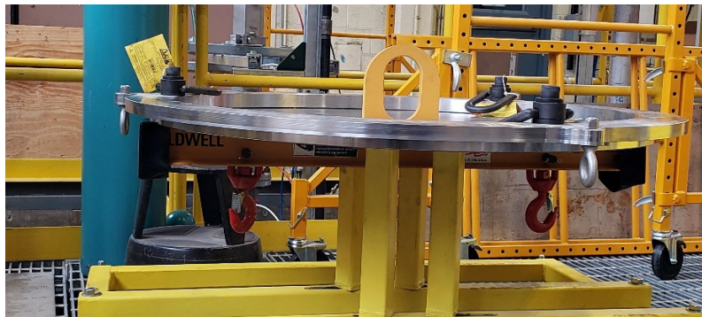
Figure 17: Custom top mounting plate was designed and installed into Flexicask assembly to accommodate a load spreader with the correct dimensions and weight rating for the THETA test article.
