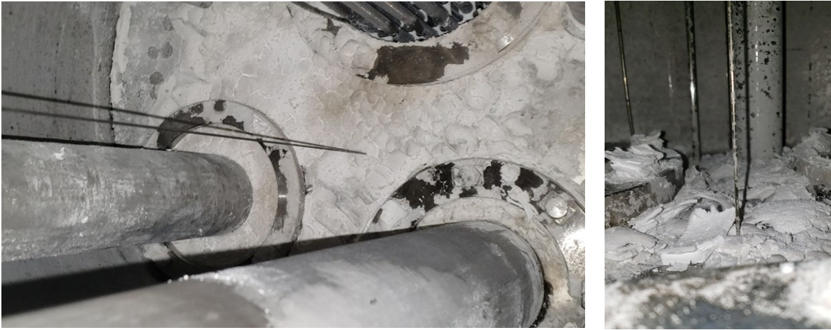
Figure 26: Photo showing a closer view of the carbonation byproduct in the inner vessel.
