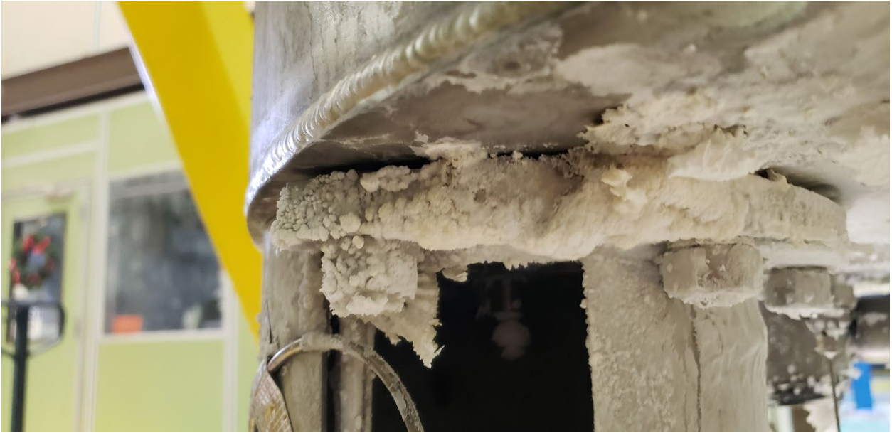
Figure 24: Photo showing some of the (bi)carbonate reaction product on the underside of the THETA inner vessel, near the outlet of the IHX. As can be seen, some crystallized formations seem to have developed during the carbonation reaction process.
