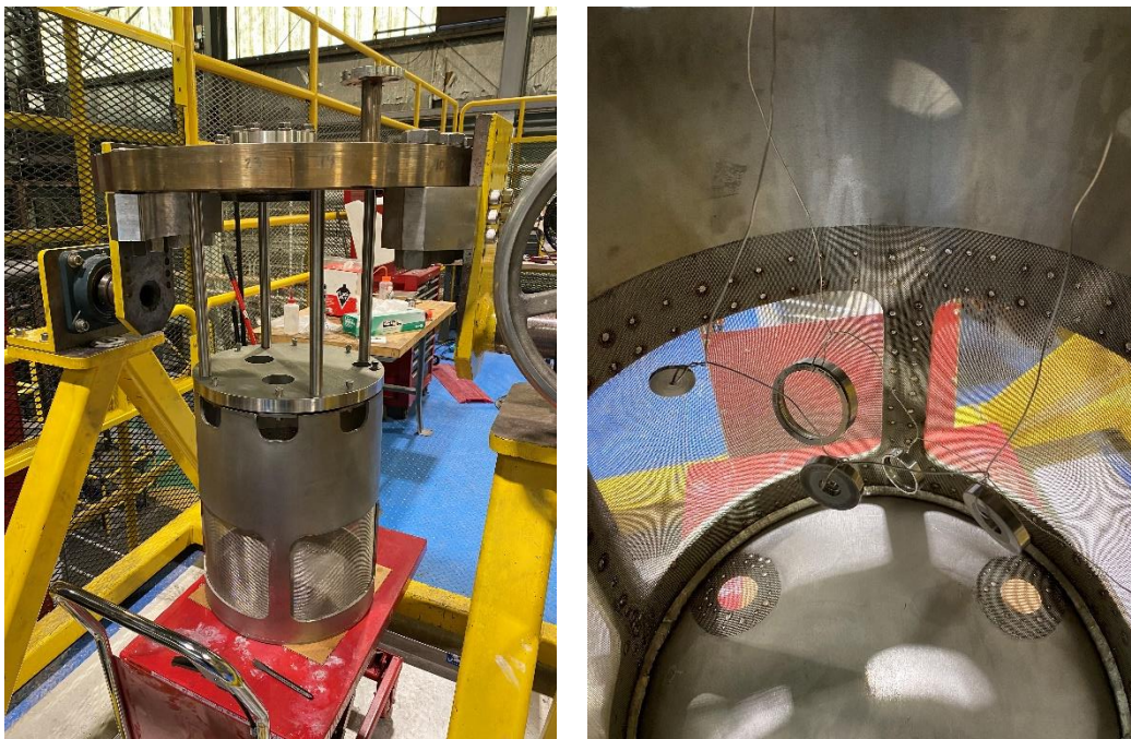
Figure 7 – Assembly of the STB liquid section on the assembly stand (left). Samples inside the STB secured with stainless steel wire (right).
