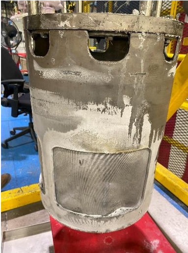
Figure 9 – The STB directly after removal from the carbonation process (left). Disassembly of the STB showing the samples hanging from the top plate after carbonation (right).
