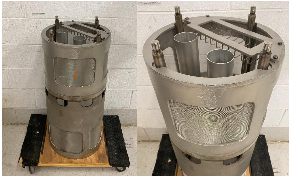
Figure 6 – Fabricated components of the STB (left). Close-up of the vapor testing section (right).
