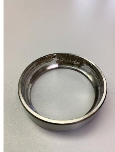
Figure 10 – Cleaned sample following sodium exposure and carbonation.
