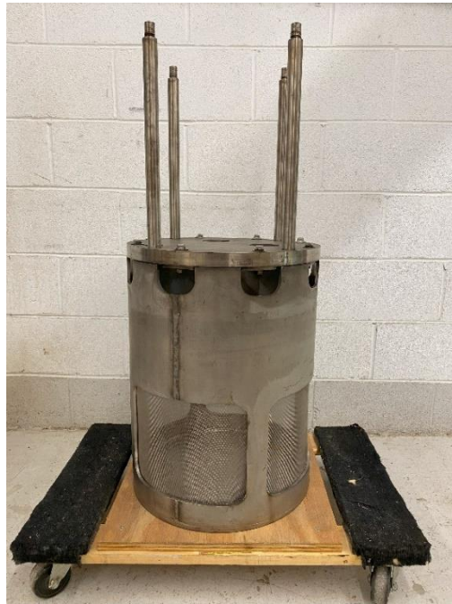
Figure 4 – Fabricated components of the STB liquid section.
