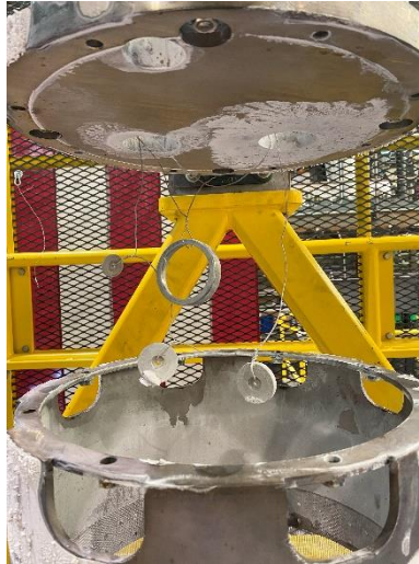
Figure 9 – The STB directly after removal from the carbonation process (left). Disassembly of the STB showing the samples hanging from the top plate after carbonation (right).
