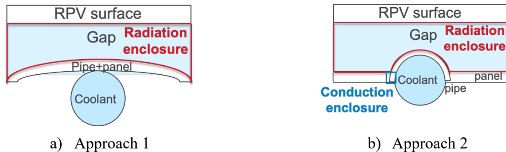
Figure 17 Schematics of RELAP5-3D modeling approaches of the water panel
