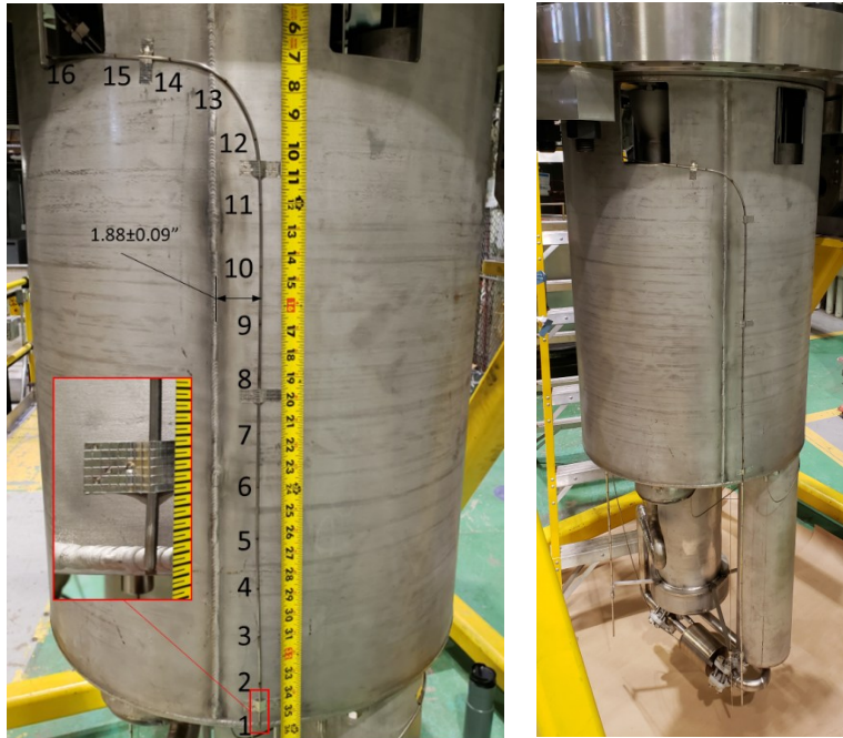
Figure 81: Photo showing location of thermocouples on hot pool vessel wall
