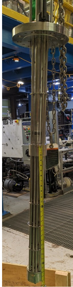
Figure 88: Intermediate heat exchanger (IHX)
